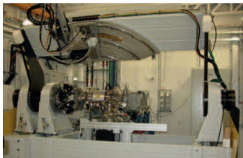
FIGURE 2.3: Photo of the UHV diffractometer on the SIXS beamline.
