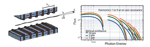
FIGURE 2.2: Schematic of an undulator (left); Intensity as a function of the chosen harmonics (right).
