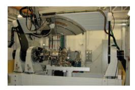
FIGURE 2.3: Photo of the UHV diffractometer on the SIXS beamline.
