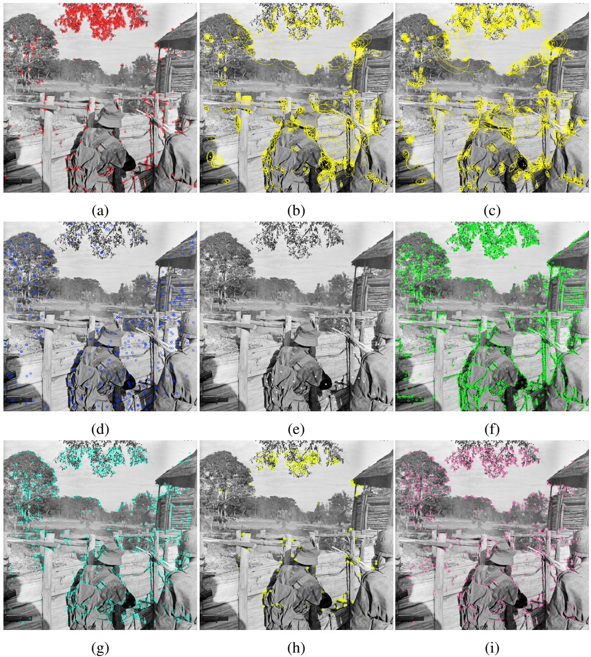
Figure 2.3: Interest points/regions detected by different detectors in an image from Musée Nicéphore Niépce collection: (a) Harris (b) Hesaff Affine (c) Harris Affine (d) MSER (e) Color symmetry (f) SIFT (g) CenSure (h) ORB (i) BRISK.
