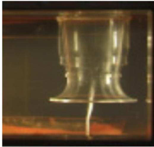
(a) Submerged vortex cavitation in the inlet part of a pump [67]
