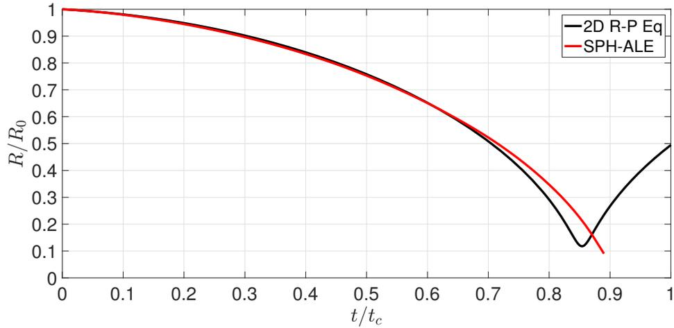
FIGURE 5.3: Comparison between numerical and analytic results of the Rayleigh collapse in free-field ( $p_w/p_b = 100$ ). (a) Non-dimensional radius vs. non-dimensional time.  $t_c$  is the analytic Rayleigh collapse time determined from the 2D Rayleigh-Plesset equation (Eq. 2.17)
