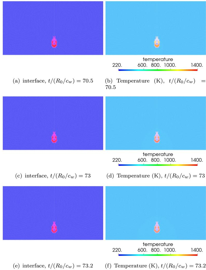
FIGURE 5.21: Evolution of collapse near a wall after the bubble collapse ( $p_w/p_b = 34$  and  $H_0/R_0 = 1.25$ ). At times: (a),(b) and (c)  $t/(R_0/c_w) = 70.5$ ; (d),(e) and (f)  $t/(R_0/c_w) = 73$ ; (g),(h) and (i)  $t/(R_0/c_w) = 73.2$ . Left: interface contour (red: gas, blue: liquid), right: temperature
