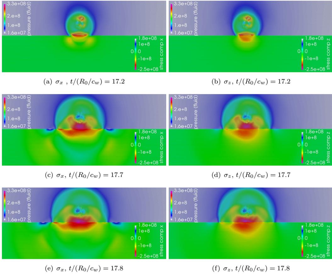
FIGURE 6.8: Evolution of pressure field  $[Pa]$  in the fluid and the stress components  $\sigma_x$  and  $\sigma_z$  in the solid domain due to the bubble collapse ( $p_w/p_b = 353$  and  $H_0/R_0 = 1.25$ ). Material: steel. (a, b) shows the instant of first impact on the wall ( $t/(R_0/c_w) = 17.2$ ); (c, d) shows the instant of second impact on the wall ( $t/(R_0/c_w) = 17.7$ ); (e, f) shows a moment after the second impact ( $t/(R_0/c_w) = 17.8$ ).
