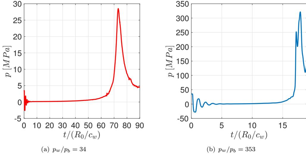
FIGURE 5.29: History of the wall pressure at the center of the wall for  $H_0/R_0 = 1.25$ .
