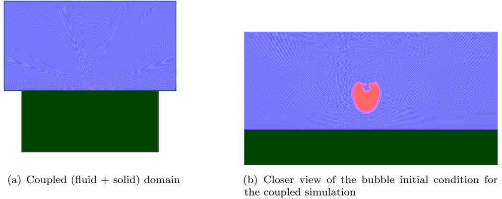
FIGURE 6.4: Coupled (fluid + solid) domain. Initial conditions for the fluid SPH domain, the solid SPH wall and the solid FEM wall in green. Case  $H_0/R_0 = 1.25$   $p_w/p_b = 353$ .
