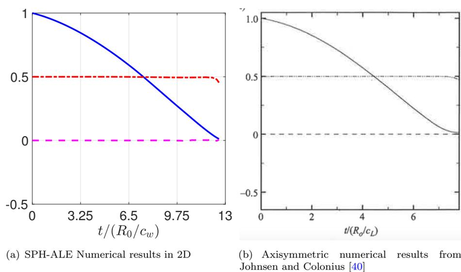
FIGURE 5.11: Rayleigh collapse in free-field ( $p_w/p_b = 353$ ). (a) SPH-ALE Numerical results in 2D, history of the normalized volume  $V/V_0$  (blue solid line), circularity (red dashed-dotted line) and displacement  $(X_C - X_0)/R_0$  (magenta dashed line). (b) Axisymmetric numerical results from [40], history of the normalized volume  $V/V_0$  (solid line), circularity (dashed-dotted line) and displacement  $(X_C - X_0)/R_0$  (dashed line)
