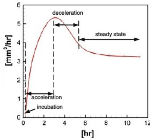
FIGURE 2.9: Rate of volume loss versus time curve [45].
