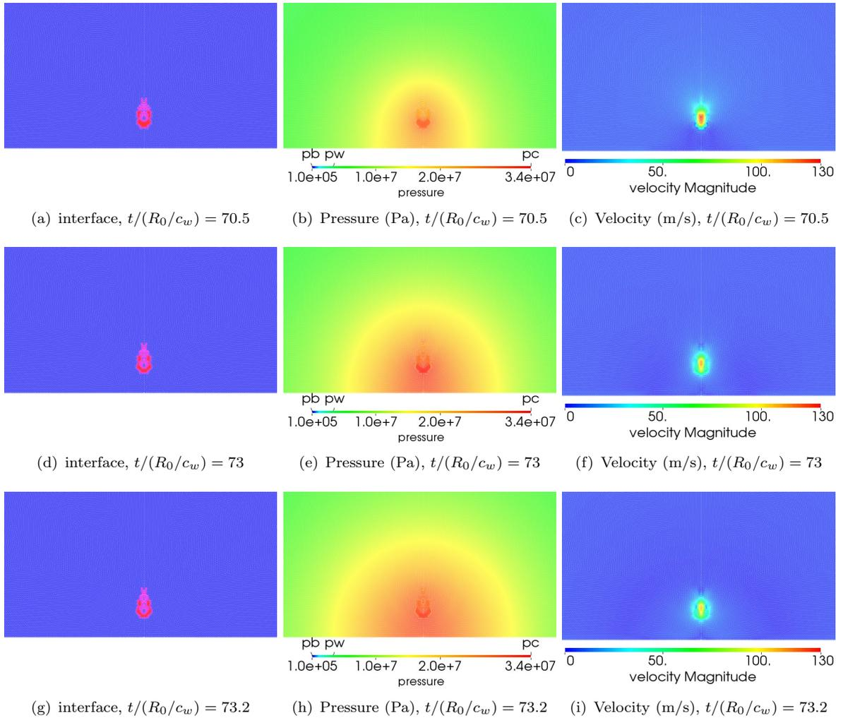
FIGURE 5.20: Evolution of collapse near a wall after the bubble collapse ( $p_w/p_b = 34$  and  $H_0/R_0 = 1.25$ ). At times: (a),(b) and (c)  $t/(R_0/c_w) = 70.5$ ; (d),(e) and (f)  $t/(R_0/c_w) = 73$ ; (g),(h) and (i)  $t/(R_0/c_w) = 73.2$ . Left: interface contours (red: gas, blue: liquid), center: pressure, right: velocity
