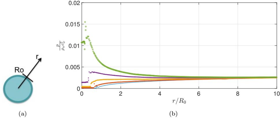
FIGURE 5.7: Pressure profile along a radial coordinate at different times, for free field collapse ( $p_w/p_b = 100$ ). At times: blue  $t/(R_0/c_w) = 15$ ; red  $t/(R_0/c_w) = 18.75$ ; yellow  $t/(R_0/c_w) = 22.5$ ; violet  $t/(R_0/c_w) = 24.75$ ; green  $t/(R_0/c_w) = 26.25$ . (a) scheme and representation of the radial coordinate; (b) pressure as a function of radial coordinate
