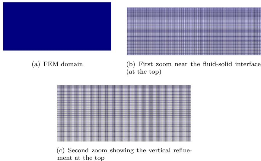
FIGURE 6.3: Mesh for the solid domain. Quadrangular elements. Whole and zoomed mesh representations near the fluid-solid interface
