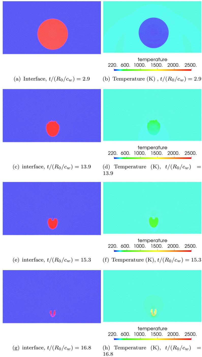
FIGURE 5.15: Evolution of collapse near a wall ( $p_w/p_b = 353$  and  $H_0/R_0 = 1.25$ ). At times: (a),(b) and (c)  $t/(R_0/c_w) = 2.9$ ; (d),(e) and (f)  $t/(R_0/c_w) = 13.9$ ; (g),(h) and (i)  $t/(R_0/c_w) = 15.3$  (j),(k) and (l)  $t/(R_0/c_w) = 16.8$ . Left: interface contour (red: gas, blue: liquid), right: temperature
