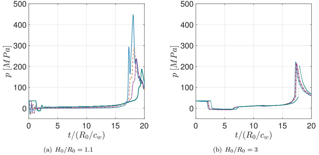
FIGURE 5.26: History of the wall pressure at different locations along the wall for  $p_w/p_b = 353$ . (a)  $H_0/R_0 = 1.1$  and (b)  $H_0/R_0 = 3$ . Blue ( $x/R_0 = 0$ ), red ( $x/R_0 = 0.5$ ), violet ( $x/R_0 = 1$ ) and green ( $x/R_0 = 2$ )
