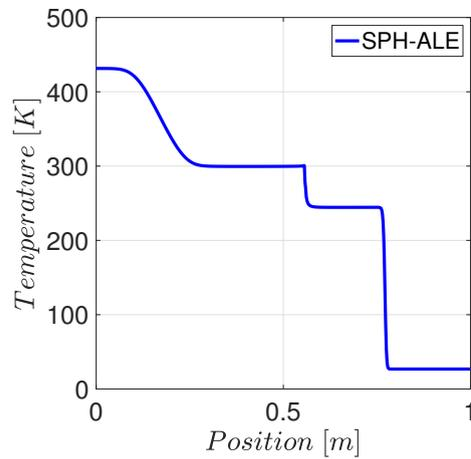
FIGURE 4.7: Shock tube test case. SPH numerical results of temperature at  $t = 7 \cdot 10^{-5} s$ .
