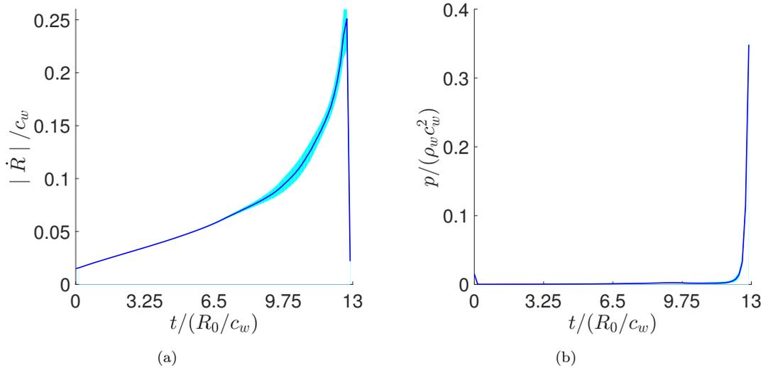
FIGURE 5.9: Rayleigh collapse in free-field ( $p_w/p_b = 353$ ). History of the velocity and pressure at the interface. (a) velocity at the interface, (b) pressure at the interface. The standard deviation is shown by the shaded area
