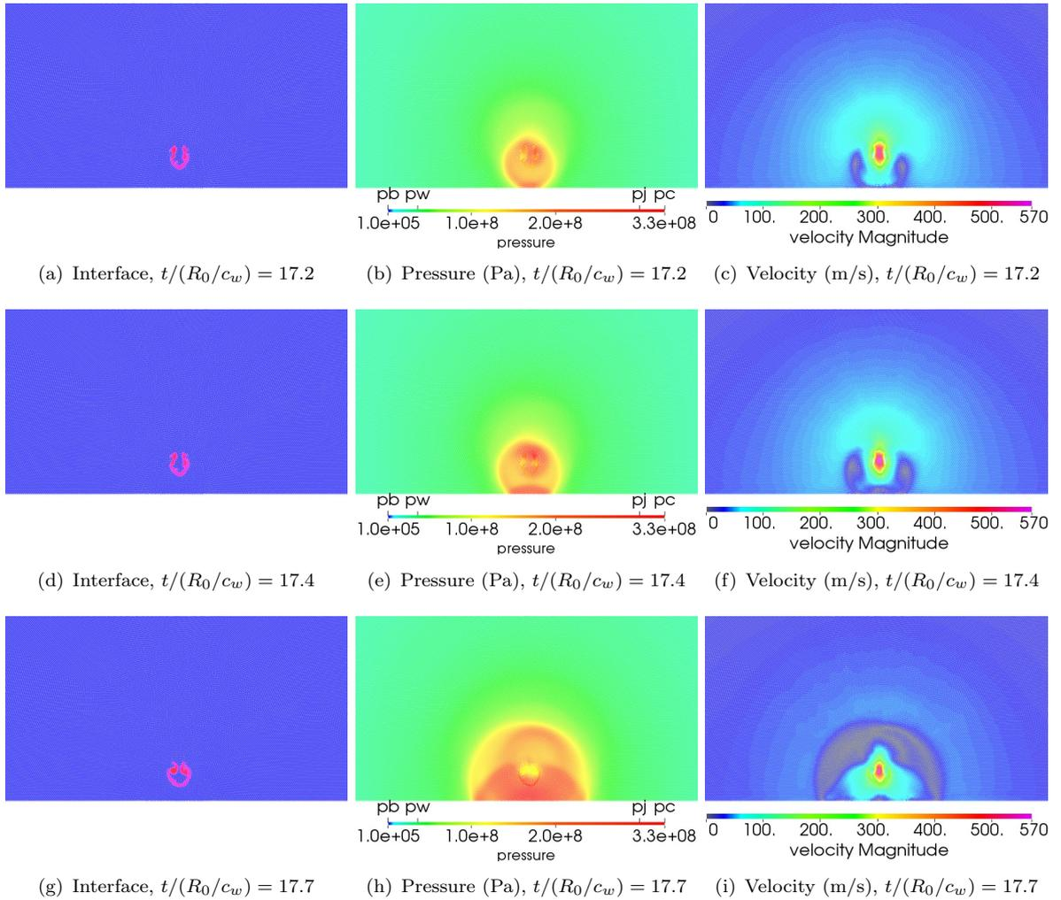
FIGURE 5.14: Evolution of collapse near a wall after the bubble collapse ( $p_w/p_b = 353$  and  $H_0/R_0 = 1.25$ ). At times: (a),(b) and (c)  $t/(R_0/c_w) = 17.2$ ; (d),(e) and (f)  $t/(R_0/c_w) = 17.4$ ; (g),(h) and (i)  $t/(R_0/c_w) = 17.7$ . Left: interface contour (red: gas, blue: liquid), center: pressure, right: velocity
