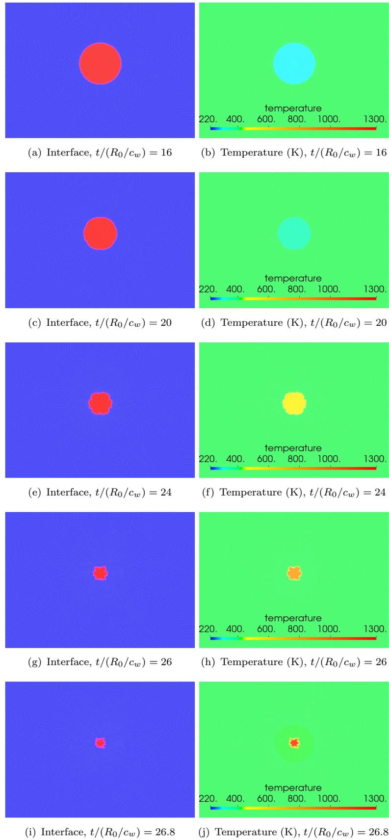
FIGURE 5.5: Evolution of free field collapse ( $p_w/p_b = 100$ ). At times: (a),(b) and (c)  $t/(R_0/c_w) = 16$ ; (d),(e) and (f)  $t/(R_0/c_w) = 20$ ; (g),(h) and (i)  $t/(R_0/c_w) = 24$ ; (j), (k) and (l)  $t/(R_0/c_w) = 26$ ; (m), (n) and (o)  $t/(R_0/c_w) = 26.8$ . Left: interface contour (red: gas, blue: liquid), right: temperature
