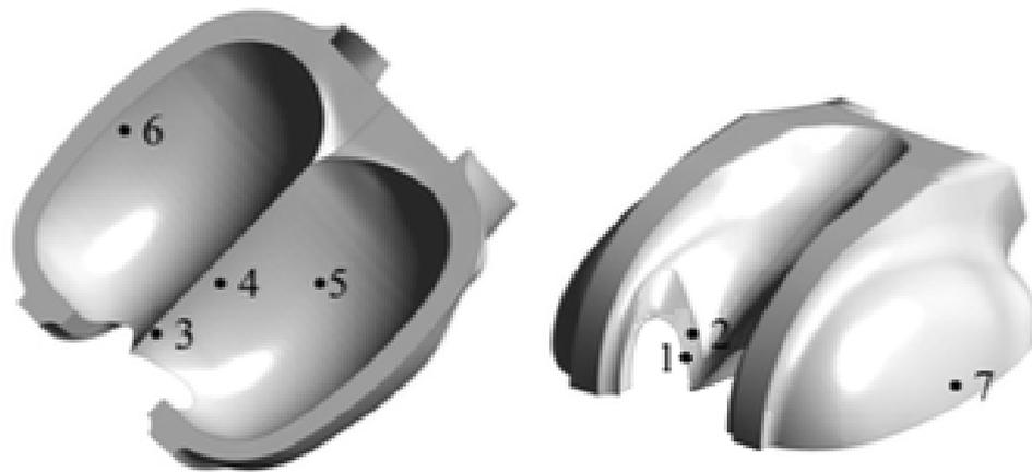
FIGURE 2.12: Location of hydraulic damage on a Pelton bucket [86]
