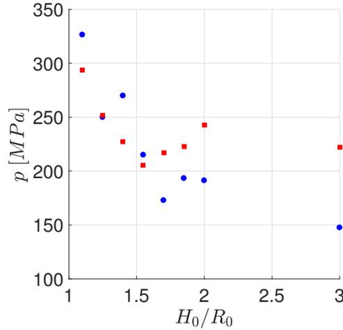
FIGURE 5.27: Pressure as a function of the standoff distance  $H_0/R_0$  for  $p_w/p_b = 353$ . Blue circle: water hammer pressure calculated by Eq. 5.2, red square: First pressure peak on the wall measured in the simulations
