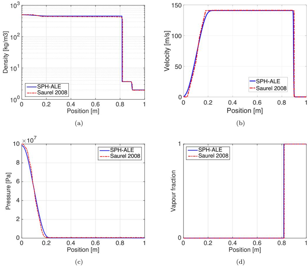
FIGURE 4.8: Multiphase shock tube test case. Numerical results in spatial distribution at  $t = 473 \mu s$ . Comparison between SPH-ALE results (solid line) and results from Saurel in [91] (dashed lines)
