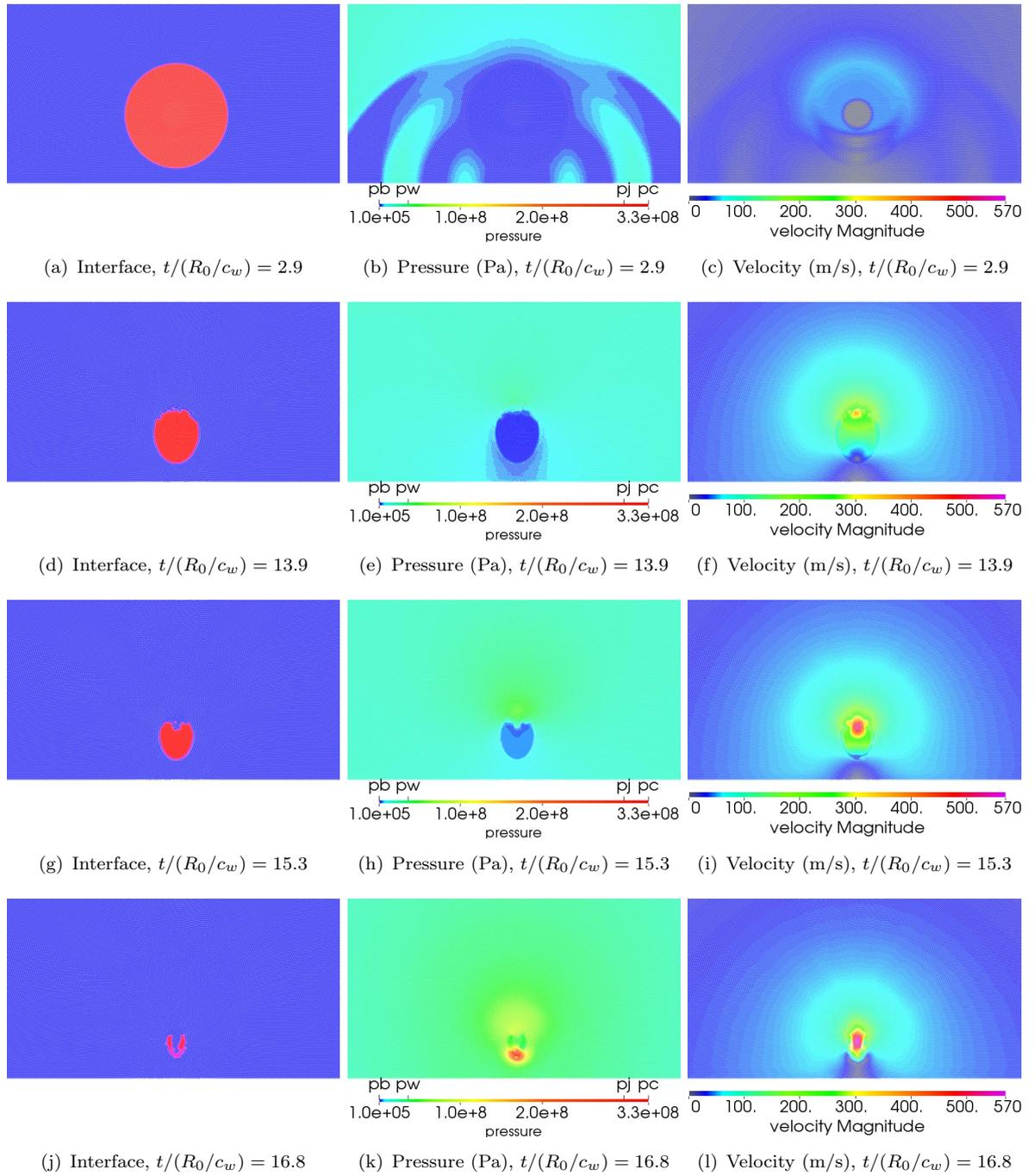
FIGURE 5.13: Evolution of collapse near a wall ( $p_w/p_b = 353$  and  $H_0/R_0 = 1.25$ ). At times: (a),(b) and (c)  $t/(R_0/c_w) = 2.9$ ; (d),(e) and (f)  $t/(R_0/c_w) = 13.9$ ; (g),(h) and (i)  $t/(R_0/c_w) = 15.3$  (j),(k) and (l)  $t/(R_0/c_w) = 16.8$ . Left: interface contour (red: gas, blue: liquid), center: pressure, right: velocity
