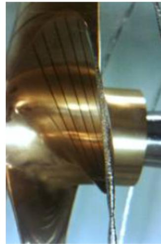
(b) Cavitating tip vortices on a propeller in open water [104]
