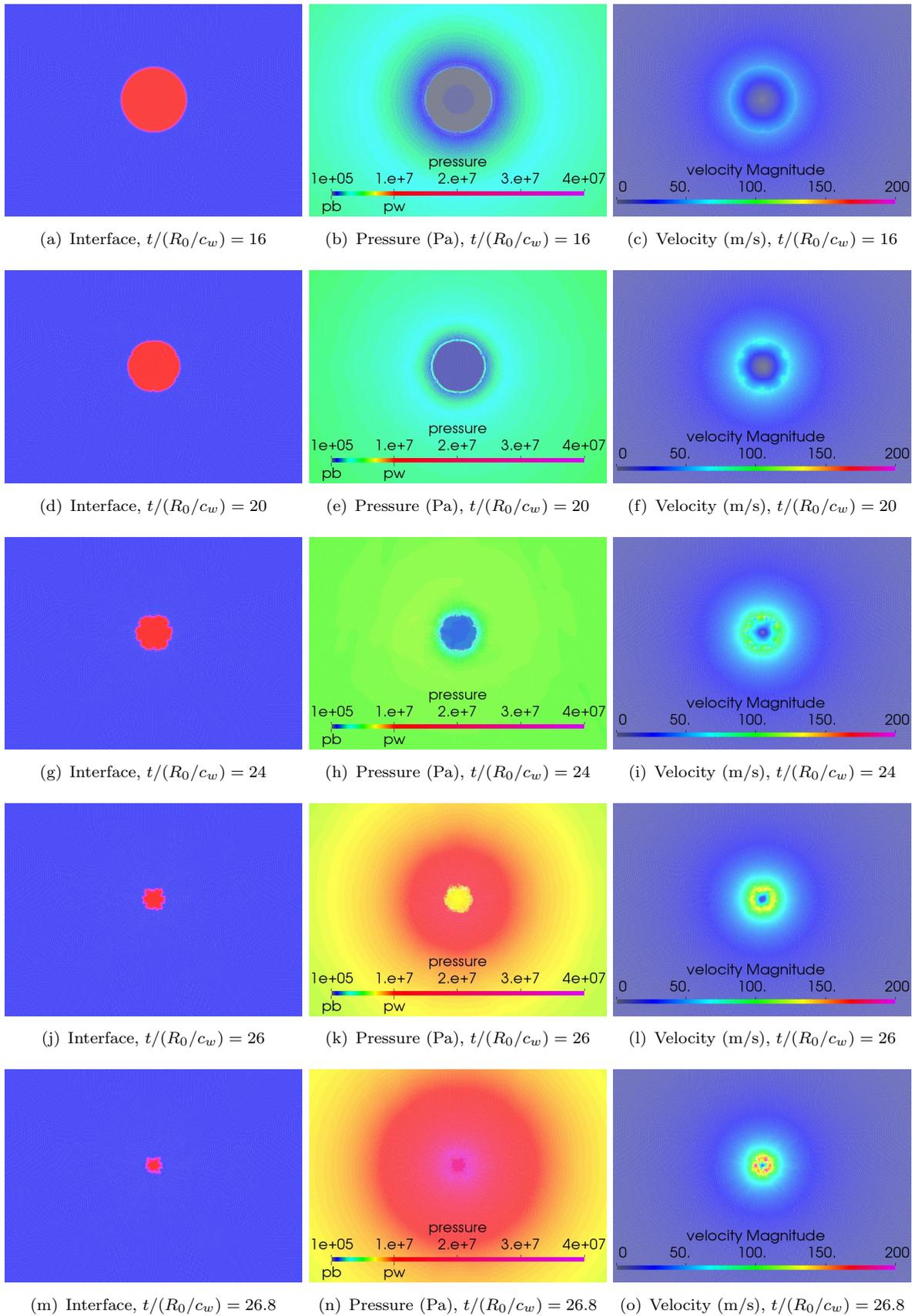
FIGURE 5.4: Evolution of free field collapse ( $p_w/p_b = 100$ ). At times: (a),(b) and (c)  $t/(R_0/c_w) = 16$ ; (d),(e) and (f)  $t/(R_0/c_w) = 20$ ; (g),(h) and (i)  $t/(R_0/c_w) = 24$ ; (j), (k) and (l)  $t/(R_0/c_w) = 26$ ; (m), (n) and (o)  $t/(R_0/c_w) = 26.8$ . Left: interface contour (red: gas, blue: liquid), center: pressure, right: velocity
