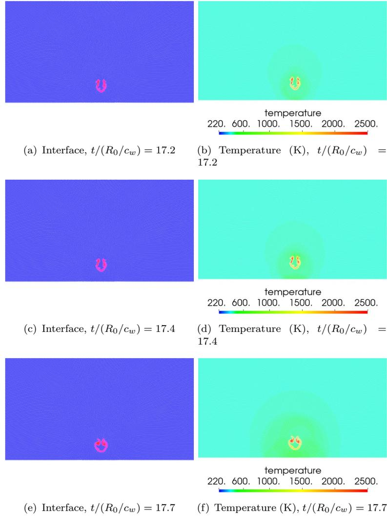
FIGURE 5.16: Evolution of collapse near a wall after the bubble collapse ( $p_w/p_b = 353$  and  $H_0/R_0 = 1.25$ ). At times: (a),(b) and (c)  $t/(R_0/c_w) = 17.2$ ; (d),(e) and (f)  $t/(R_0/c_w) = 17.4$ ; (g),(h) and (i)  $t/(R_0/c_w) = 17.7$ . Left: interface contour (red: gas, blue: liquid), right: temperature
