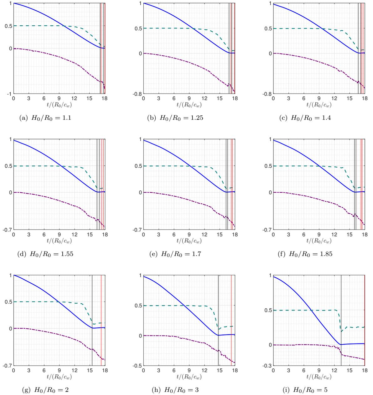
FIGURE 5.17: History of the normalized volume  $V/V_0$  (blue solid line), circularity (green dashed line) and displacement  $(X_C - X_0)/R_0$  (violet dashed-dotted line) of collapse near a wall for  $p_w/p_b = 353$ . Jet impact time (first black vertical line), bubble collapse time (second black vertical line), pressure peaks on the wall (two red vertical lines)
