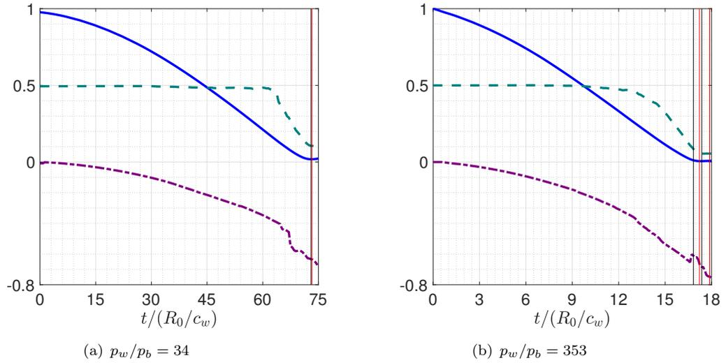
FIGURE 5.19: History of the normalized volume  $V/V_0$  (blue solid line), circularity (green dashed line) and displacement  $(X_C - X_0)/R_0$  (violet dashed-dotted line) of collapse near a wall ( $H_0/R_0 = 1.25$ ). (a)  $p_w/p_b = 34$ , (b)  $p_w/p_b = 353$
