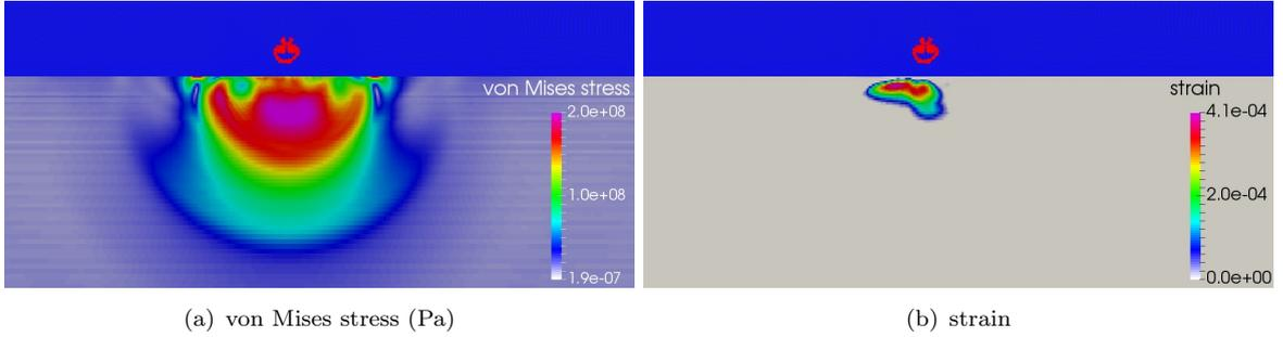
FIGURE 6.12: Material response at  $t/(R_0/c_w) = 17.8$ , moment of highest stress due to the bubble collapse for  $p_w/p_b = 353$  and  $H_0/R_0 = 1.25$ . Material: steel.
