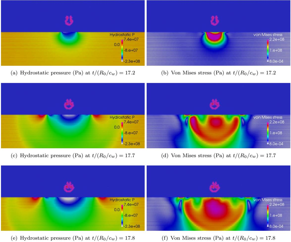
FIGURE 6.9: Evolution of the material response due to the bubble collapse ( $p_w/p_b = 353$ ,  $H_0/R_0 = 1.25$ ). Material: stainless steel. (a) and (b) show the moment of the first wave impact on the wall (at  $t/(R_0/c_w) = 17.2$ ); (c) and (d) show the moment of the second wave impact on the wall (at  $t/(R_0/c_w) = 17.7$ ); (e) and (f) show a moment after the second impact ( $t/(R_0/c_w) = 17.8$ ).
