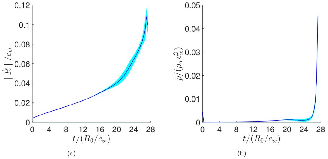
FIGURE 5.8: Rayleigh collapse in free-field ( $p_w/p_b = 100$ ). History of the velocity and pressure at the interface. (a) velocity at the interface, (b) pressure at the interface. The standard deviation is shown by the shaded area
