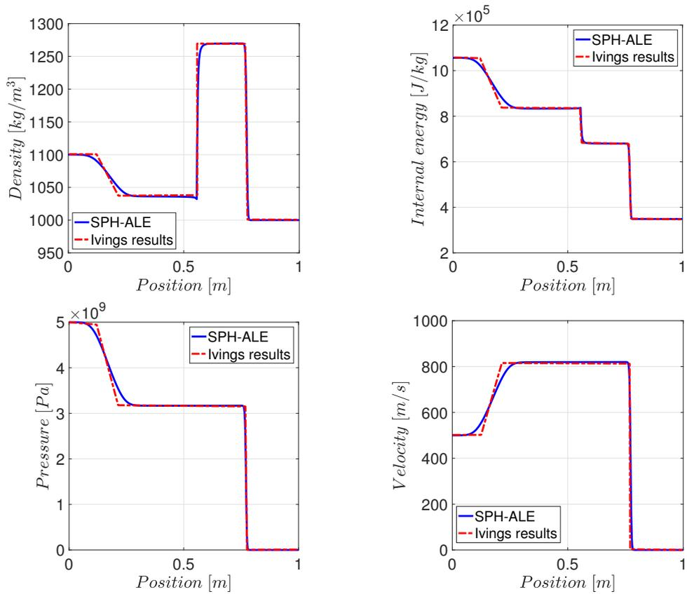
FIGURE 4.6: Shock tube test case. Flow fields in spatial distribution at  $t = 7 \cdot 10^{-5} s$ . Comparison between SPH-ALE numerical results (solid lines) and the exact solution from Ivings in [37] (dashed lines)
