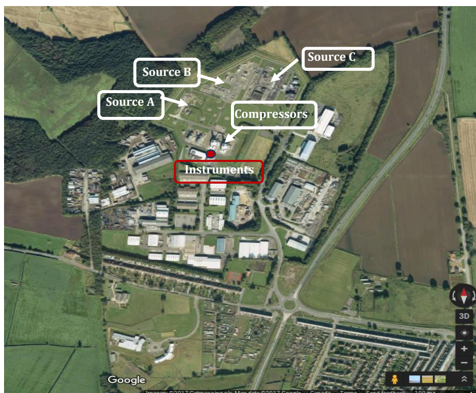
Figure 3.1 Aerial view of the natural gas compressor station and the location of the presumed principle natural gas sources from Ars et al. 2017 © Google Maps. Location of sampling inlet is indicated by circular red marker.
