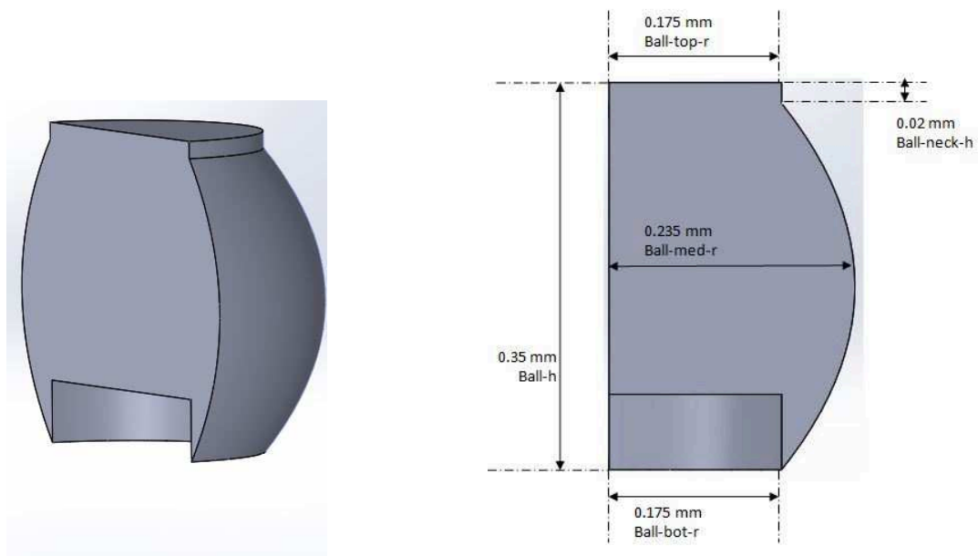
FIGURE 4.11: Dimensions du joint de brasure
