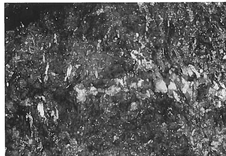
Fig. 58. Detail of siderite of La Chevrette, intricately intergrown fabric of fusiform crystals. La Chevrette, 2 x.
