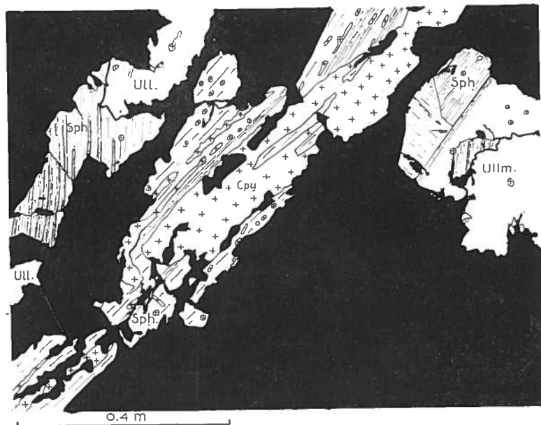
Fig. 64. Arbitrarily shaped ullmannite (Ullm) crystals are confined to the sulphide-streaks of the La Fayolle vein. Note intergrowths of sphalerite (Sph) and chalcopyrite (Cpy) and exsolution drops of chalcopyrite (crosses) in sphalerite.
