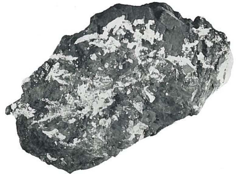
Fig. 68. Large euhedral crystals of siderite and ankerite (white) from the vug-like deposit of Le Vent, \frac{1}{2} x.
