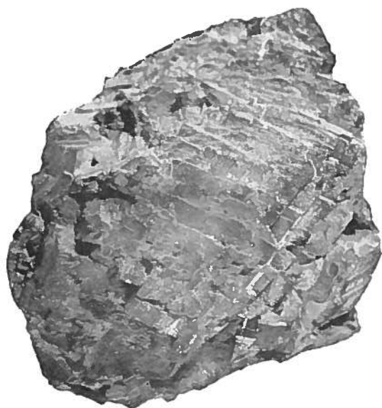
Fig. 59. Large rhombohedral crystals of siderite belonging to the younger mineralization. Le Merle, \frac{2}{3} x.
