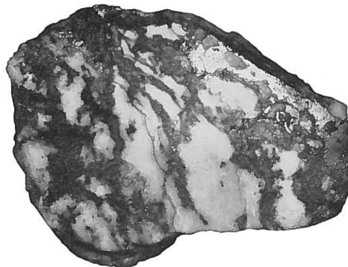
Fig. 88. Galena (high reflect.) and sphalerite (black) have been disrupted and dissected by quartz (white) into streaky fragments. Fosse Guerre, 1x.
