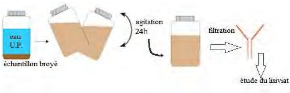
Figure B1- 11: illustration d'un essai de lixiviation
