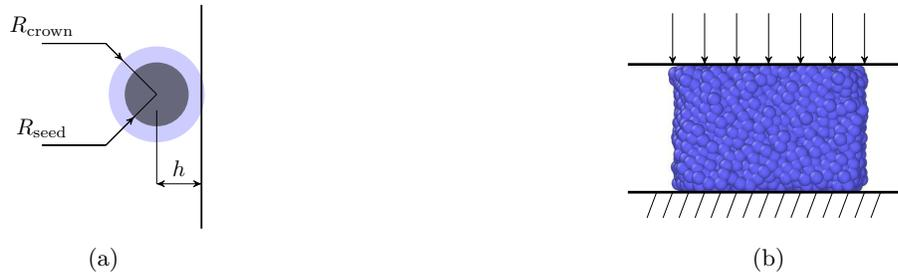
Figure 3: Boundary conditions. (a) Elementary mesh / particle interaction. Crown contact example. (b) Compression test: top and bottom meshes with prescribed motion; free lateral sides.
