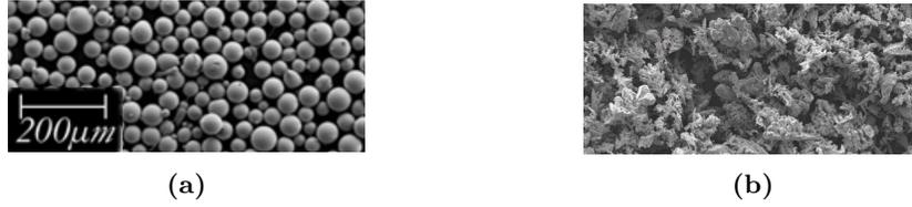
**Figure 2.13:** SEM views of the initial state of the powders at identical scales. (a) Atomized amorphous  $Zr_{57}Cu_{20}Al_{10}Ni_8Ti_5$ : spheroidal powder. SEM view from [73, p.41]. (b) Electrolytic crystalline copper: dendritic powder.
