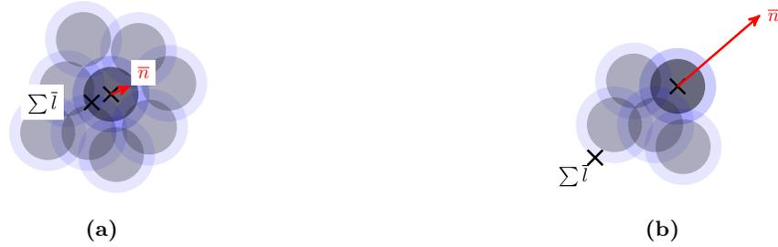
**Figure 9.8:** Computation of the outward vector  $\bar{n}$  of a particle, from the positions of its neighbors. (a) A particle surrounded by neighbors. The centroid of the neighbors is very close to the center of particle. The magnitude  $n$  is small and its orientation is meaningless. (b) A particle at a free surface. The magnitude  $n$  is large and  $\bar{n}$  points “outwards”.
