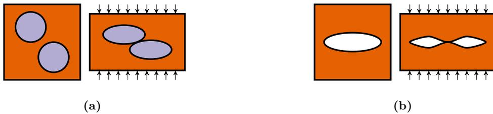
**Figure 3.9:** Contact/self-contact typology of discontinuity interactions. (a) Contact between two distinct inclusions in a matrix. (b) Self-contact of the boundary of a hole in a matrix.
