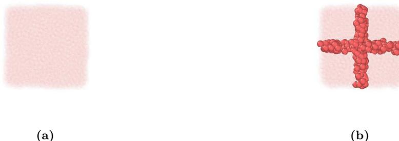
**Figure B.1:** Illustration of a MPI bug. Compression of a dense sample, using the self-contact detection. Top view, no transparency for the particles with a least one “interface” detected. (a) MPI grid  $1 \times 1 \times 1$ . Correct behavior: no interface detected. (b) MPI grid  $2 \times 2 \times 1$ . Erroneous behavior: interfaces detected at the boundaries of the processors. The self-contact variables are not correctly passed between processors.
