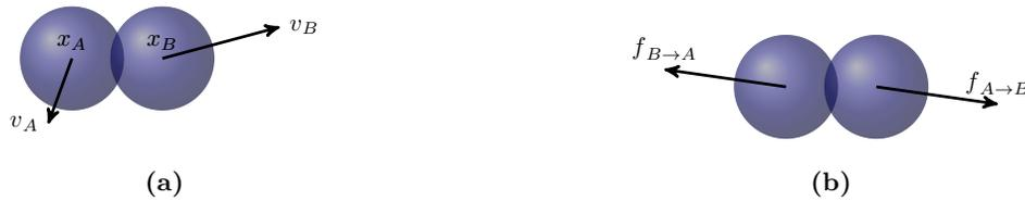
**Figure 8.3:** From kinematics to forces. (a) Position and velocity of a pair of interacting particles ( $A, B$ ). (b) Reciprocal forces:  $\bar{f}_{B \rightarrow A} = -\bar{f}_{A \rightarrow B}$ , typically computed from relative position and velocity of the particles.
