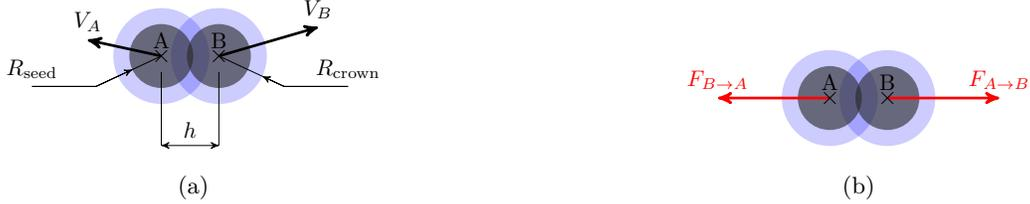
Figure 1: Pairwise interactions. (a) Geometry and kinematics of a pair: relative position and velocities. Seed contact example. (b) Interaction reciprocal forces:  $F_{A \to B} = -F_{B \to A}$ . Pairwise forces, computed from the kinematics of the pair (Equation 1).
