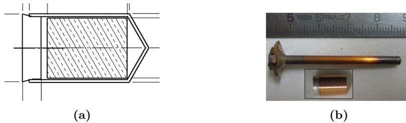
**Figure 2.16:** Encapsulated co-extrusion of compacted powders. (a) Schematic of the copper capsule containing the compacted powder (cross-hatched) during the extrusion. The capsule is closed by a steel lid. (b) Hot extruded and initial states. The composite is protected by the capsule and is not visible.
