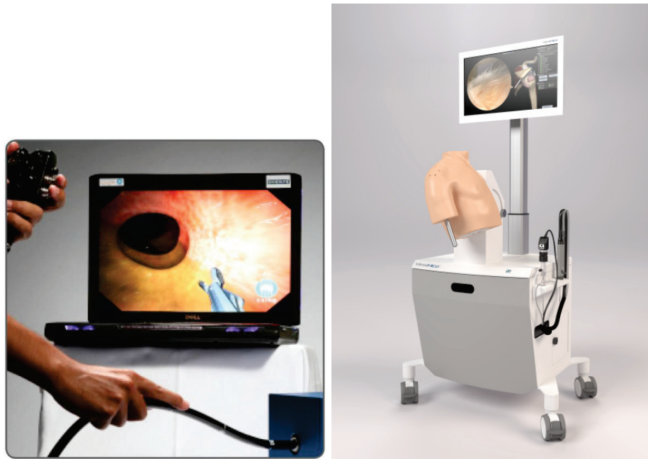
FIGURE 1.1: Left: EndoSim Flexible Endoscopic Simulator from Surgical Science, Inc. Model number ES01; right: VirtaMed ArthroS with shoulder model from VirtaMed AG.
