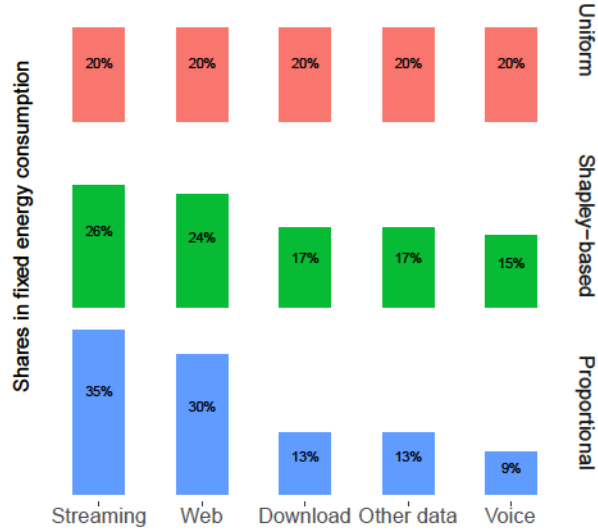
Figure 2.5: Shares in fixed energy consumption: uniform, proportional and Shapley-based sharing.
