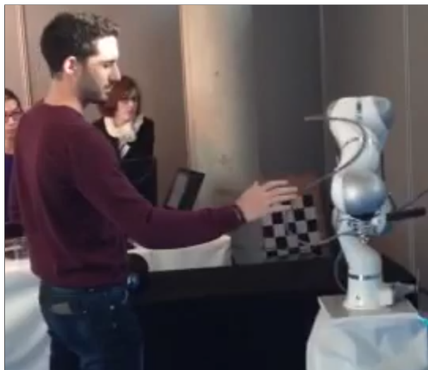
Figure 3.1: View of a user sharing the same workspace with a KUKA LWR4 robotic manipulator. The kinetic energy of the robot is modulated as function of the real-time distance between the human and the robot in order to best perform the task of the robot while ensuring safety.
