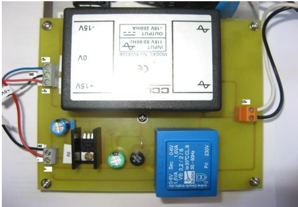
Figure 53: Analog power supply unit with 5V and +/-15v, powering the four quadrant detector unit, the conductivity measurement circuit and the pressure sensor card.
