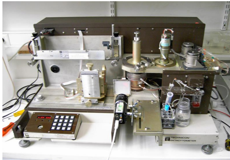
Figure 33: Modified Technicon Ektacytometer with a beam splitter and a camera
