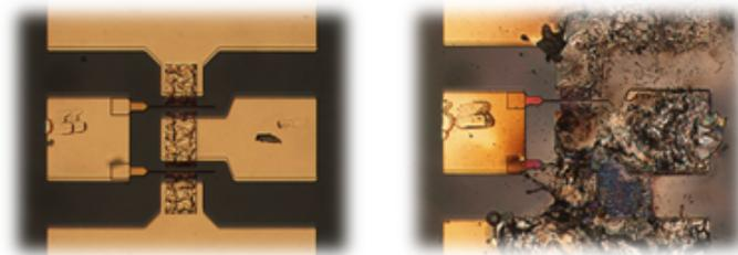
Figure 3.4: Optical image of a device before stress and after a catastrophic degradation
