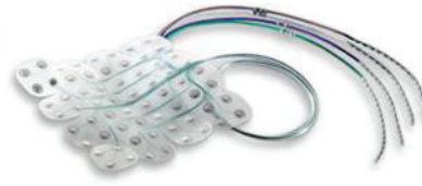
Figure 1.8: Commercialized ECoG array [Blackrock, 2017].
