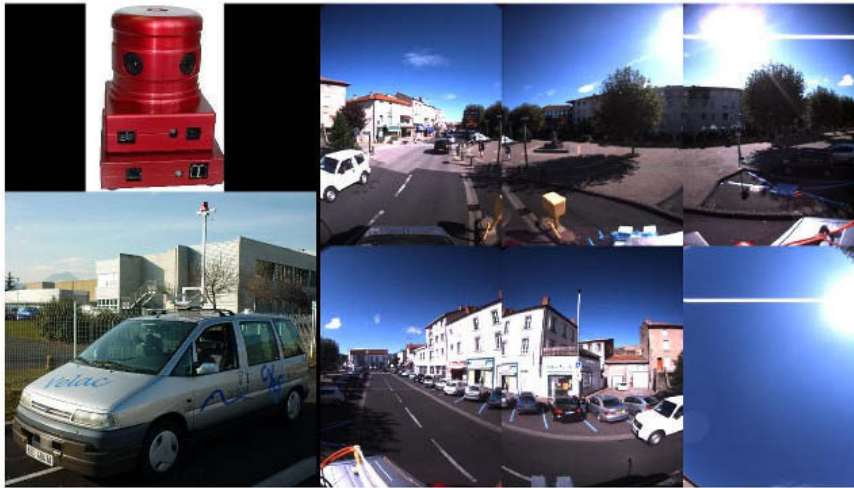
FIGURE 3.14: Camera (PointGrey Ladybug 2) and images for CC. The cameras are global shutter. The camera pointing toward the sky is not used in our experiments.
