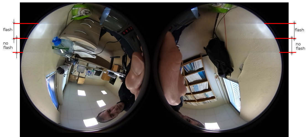
FIGURE G.3: Ricoh Theta S camera observing a room periodically flashed by a stroboscope. The flash/no flash can be seen on the wall at the top of the circular images (best viewed in the electronic version).
