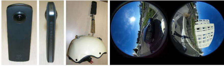
FIGURE 3.13: Spherical camera (Ricoh Theta S) and images for WU. Both rolling shutter and image motion go from bottom to top.
