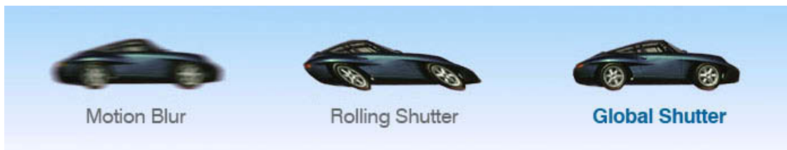
FIGURE 3.9: Motion blur, RS and GS. Source: www.teledynedalsa.com .
