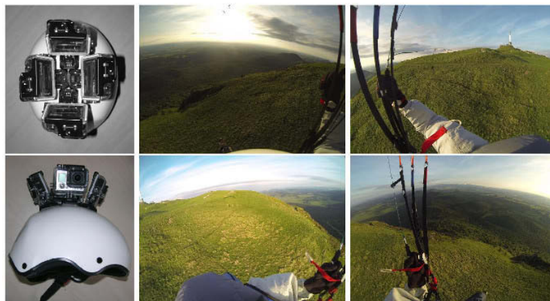
FIGURE 3.12: Cameras (four Gopro Hero 3 in their housings) and images for FH. The rolling shutter always goes from top to bottom, the image motion goes forward/toward right/backward/toward left.
