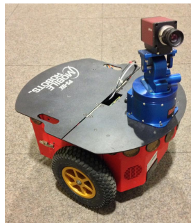
Figure 3.32: Pioneer robot used in the navigation experiment
