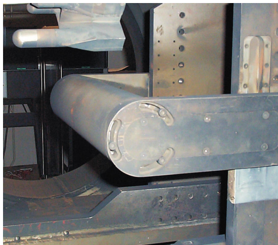
Figure 1.11: Image of the cylindrical experimental model in the HEG facility (taken from [Karl et al. , 2003]).
