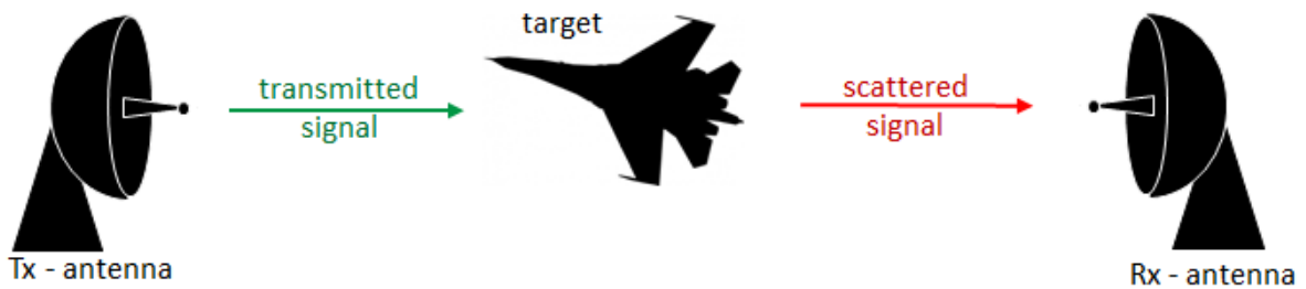
Figure 1.4 Forward scatter radar
