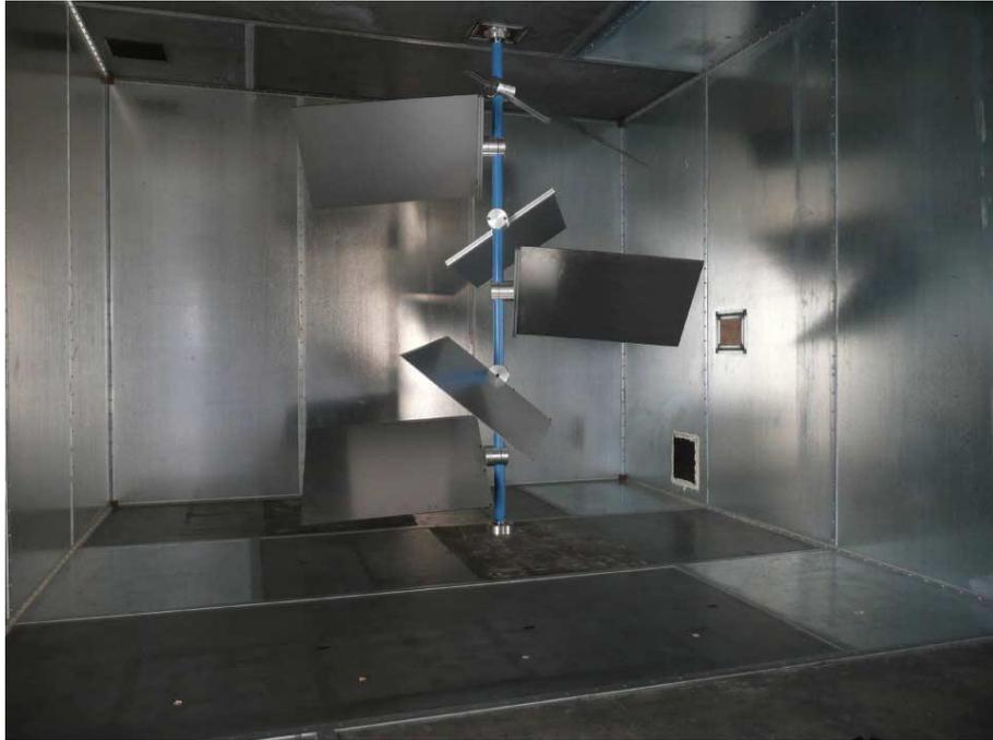
Figure 2.18 Reverberation chamber at IETR research laboratory
