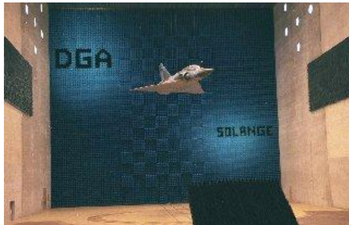
Figure 1.18 SOLANGE indoor RCS range [19]
