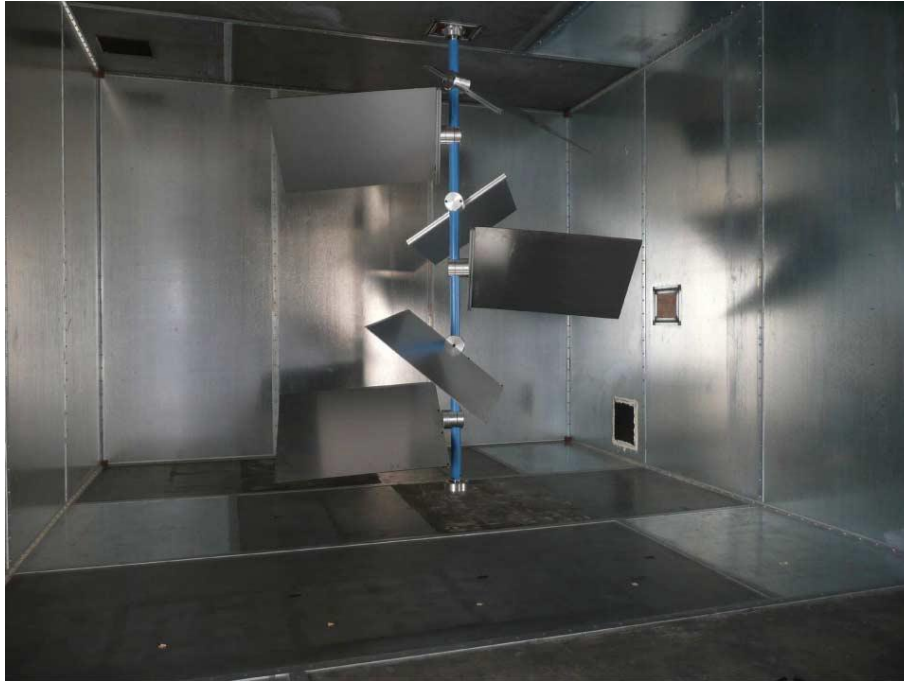
Figure 2.18 Reverberation chamber at IETR research laboratory
