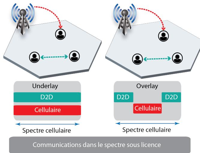
Figure 2.6 – Communications D2D : *underlay* vs *overlay*.
