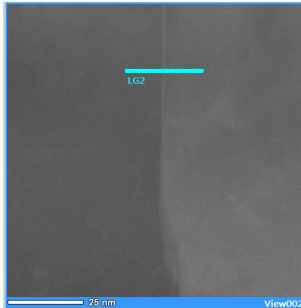
**Fig. 2.26.** STEM bright-field image of the series of EDX points across the GB in a thin foil from the Fe-0.034at%P-0.01at.%C alloy (irradiated to 0.75 dpa)
