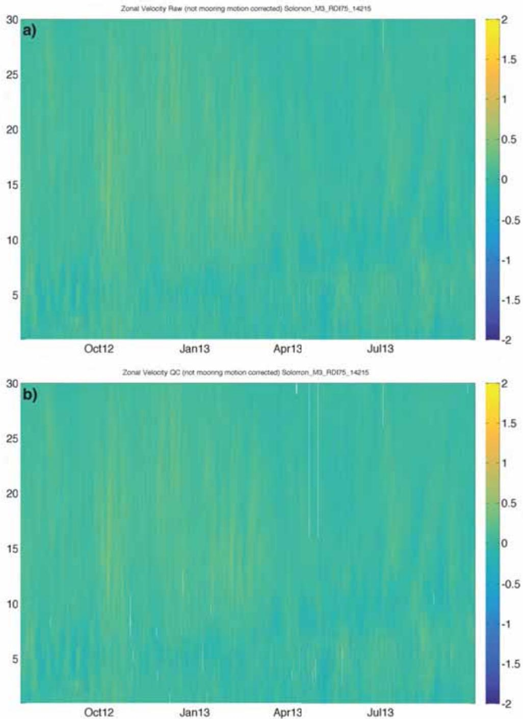
Figure 15 – Comparisons of zonal velocity ( $m.s^{-1}$ ) in Solomon Strait M3, (a) raw zonal velocity and (b) QC zonal velocity of the RDI 75 kHz ADCP.
