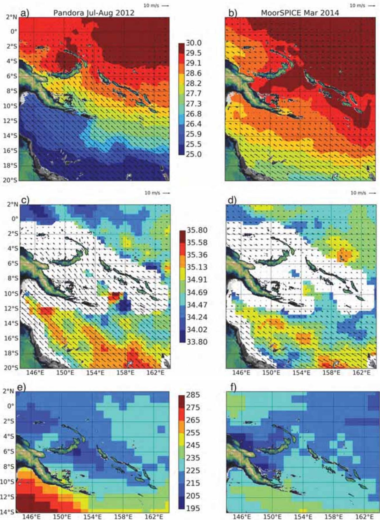
**Figure 3.2** – (top panels) SST ( $^{\circ}C$ ) from OSTIA during (a) Pandora and (b) MoorSPICE cruises. (middle panels) SSS (pss-78) from the “L4aSSS In situ Match-up products” during (c) Pandora and (d) MoorSPICE cruises. Satellite wind vectors averaged during each cruise from ASCAT are overlaid. Note the unit vector in the upper right of the top panels. (bottom panels) daily gridded OLR ( $W.m^{-2}$ ) averaged during (e) Pandora and (f) MoorSPICE cruises.
