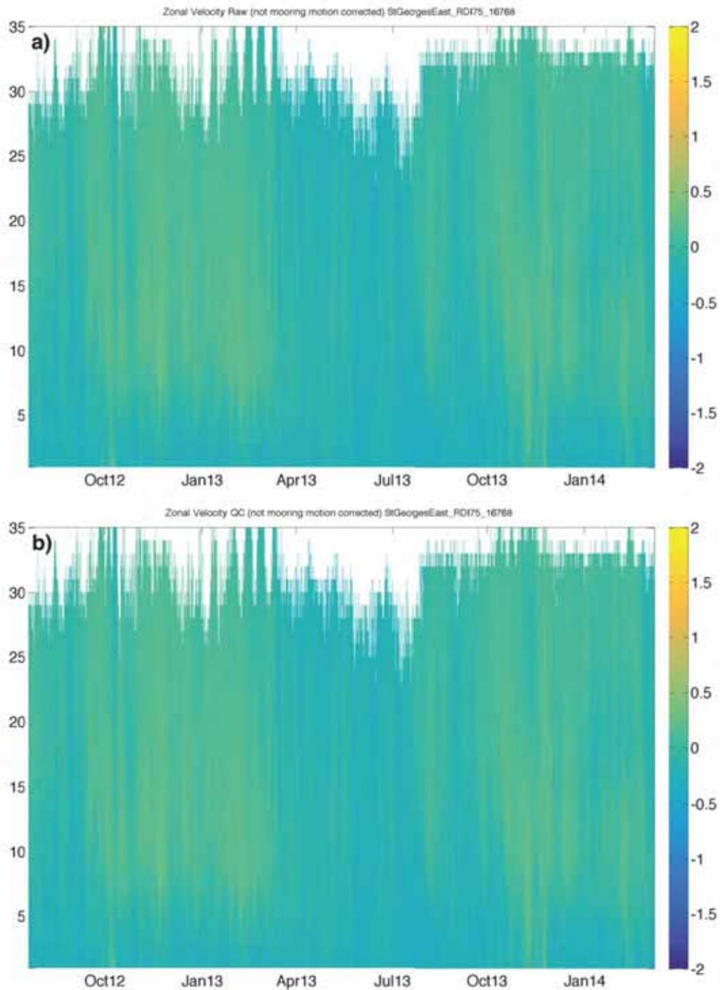
Figure 21 – Comparisons of zonal velocity ( $m.s^{-1}$ ) in St Georges Channel East, (a) raw zonal velocity and (b) QC zonal velocity of the RDI 75 kHz ADCP.
