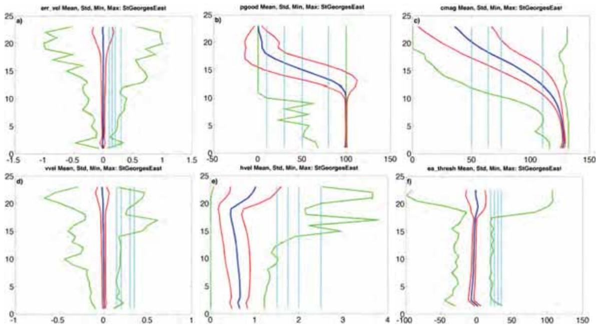
Figure 17 – Mean (thick blue line), standard deviation (red lines) and minimum and maximum (green lines) of the (a) error velocity ( $m.s^{-1}$ ); (b) percent good; (c) correlation magnitude; (d) vertical velocity ( $m.s^{-1}$ ); (e) horizontal velocity ( $m.s^{-1}$ ) and (f) echo amplitude (counts) for the Solomon Strait M3 RDI 75 kHz ADCP versus bin. The four threshold values used in each QC test are marked by cyan lines in panels (a) to (f).
