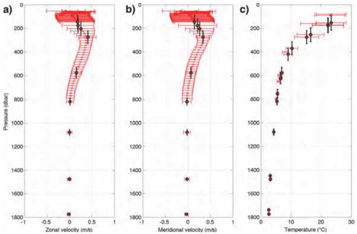
**Figure D1** – Solomon M1 vertical profiles averaged over time (red dots) within a two standard deviation uncertainty (red lines) of (a) zonal velocity; (b) meridional velocity and (c) temperature as a function of pressure. Note the two standard deviation uncertainty for pressure (black lines).
