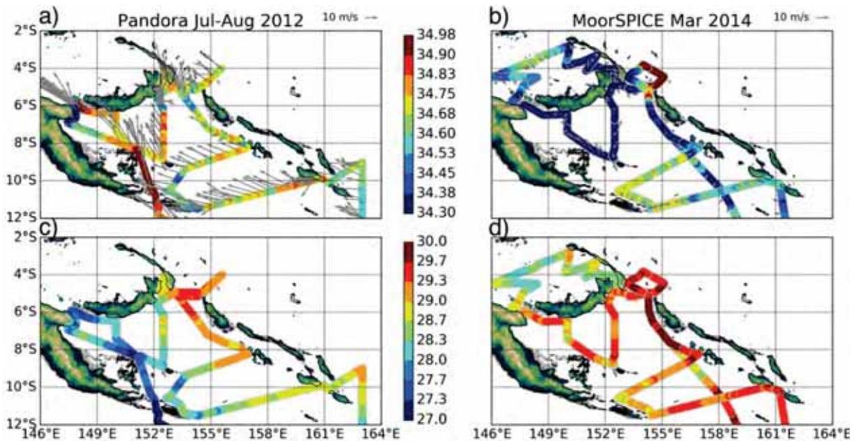
**Figure 3.5** – Observed along-track sea surface salinity (color scale, pss-78) from the Thermosalinograph (TSG) and in situ winds during (a) Pandora (July-August 2012) and (b) MoorSPICE (March 2014) cruises. Along track sea surface temperature (color scale, °C) from the hull during (c) Pandora and (d) MoorSPICE. Note the unit vector in the upper right of the top panels.
