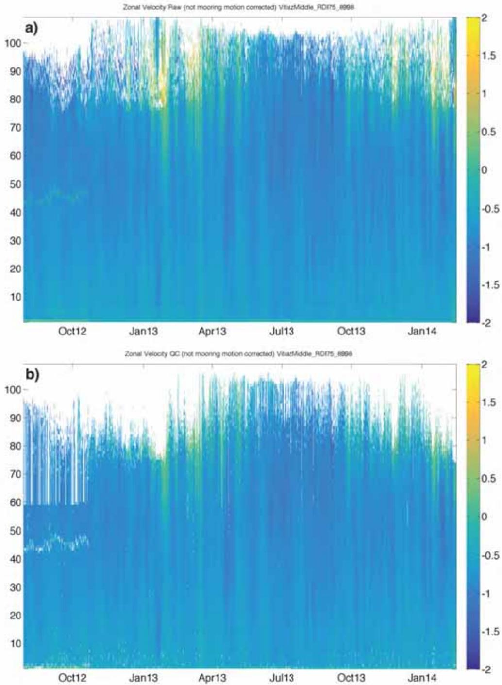
Figure 30 – Comparisons of zonal velocity ( $m.s^{-1}$ ) in Vitiāz Strait Middle, (a) raw zonal velocity and (b) QC zonal velocity of the upward RDI 75 kHz ADCP.
