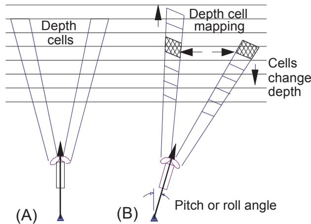
**Figure 6.4** – Schematic of the ADCP tilt induced by pitch and roll variations. The hatched cells in (B) indicate different depth cells than those in (A). From *Gordon and Instruments* (1996).
