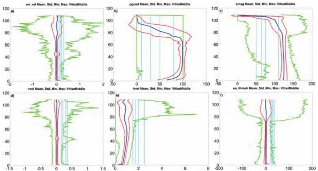
Figure 29 – Mean (thick blue line), standard deviation (red lines) and minimum and maximum (green lines) of the (a) error velocity ( $m.s^{-1}$ ); (b) percent good; (c) correlation magnitude; (d) vertical velocity ( $m.s^{-1}$ ); (e) horizontal velocity ( $m.s^{-1}$ ) and (f) echo amplitude (counts) for the Vitiast Strait Middle upward RDI 75 kHz ADCP versus bin. The four threshold values used in each QC test are marked by cyan lines in panels (a) to (f).
