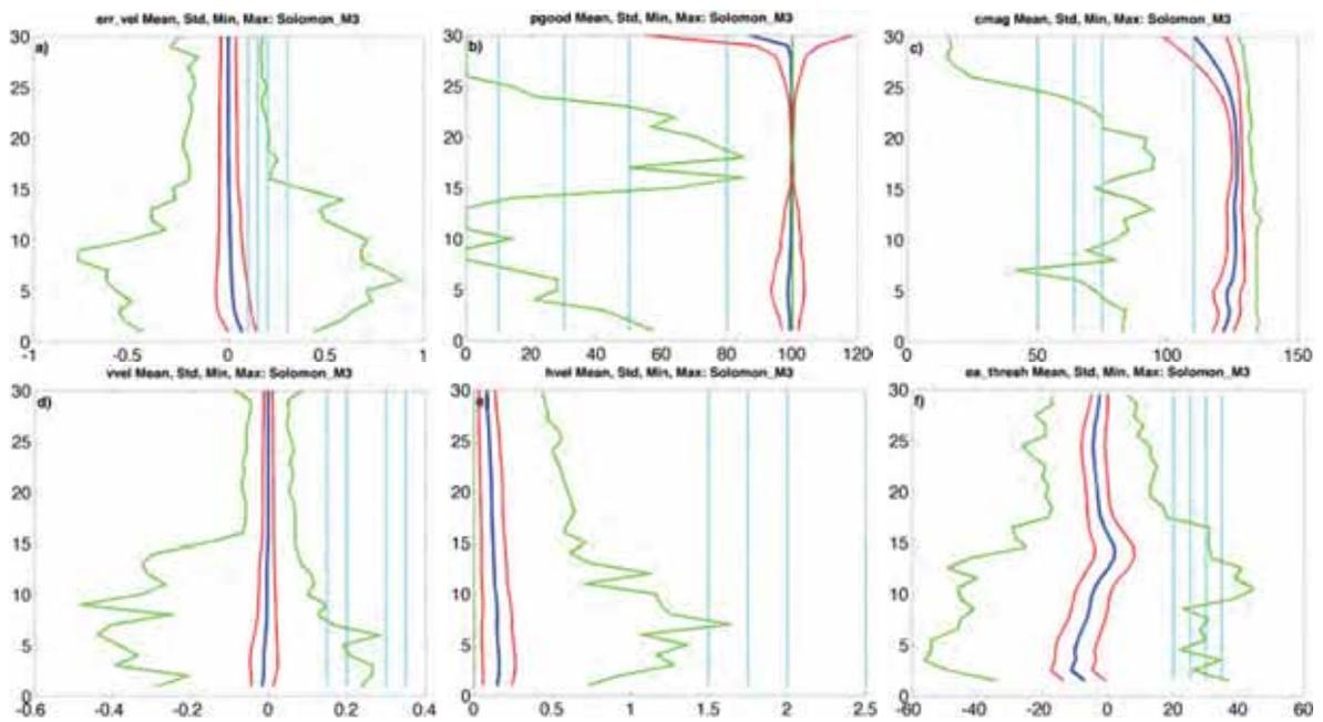
Figure 14 – Mean (thick blue line), standard deviation (red lines) and minimum and maximum (green lines) of the (a) error velocity ( $m.s^{-1}$ ); (b) percent good; (c) correlation magnitude; (d) vertical velocity ( $m.s^{-1}$ ); (e) horizontal velocity ( $m.s^{-1}$ ) and (f) echo amplitude (counts) for the Solomon Strait M3 RDI 75 kHz ADCP versus bin. The four threshold values used in each QC test are marked by cyan lines in panels (a) to (f).
