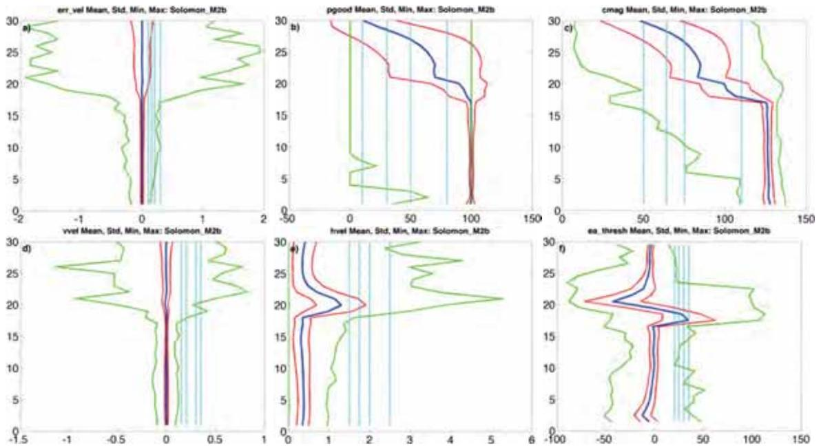
Figure 8 – Mean (thick blue line), standard deviation (red lines) and minimum and maximum (green lines) of the (a) error velocity ( $m.s^{-1}$ ); (b) percent good; (c) correlation magnitude; (d) vertical velocity ( $m.s^{-1}$ ); (e) horizontal velocity ( $m.s^{-1}$ ) and (f) echo amplitude (counts) for the Solomon Strait M2b RDI 75 kHz ADCP versus bin. The four threshold values used in each QC test are marked by cyan lines in panels (a) to (f).
