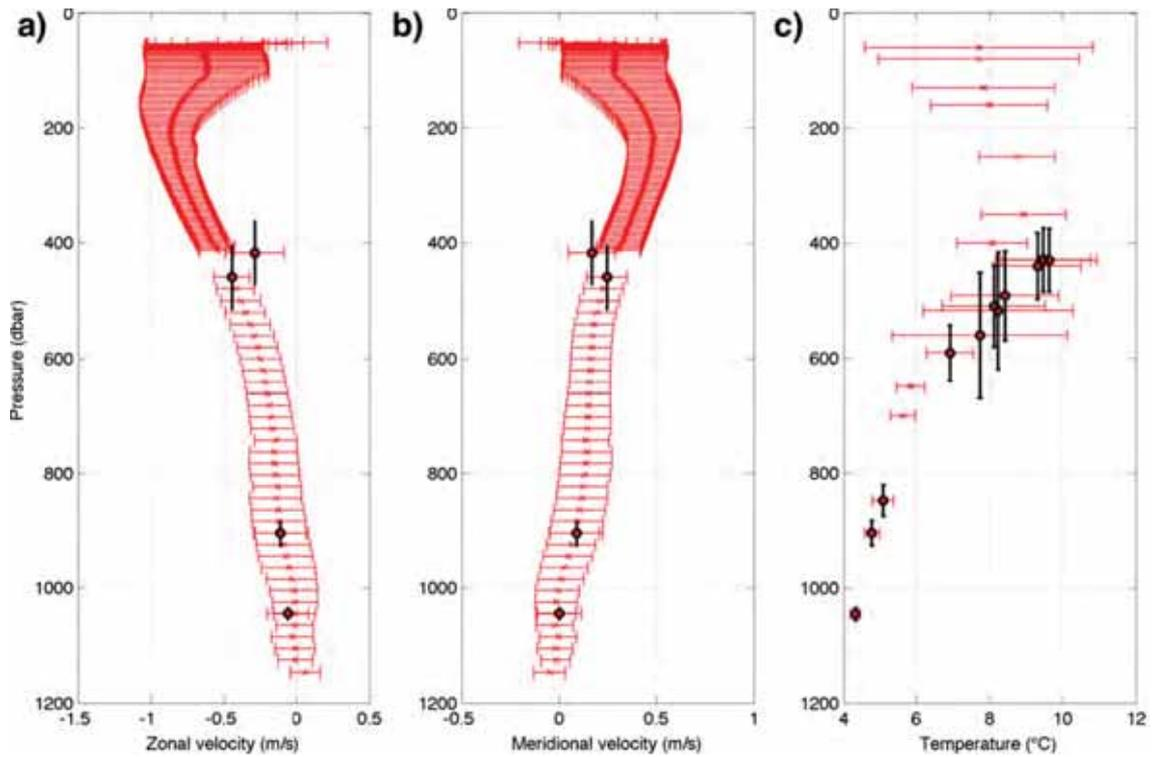
**Figure D8** – Vitiáz Middle vertical profiles averaged over time (red dots) within a two standard deviation uncertainty (red lines) of (a) zonal velocity; (b) meridional velocity and (c) temperature as a function of pressure. Note the two standard deviation uncertainty for pressure (black lines).
