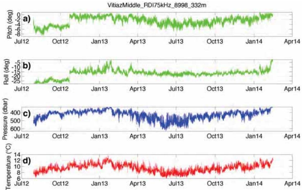
Figure 28 – Vitiast Strait Middle RDI 75 kHz (upward) raw data of (a) pitch; (b) roll; (c) pressure and (d) temperature timeseries.
