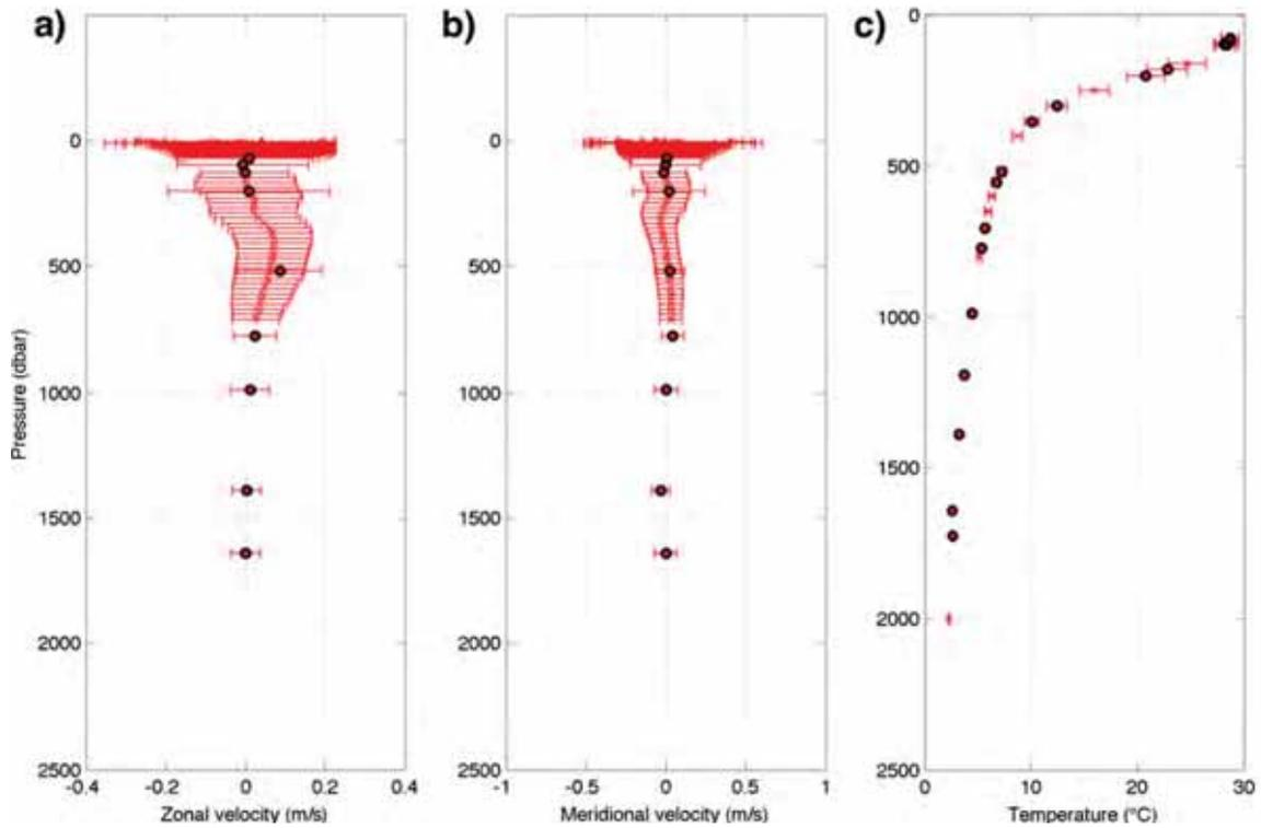
**Figure D4** – Solomon M3 vertical profiles averaged over time (red dots) within a two standard deviation uncertainty (red lines) of (a) zonal velocity; (b) meridional velocity and (c) temperature as a function of pressure. Note the two standard deviation uncertainty for pressure (black lines).
