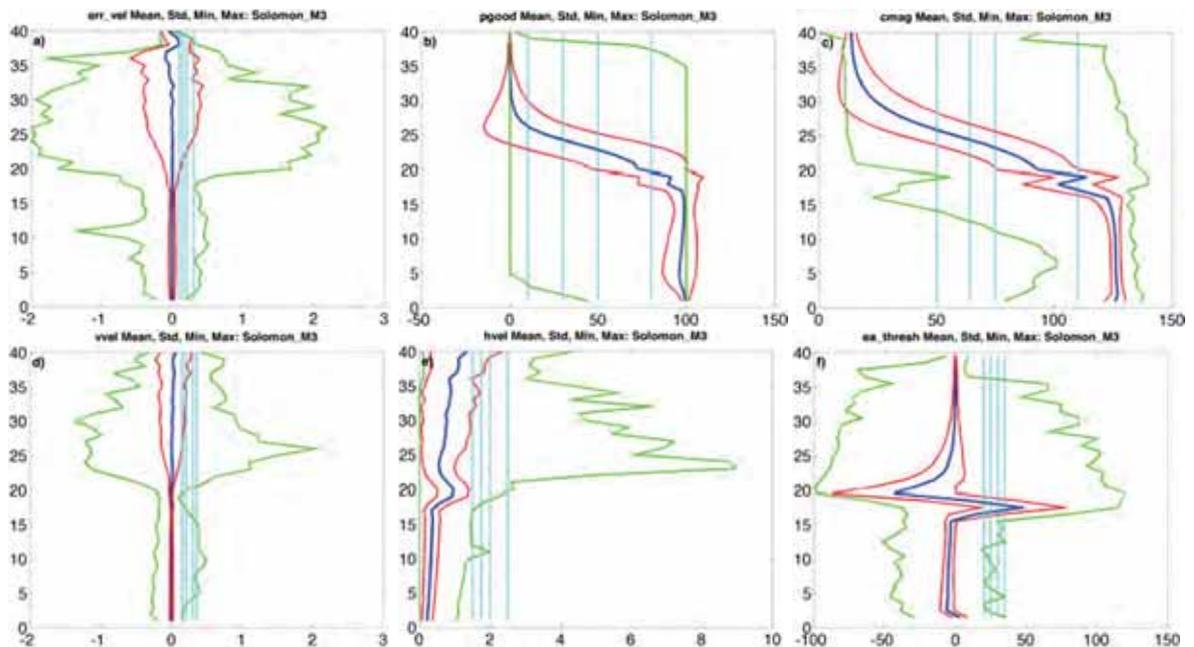
Figure 11 – Mean (thick blue line), standard deviation (red lines) and minimum and maximum (green lines) of the (a) error velocity ( $m.s^{-1}$ ); (b) percent good; (c) correlation magnitude; (d) vertical velocity ( $m.s^{-1}$ ); (e) horizontal velocity ( $m.s^{-1}$ ) and (f) echo amplitude (counts) for the Solomon Strait M3 RDI 300 kHz ADCP versus bin. The four threshold values used in each QC test are marked by cyan lines in panels (a) to (f).
