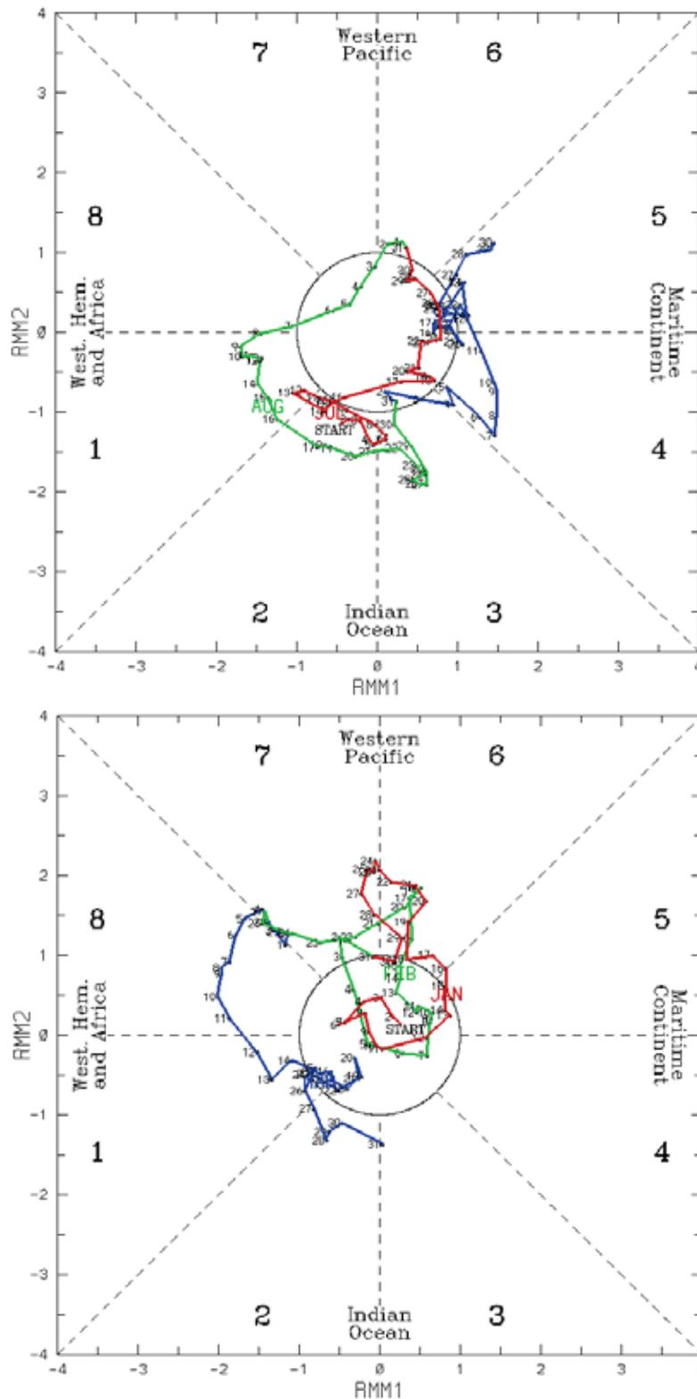
**Figure 3.4** – Diagram of the MJO phases during (a) July-September 2012 and (b) January-March 2014. The Real-time Multivariate MJO series 1 (RMM1) and 2 (RMM2) are a pair of principal component (PC) time series that combine cloud amount and winds at upper (200-hPa) and lower levels (850-hPa) of the atmosphere. Note labeled dots for each day, while color corresponds to each month as indicated in diagrams (a) and (b). From the Bureau of Meteorology, Commonwealth of Australia.
