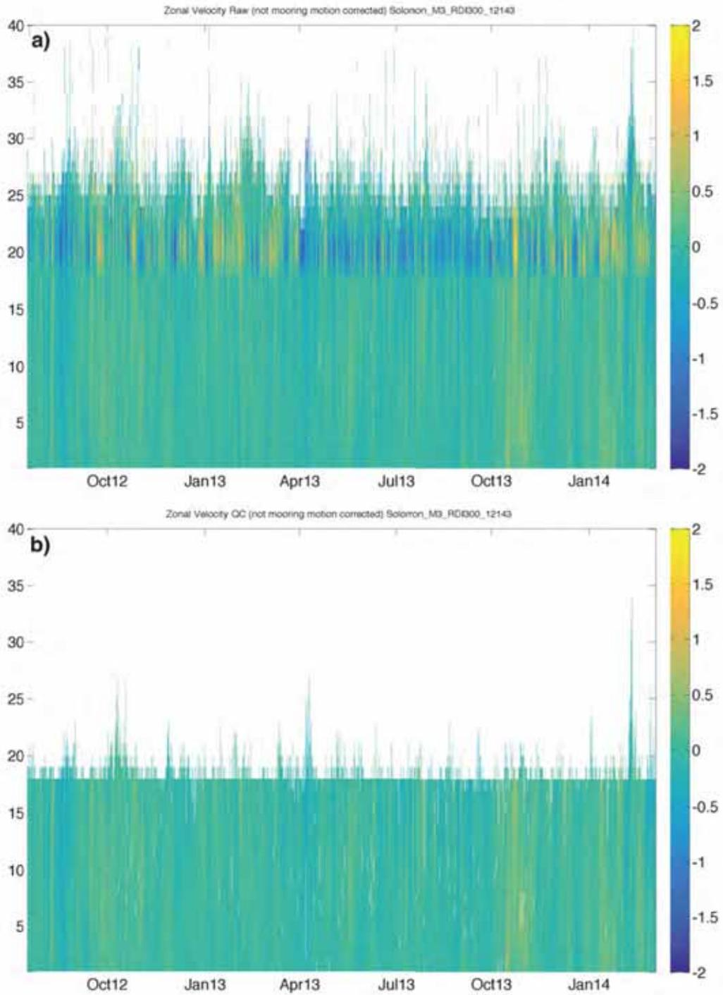
Figure 12 – Comparisons of zonal velocity ( $m.s^{-1}$ ) in Solomon Strait M3, (a) raw zonal velocity and (b) QC zonal velocity of the RDI 300 kHz ADCP.
