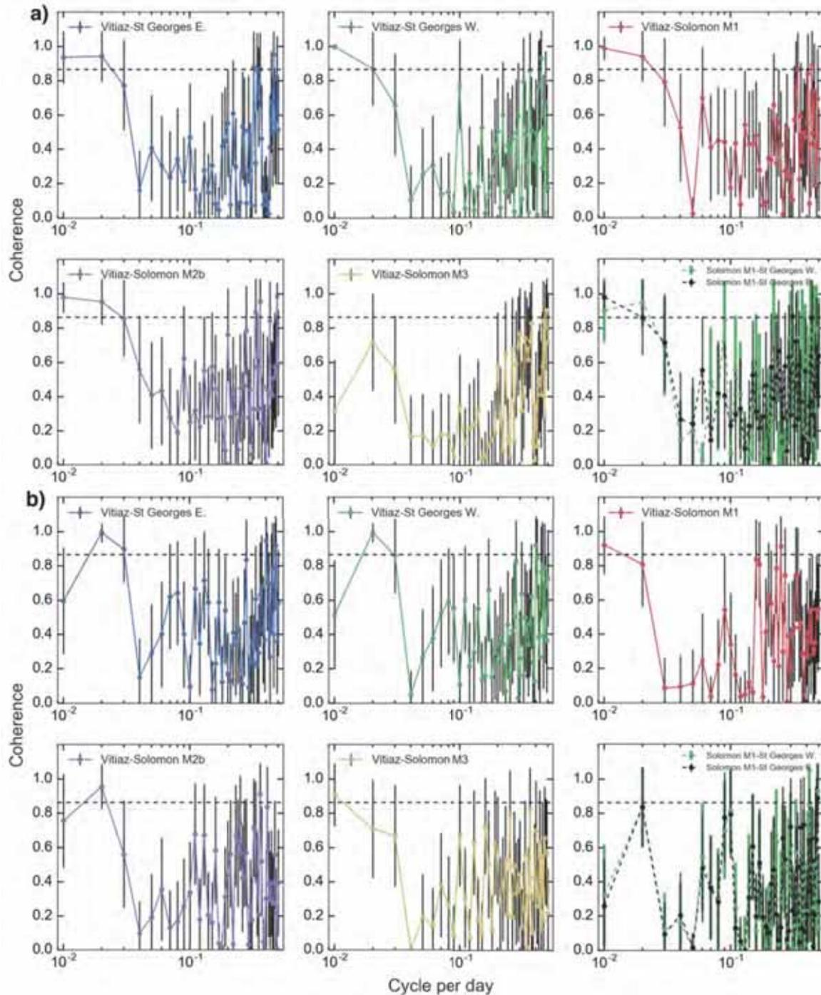
**Figure 6.12** – Spectral coherence computed for each MoorSPICE mooring at (a) the thermocline and (b) intermediate levels. Line colors indicate the selected pair of moorings as shown in legends. Error bars (black lines) are one standard deviation. The 95% confidence interval is indicated (dash lines) following *Emery and Thomson* (2001) (see text).
