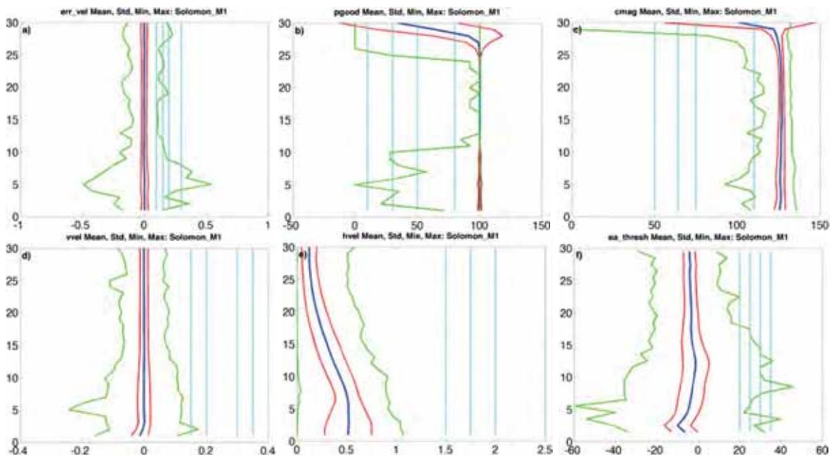
Figure 5 – Mean (thick blue line), standard deviation (red lines) and minimum and maximum (green lines) of the (a) error velocity ( $m.s^{-1}$ ); (b) percent good; (c) correlation magnitude; (d) vertical velocity ( $m.s^{-1}$ ); (e) horizontal velocity ( $m.s^{-1}$ ) and (f) echo amplitude (counts) for the Solomon Strait M1 RDI 75 kHz ADCP versus bin. The four threshold values used in each QC test are marked by cyan lines in panels (a) to (f).
