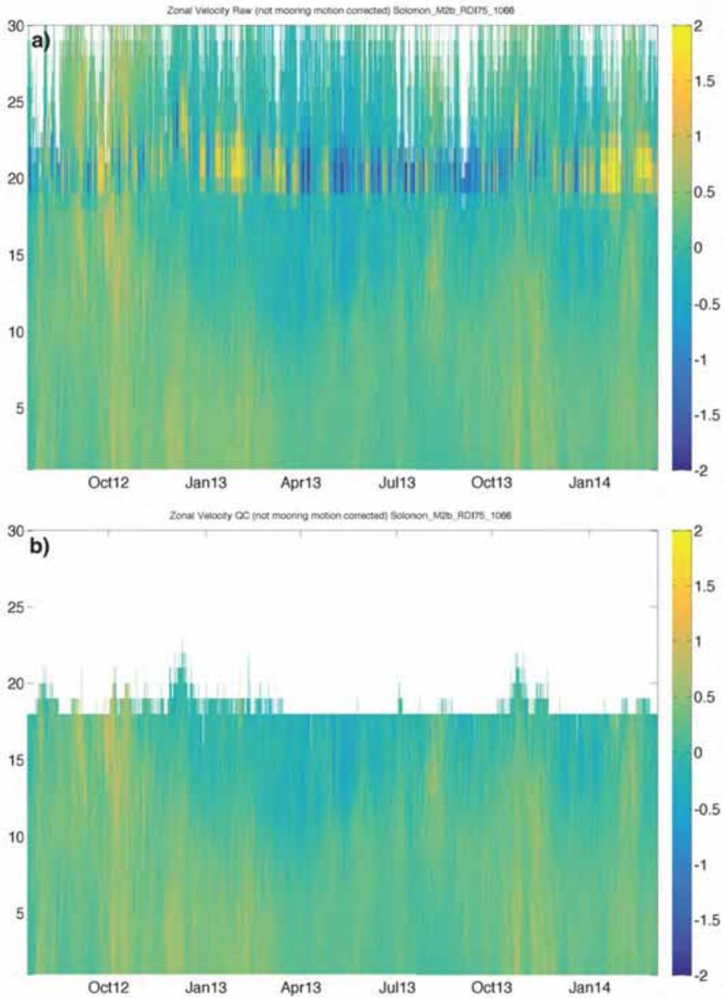
Figure 9 – Comparisons of zonal velocity ( $m.s^{-1}$ ) in Solomon Strait M2b, (a) raw zonal velocity and (b) QC zonal velocity of the RDI 75 kHz ADCP.
