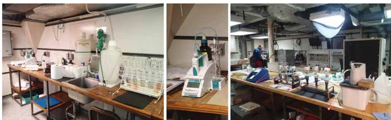
**Figure 2.3** – Pictures of the ship laboratory during MoorSPICE. Materials for measuring dissolved oxygen are shown in both left and middle panels. Salinity and other measurements such as phytoplankton pigments (right panel), were also carried out (photos: C. Germaineaud).
