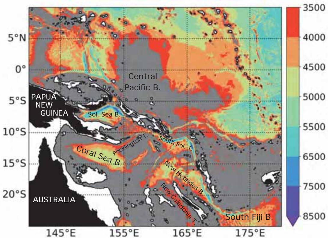
**Figure 5.2** – Southwest Pacific bathymetry at depths greater than 3500 m (color scale, meters). The 1000 m contour (black line) is shown. Areas shallower than 1000 m are in white. Grey shading shows areas deeper than 1000 m and shallower than 3500 m.
