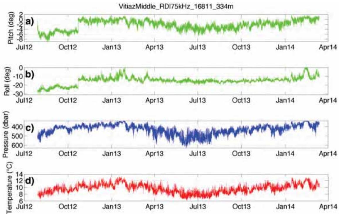
Figure 31 – Vitiast Strait Middle RDI 75 kHz (downward) raw data of (a) pitch; (b) roll; (c) pressure and (d) temperature timeseries.
