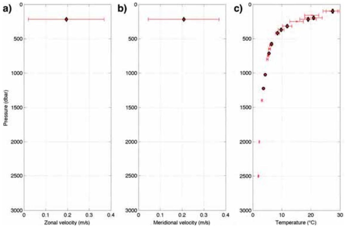
**Figure D2** – Solomon M2a vertical profiles averaged over time (red dots) within a two standard deviation uncertainty (red lines) of (a) zonal velocity; (b) meridional velocity and (c) temperature as a function of pressure. Note the two standard deviation uncertainty for pressure (black lines).
