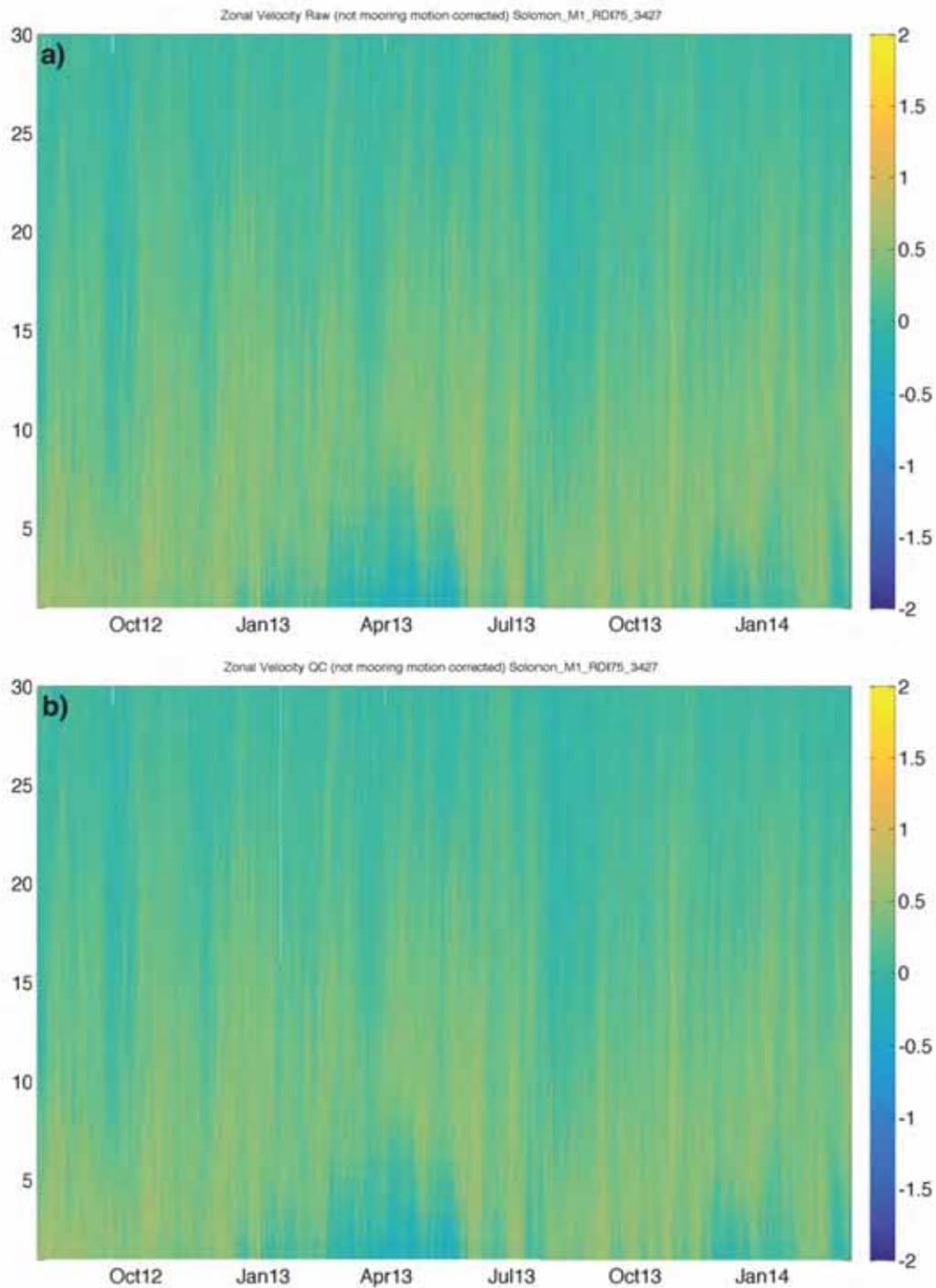
Figure 6 – Comparisons of zonal velocity ( $m.s^{-1}$ ) in Solomon Strait M1, (a) raw zonal velocity and (b) QC zonal velocity of the RDI 75 kHz ADCP.
