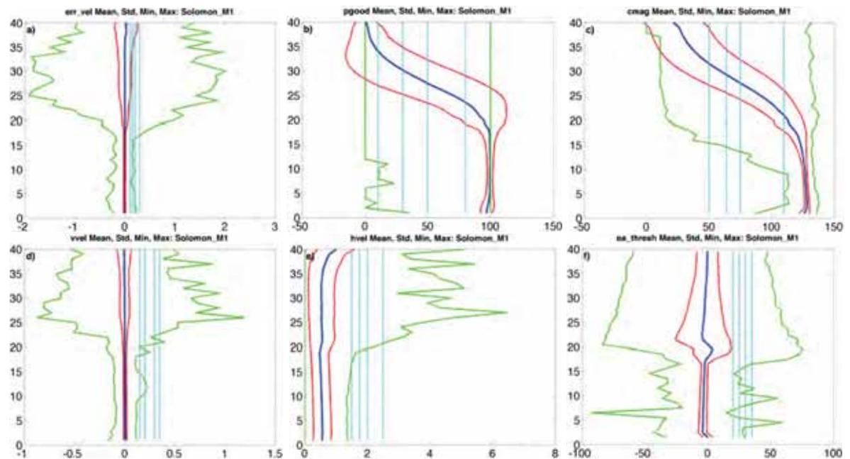
Figure 2 – Mean (thick blue line), standard deviation (red lines) and minimum and maximum (green lines) of the (a) error velocity ( $m.s^{-1}$ ); (b) percent good; (c) correlation magnitude; (d) vertical velocity ( $m.s^{-1}$ ); (e) horizontal velocity ( $m.s^{-1}$ ) and (f) echo amplitude (counts) for the Solomon Strait M1 RDI 300 kHz ADCP versus bin. The four threshold values used in each QC test are marked by cyan lines in panels (a) to (f).
