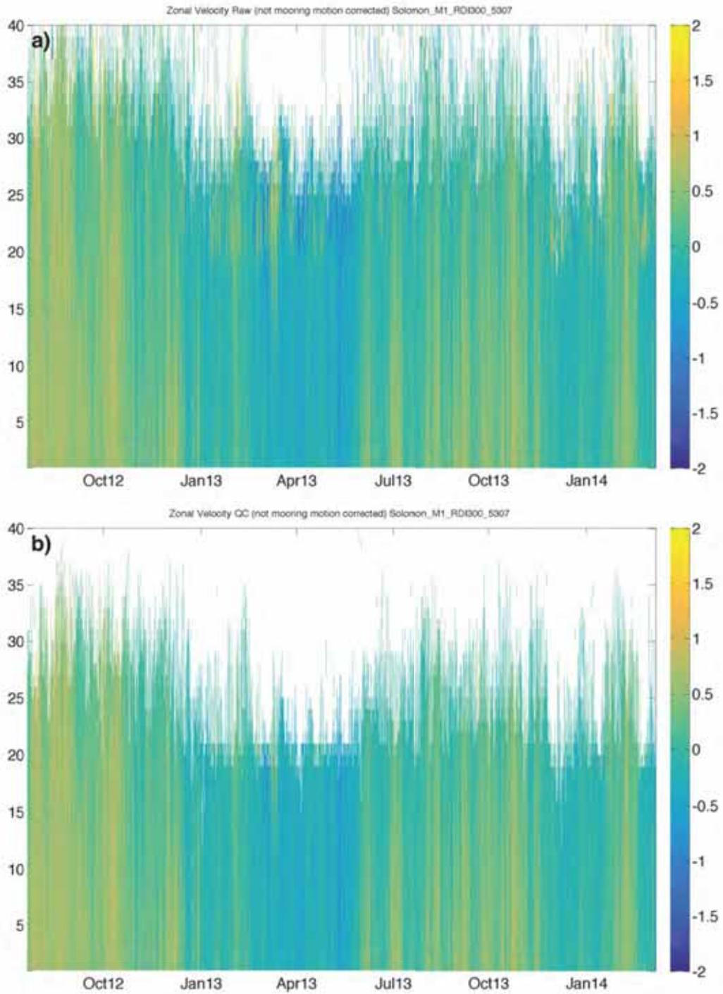
Figure 3 – Comparisons of zonal velocity ( $m.s^{-1}$ ) in Solomon Strait M1, (a) raw zonal velocity and (b) QC zonal velocity of the RDI 300 kHz ADCP.
