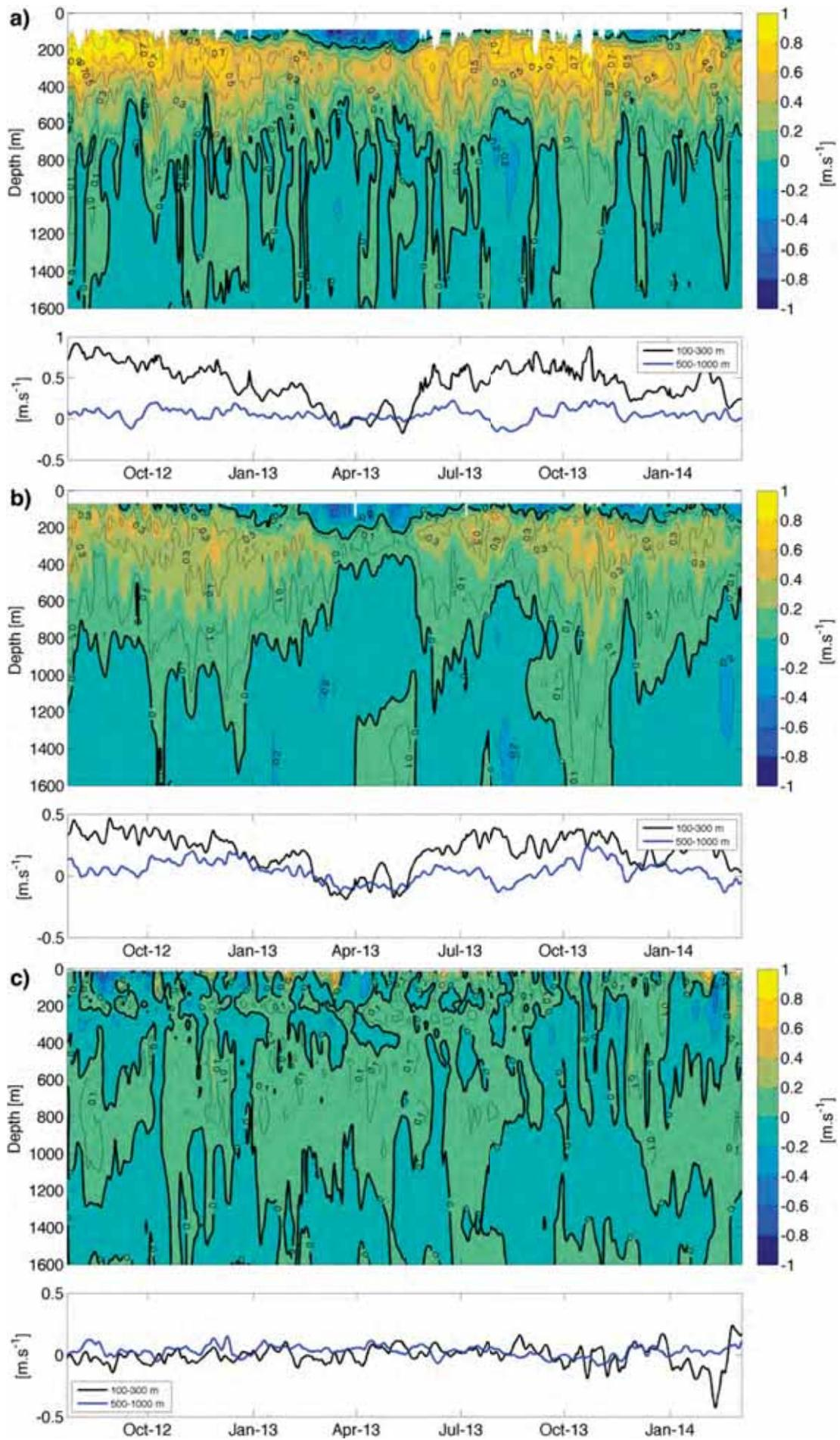
**Figure 6.10** – Timeseries of the gridded velocity field (color scale) rotated along the mean flow direction, after a low-pass filter with a 4-day Hamming window near the surface to 1600 m (top panel) and averaged over the thermocline (100-300 m, black line) and intermediate (500-1000 m, blue line) layers (bottom panels) at (a) Solomon M1, (b) Solomon M2b and (c) Solomon M3.
