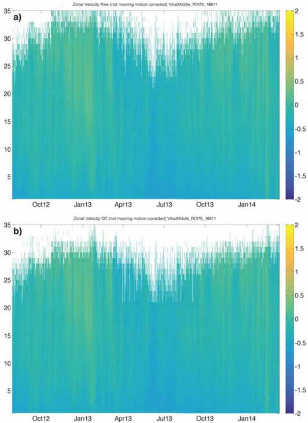
Figure 33 – Comparisons of zonal velocity ( $m.s^{-1}$ ) in Vitiaz Strait Middle, (a) raw zonal velocity and (b) QC zonal velocity of the downward RDI 75 kHz ADCP.
