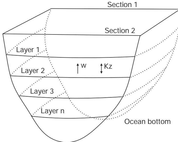
**Figure 2.5** – Schematic of the inverse model structure. The velocity field is estimated so that conservation requirements are met within isopycnal layers. Advective ( $w$ ) and diffusive ( $\kappa_z$ ) exchanges are allowed between layers.
