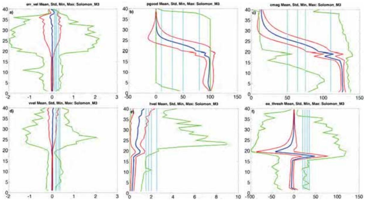
**Figure 6.6** – Mean (thick blue line), standard deviation (red lines) and minimum and maximum (green lines) of the (a) error velocity ( $m.s^{-1}$ ); (b) percent good; (c) correlation magnitude; (d) vertical velocity ( $m.s^{-1}$ ); (e) horizontal velocity ( $m.s^{-1}$ ) and (f) echo amplitude (counts) for the Solomon M3 upward ADCP versus bin. The four threshold values used in each quality control test are marked by cyan lines in panels (a) to (f).
