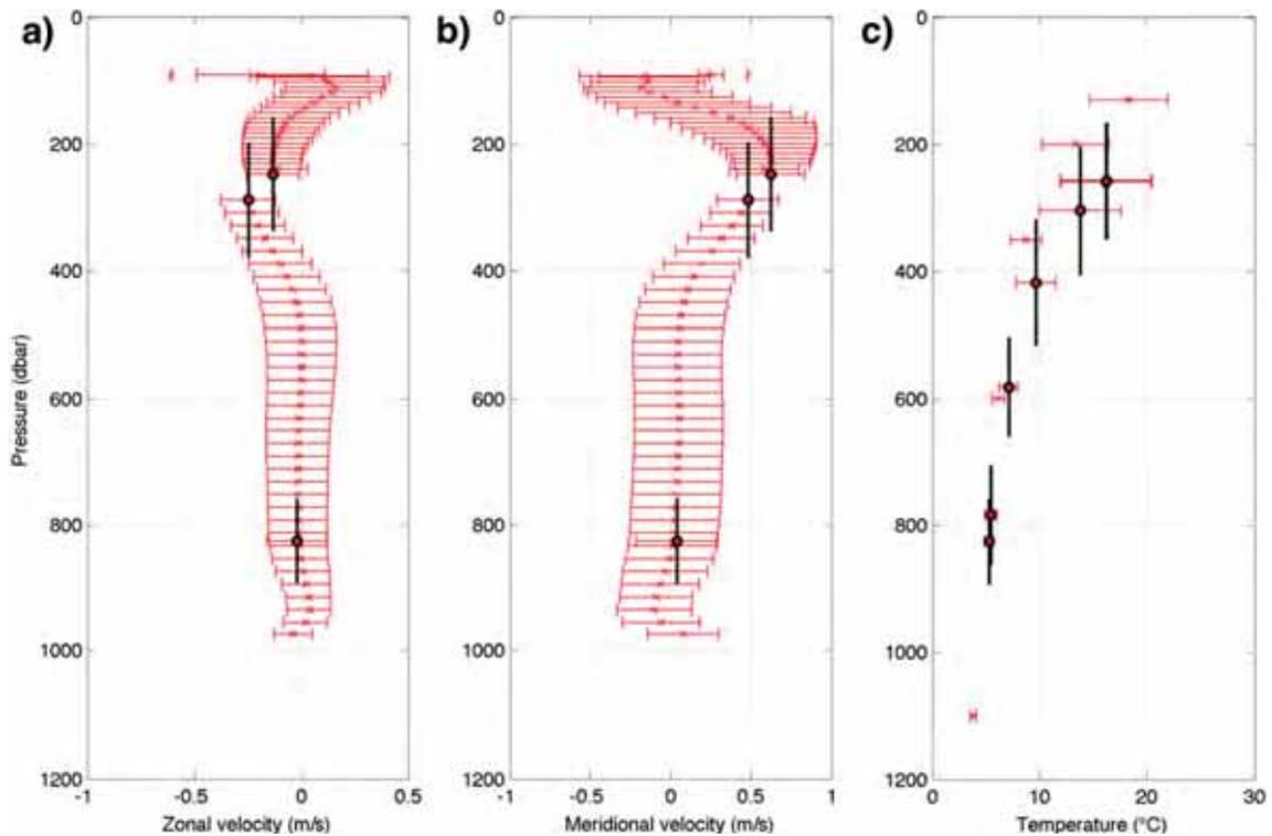
**Figure D5** – St Georges East vertical profiles averaged over time (red dots) within a two standard deviation uncertainty (red lines) of (a) zonal velocity; (b) meridional velocity and (c) temperature as a function of pressure. Note the two standard deviation uncertainty for pressure (black lines).
