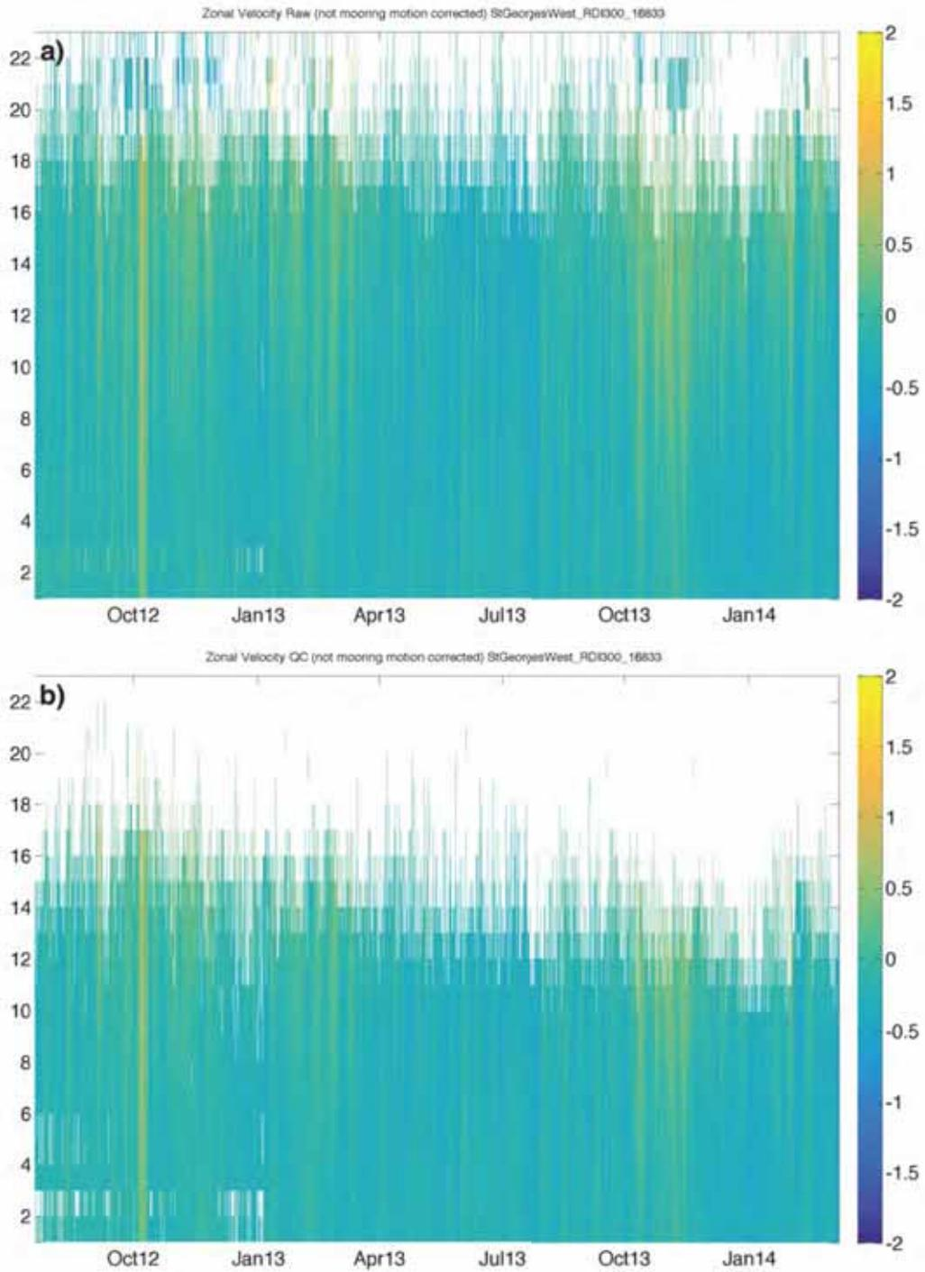
Figure 24 – Comparisons of zonal velocity ( $m.s^{-1}$ ) in St Georges Channel West, (a) raw zonal velocity and (b) QC zonal velocity of the RDI 300 kHz ADCP.
