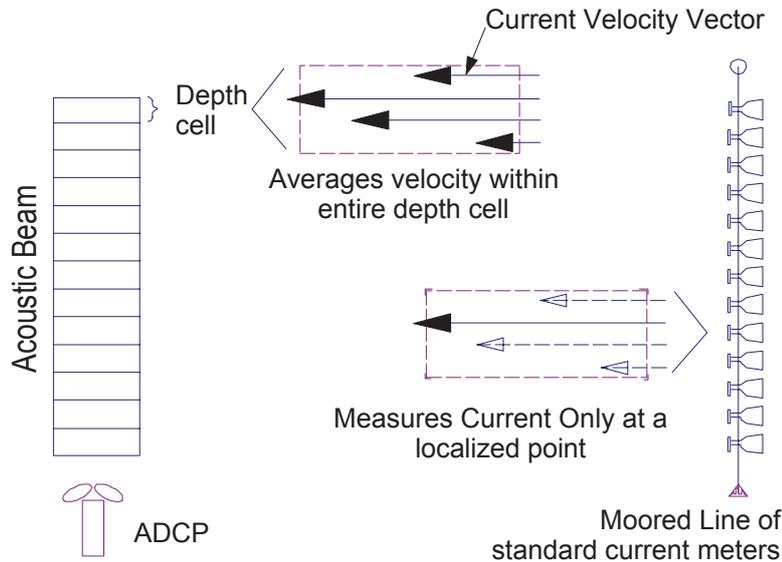
**Figure 6.3** – Schematic of the ADCP bins (depth cells) compared with discrete current meters on a mooring. From *Gordon and Instruments* (1996).
