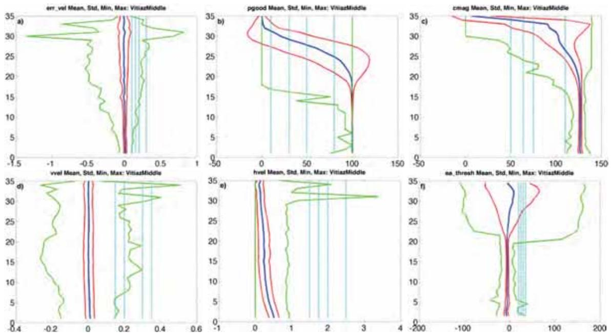
Figure 32 – Mean (thick blue line), standard deviation (red lines) and minimum and maximum (green lines) of the (a) error velocity ( $m.s^{-1}$ ); (b) percent good; (c) correlation magnitude; (d) vertical velocity ( $m.s^{-1}$ ); (e) horizontal velocity ( $m.s^{-1}$ ) and (f) echo amplitude (counts) for the Vitiast Strait Middle downward RDI 75 kHz ADCP versus bin. The four threshold values used in each QC test are marked by cyan lines in panels (a) to (f).
