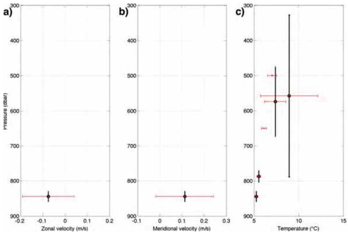
**Figure D9** – Vitiáz West vertical profiles averaged over time (red dots) within a two standard deviation uncertainty (red lines) of (a) zonal velocity; (b) meridional velocity and (c) temperature as a function of pressure. Note the two standard deviation uncertainty for pressure (black lines).
