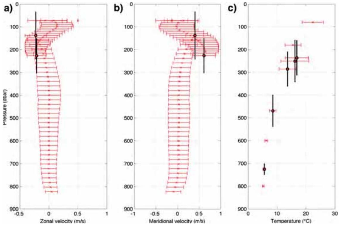
**Figure D6** – St Georges West vertical profiles averaged over time (red dots) within a two standard deviation uncertainty (red lines) of (a) zonal velocity; (b) meridional velocity and (c) temperature as a function of pressure. Note the two standard deviation uncertainty for pressure (black lines).
