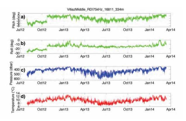
Figure 31 – Vitiaz Strait Middle RDI 75 kHz (downward) raw data of (a) pitch; (b) roll; (c) pressure and (d) temperature timeseries.
