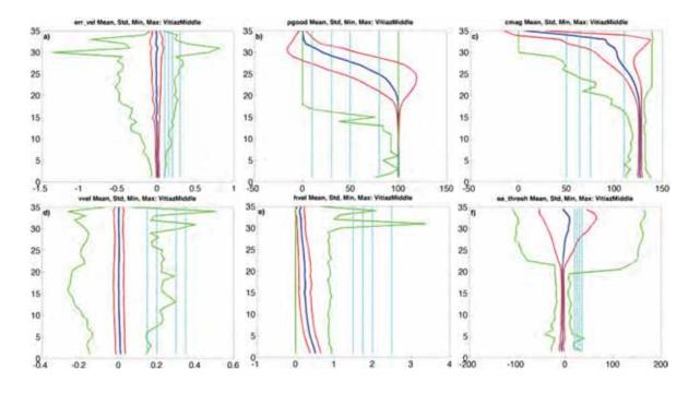
Figure 32 – Mean (thick blue line), standard deviation (red lines) and minimum and maximum (green lines) of the (a) error velocity  $(m.s^{-1})$ ; (b) percent good; (c) correlation magnitude; (d) vertical velocity  $(m.s^{-1})$ ; (e) horizontal velocity  $(m.s^{-1})$  and (f) echo amplitude (counts) for the Vitiaz Strait Middle downward RDI 75 kHz ADCP versus bin. The four threshold values used in each QC test are marked by cyan lines in panels (a) to (f).
