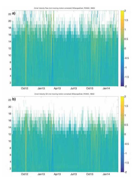
Figure 18 – Comparisons of zonal velocity  $(m.s^{-1})$  in St Georges Channel East, (a) raw zonal velocity and (b) QC zonal velocity of the RDI 300 kHz ADCP.
