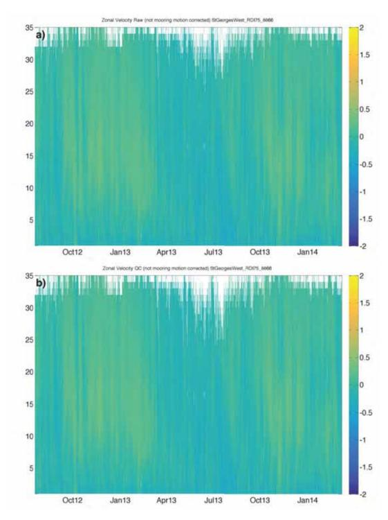
Figure 27 – Comparisons of zonal velocity  $(m.s^{-1})$  in St Georges Channel West, (a) raw zonal velocity and (b) QC zonal velocity of the RDI 75 kHz ADCP.
