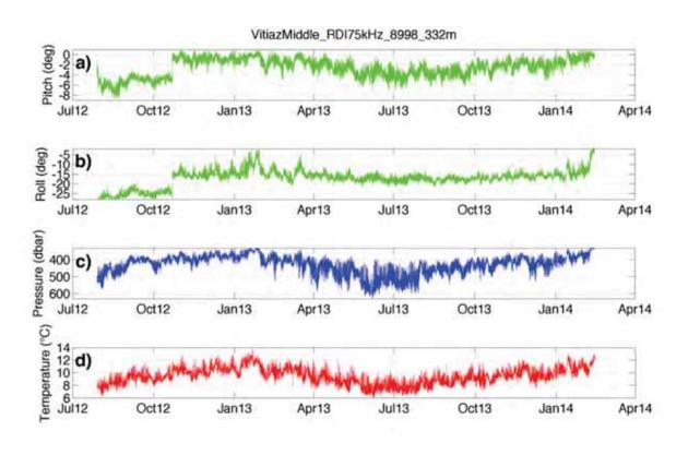
Figure 28 – Vitiaz Strait Middle RDI 75 kHz (upward) raw data of (a) pitch; (b) roll; (c) pressure and (d) temperature timeseries.
