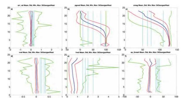
Figure 23 – Mean (thick blue line), standard deviation (red lines) and minimum and maximum (green lines) of the (a) error velocity  $(m.s^{-1})$ ; (b) percent good; (c) correlation magnitude; (d) vertical velocity  $(m.s^{-1})$ ; (e) horizontal velocity  $(m.s^{-1})$  and (f) echo amplitude (counts) for the St Georges Channel West RDI 300 kHz ADCP versus bin. The four threshold values used in each QC test are marked by cyan lines in panels (a) to (f).
