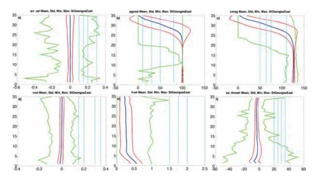
Figure 20 – Mean (thick blue line), standard deviation (red lines) and minimum and maximum (green lines) of the (a) error velocity  $(m.s^{-1})$ ; (b) percent good; (c) correlation magnitude; (d) vertical velocity  $(m.s^{-1})$ ; (e) horizontal velocity  $(m.s^{-1})$  and (f) echo amplitude (counts) for the St Georges Channel East RDI 75 kHz ADCP versus bin. The four threshold values used in each QC test are marked by cyan lines in panels (a) to (f).
