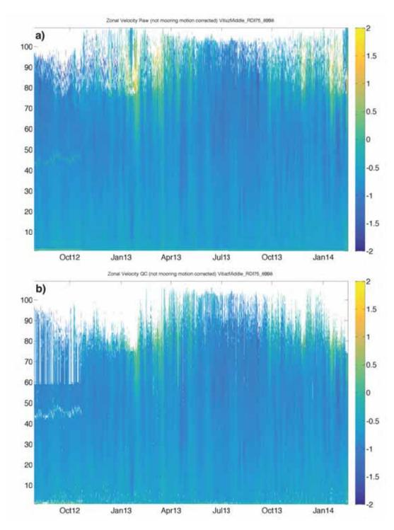
Figure 30 – Comparisons of zonal velocity  $(m.s^{-1})$  in Vitiaz Strait Middle, (a) raw zonal velocity and (b) QC zonal velocity of the upward RDI 75 kHz ADCP.
