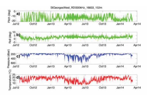
Figure 22 – St Georges Channel West RDI 300 kHz (upward) raw data of (a) pitch; (b) roll; (c) pressure and (d) temperature timeseries.
