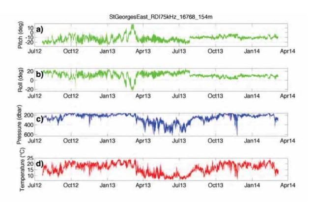
Figure 19 – St Georges Channel East RDI 75 kHz (downward) raw data of (a) pitch; (b) roll; (c) pressure and (d) temperature timeseries.
