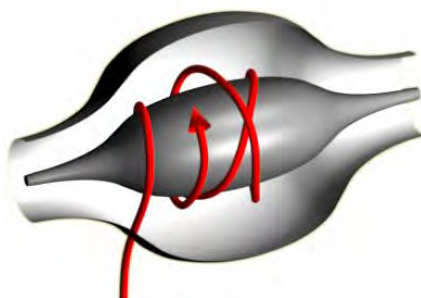
Figure II.B-4: Schematic view of the orbitrap. The red arrow shows the complex spiral trajectory of the ion around the inner electrode.
