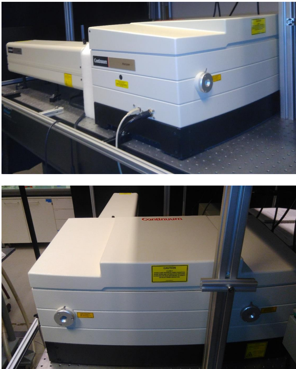
Figure 3.3.1. Horizon OPO and Surelite laser, in foreground and background respectively.
