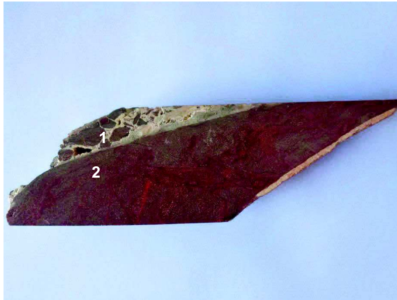
Figure 6.12 Core sample from a sandstone in the Buntsandstein at 1,204-m depth in the well EPS-1. The core sample exhibits a part of a fracture zone (1) and its damage zone (2). Barite and galena fill the hydraulic breccia. The diameter of the core sample is 8 cm.
