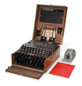
Figure 2.4: A four-rotor ENIGMA machine.
