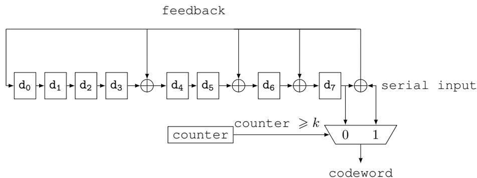
Figure 5.6: Standard LFSR architecture block diagram. (Design BCH-LFSR)
