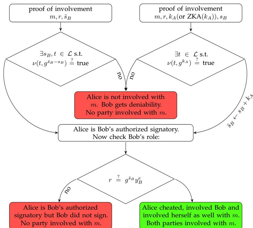
Figure 4.5: The verification procedure: **proof of involvement**.
