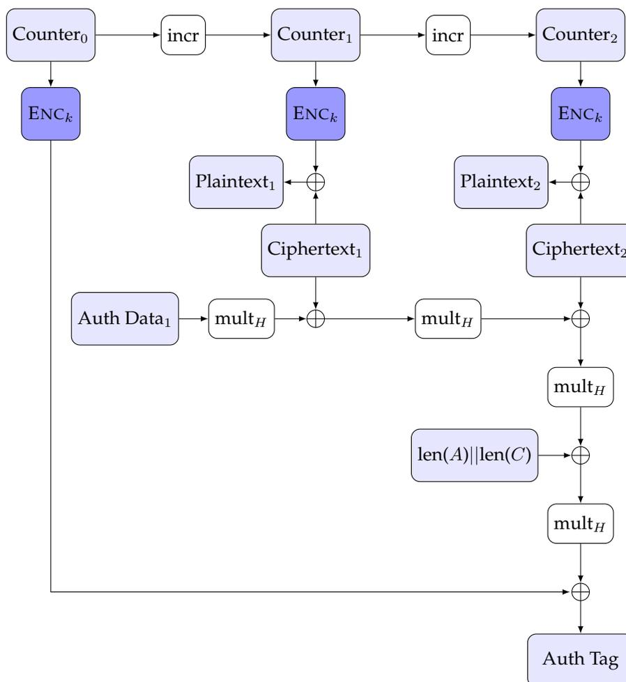
Figure 3.2: The GCM authenticated mode of operation - DECRYPT.
