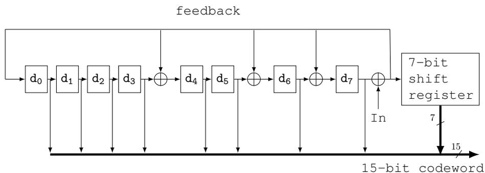
Figure 5.7: Improved LFSR architecture block diagram. In denotes the module's serial input. (Design BCH-LFSR-improved)
