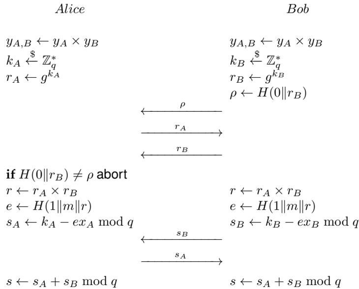
Figure 4.2: Generating the Schnorr co-signature of message  $m$ .
