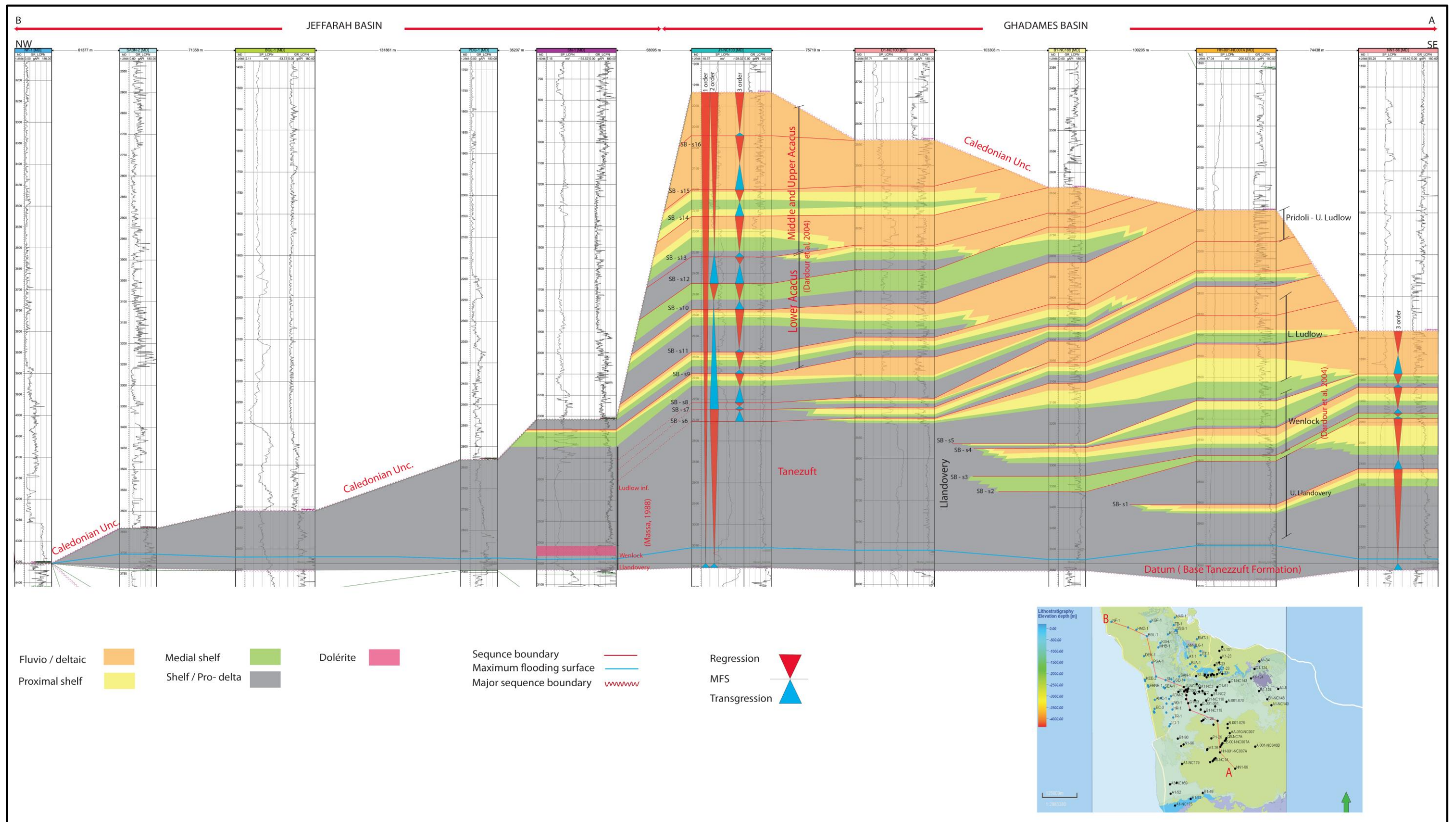
Figure 4.9: SE-NW cross section of the Silurian illustrating the depositional environment and sequence stratigraphy.
