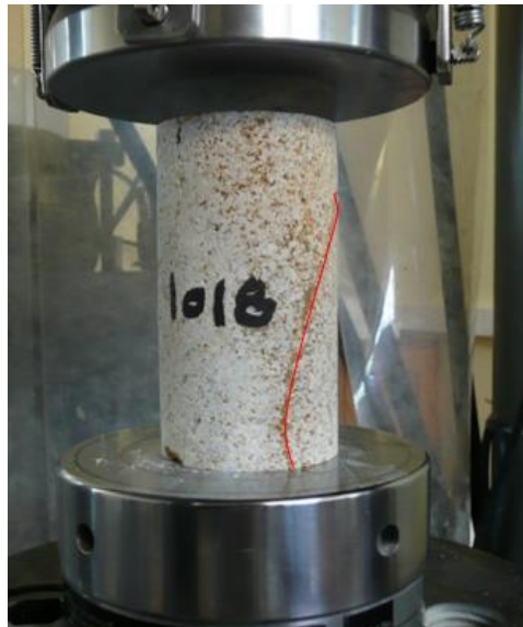
Figure 3-1 Discontinuity in sample 1018
