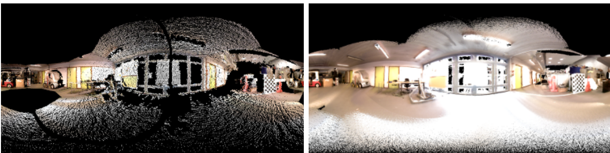
Figure 7.7 – Virtual keyframe fusion example. The left image depicts the initial keyframe. The resulting keyframe after fusion of the nearby frames is shown in the right. Observe that the occlusions are handled using this representation and the final model is a more complete keyframe with a bigger region of interest.
