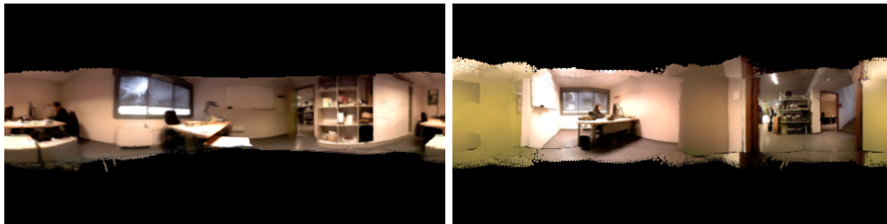
Figure 7.8 – Virtual keyframe examples with smaller coverage radius. The first virtual keyframe from the left depicts the office with few nearby frames included in the radius of visibility. The second image is the resulting keyframe in a door crossing, which also has a small radius of visibility.
