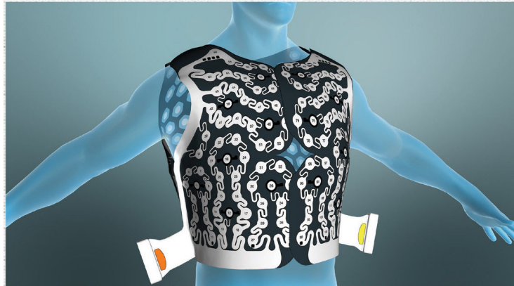
Figure 1.9: CardioInsight device for body surface potential mapping. (ECVUE, CardioInsight Technologies Inc., Cleveland, Ohio)
