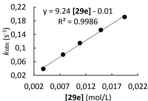
**Table S15.** Kinetics of the reaction of **29e** with **28c** (CH<sub>2</sub>Cl<sub>2</sub>, 20°C, stopped-flow, detection at 671 nm)
