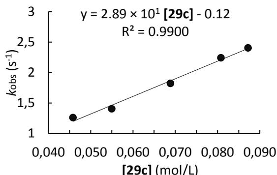
**Table S9.** Kinetics of the reaction of **29c** with **28b** (CH<sub>2</sub>Cl<sub>2</sub>, 20°C, stopped-flow, detection at 586 nm)
