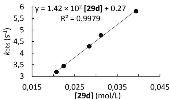
**Table S13.** Kinetics of the reaction of **29d** with **28b** (CH<sub>2</sub>Cl<sub>2</sub>, 20°C, stopped-flow, detection at 586 nm)
