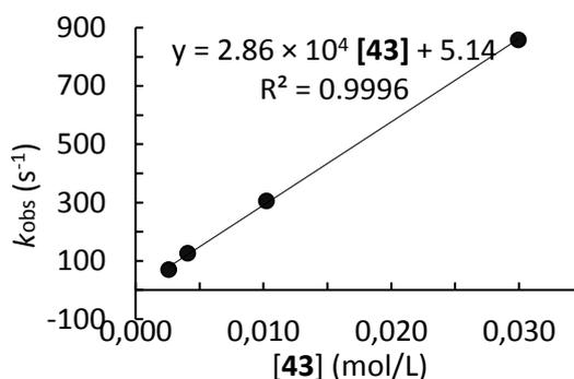
**Table S2.** Kinetics of the reaction of **43** with **41e** (CH<sub>3</sub>CN, 20°C, stopped-flow, detection at 616 nm).
