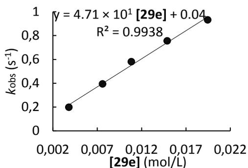
**Table S16.** Kinetics of the reaction of **29e** with **28b** (CH<sub>2</sub>Cl<sub>2</sub>, 20°C, stopped-flow, detection at 586 nm)
