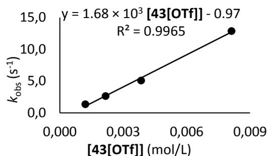
**Table S15.** Kinetics of the reaction of **43[OTf]** with **41f** (CH<sub>2</sub>Cl<sub>2</sub> 20°C, stopped-flow, detection at 642 nm)
