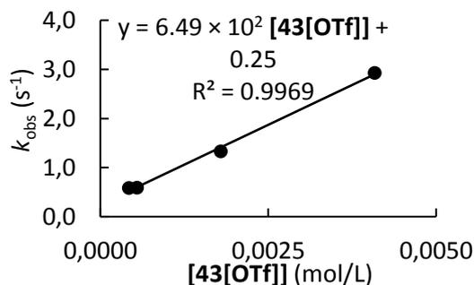
**Table S10.** Kinetics of the reaction of **D-43b[OTf]** with **41d** (CH<sub>3</sub>CN, 20°C, stopped-flow, detection at 612 nm)
