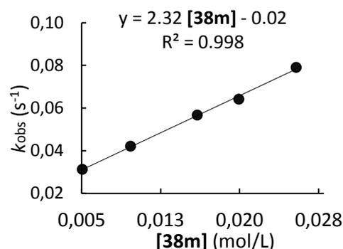
**Table S3.** Kinetics of the reaction of **38m** with **41c** (CH<sub>2</sub>Cl<sub>2</sub>, 20°C, stopped-flow, detection at 619 nm)
