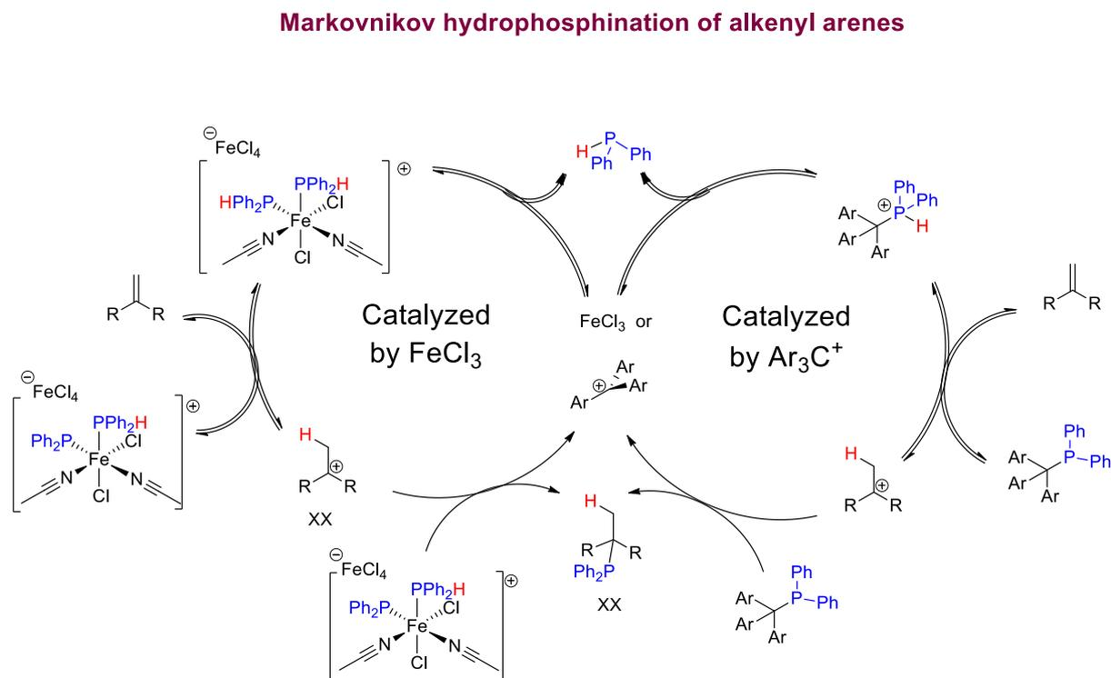
Scheme 5.16 Comparison of the Markovnikov catalyzed hydrophosphination of alkenes with  $\text{HPPh}_2$  catalysed by  $\text{FeCl}_3$  or  $[\text{Ar}_3\text{C}][\text{BF}_4]$ . Acetonitrile have been added as it is the solvent.
