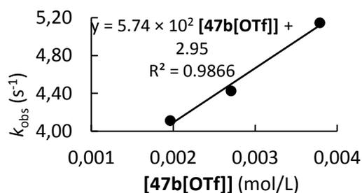
**Table S20.** Kinetics of the reaction of **47b[OTf]** with **41e** (CH<sub>3</sub>CN, 20°C, stopped-flow, detection at 616 nm)
