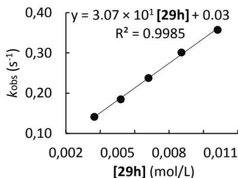
**Table S22.** Kinetics of the reaction of **29h** with **28b** (CH<sub>2</sub>Cl<sub>2</sub>, 20°C, stopped-flow, detection at 586 nm)
