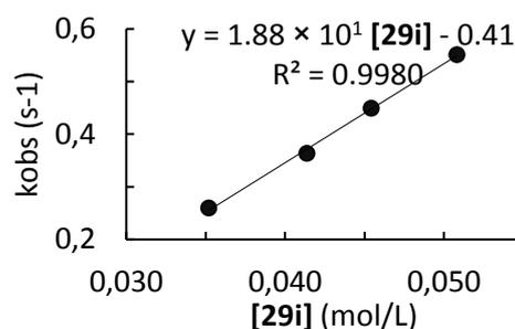
**Table S23.** Kinetics of the reaction of **29i** with **28d** (CH<sub>2</sub>Cl<sub>2</sub>, 20°C, stopped-flow, detection at 619 nm)
