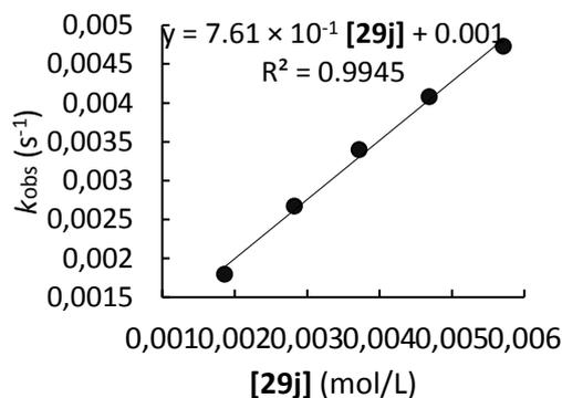
**Table S25.** Kinetics of the reaction of **29j** with **28b** (CH<sub>2</sub>Cl<sub>2</sub>, 20°C, stopped-flow, detection at 586 nm)
