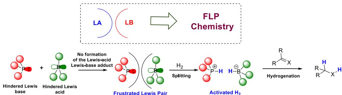
Figure 2 General figure of the first part: FLP chemistry.
