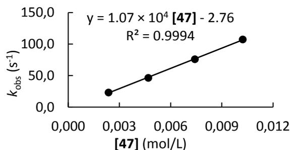
**Table S18.** Kinetics of the reaction of **47** with **41f** (CH<sub>3</sub>CN, 20°C, stopped-flow, detection at 642 nm)
