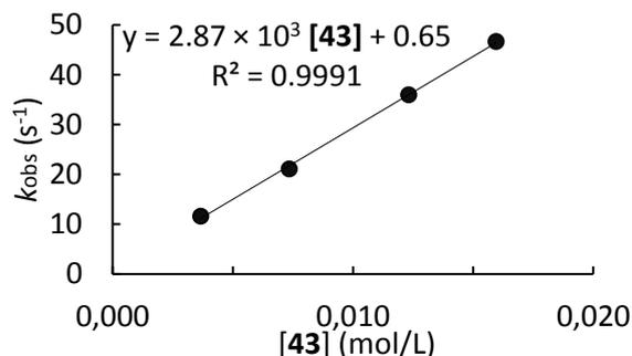
**Table S3.** Kinetics of the reaction of **43** with **41f** (CH<sub>3</sub>CN, 20°C, stopped-flow, detection at 642 nm).
