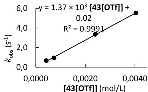
**Table S9.** Kinetics of the reaction of **43[OTf]** with **41f** (CH<sub>3</sub>CN, 20°C, stopped-flow, detection at 642 nm)
