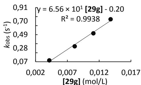
**Table S29.** Kinetics of the reaction of **29g** with **28b** (CH<sub>2</sub>Cl<sub>2</sub>, 20°C, stopped-flow, detection at 586 nm)
