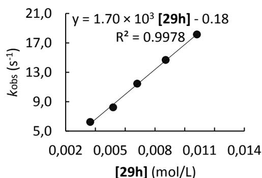
**Table S23.** Kinetics of the reaction of **29h** with **28a** (CH<sub>2</sub>Cl<sub>2</sub>, 20°C, stopped-flow, detection at 601 nm)
