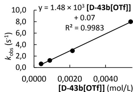
**Table S12.** Kinetics of the reaction of **D-43b[OTf]** with **41f** (CH<sub>3</sub>CN, 20°C, stopped-flow, detection 642 nm)
