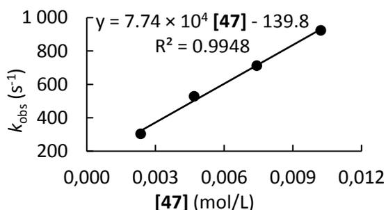
**Table S17.** Kinetics of the reaction of **47** with **41e** (CH<sub>3</sub>CN, 20°C, stopped-flow, detection at 616 nm)
