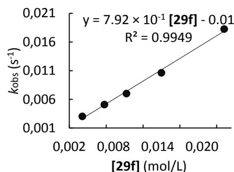
**Table S18.** Kinetics of the reaction of **29f** with **28c** (CH<sub>2</sub>Cl<sub>2</sub>, 20°C, stopped-flow, detection at 671 nm).
