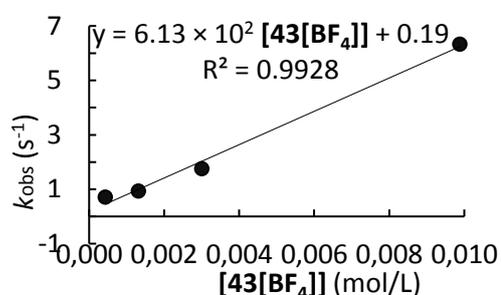
**Table S7.** Kinetics of the reaction of **43[OTf]** with **41d** (CH<sub>3</sub>CN 20°C, stopped-flow, detection at 612 nm)
