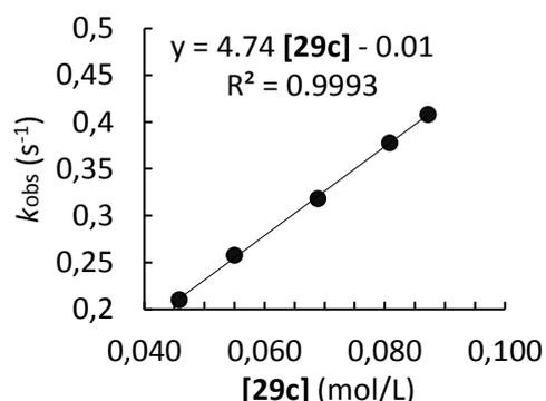
**Table S8.** Kinetics of the reaction of **29c** with **28c** (CH<sub>2</sub>Cl<sub>2</sub>, 20°C, stopped-flow, detection at 671 nm)
