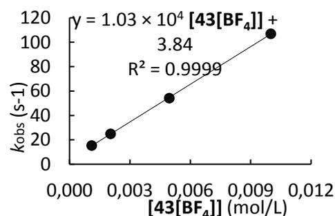
**Table S5.** Kinetics of the reaction of **43[BF<sub>4</sub>]** with **41e** (CH<sub>3</sub>CN 20°C, stopped-flow, detection at 616 nm)
