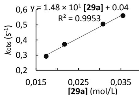
**Table S3.** Kinetics of the reaction of **29a** with **28b** (CH<sub>2</sub>Cl<sub>2</sub>, 20°C, stopped-flow, detection at 586 nm)
