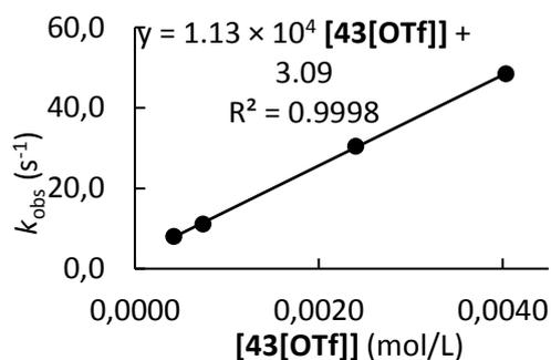
**Table S8.** Kinetics of the reaction of **43[OTf]** with **41e** (CH<sub>3</sub>CN 20°C, stopped-flow, detection at 616 nm)
