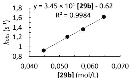
**Table S5.** Kinetics of the reaction of **29b** with **28c** (CH<sub>2</sub>Cl<sub>2</sub>, 20°C, stopped-flow, detection at 671 nm).
