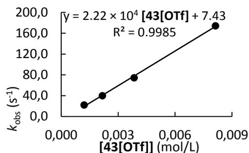
**Table S14.** Kinetics of the reaction of **43[OTf]** with **41e** (CH<sub>2</sub>Cl<sub>2</sub> 20°C, stopped-flow detection at 616 nm)
