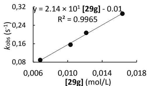
**Table S28.** Kinetics of the reaction of **29g** with **28c** (CH<sub>2</sub>Cl<sub>2</sub>, 20°C, stopped-flow, detection at 671 nm)
