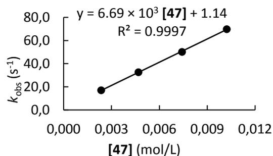
**Table S19.** Kinetics of the reaction of **47b[OTf]** with **41d** (CH<sub>3</sub>CN, 20°C, stopped-flow, detection at 612 nm)
