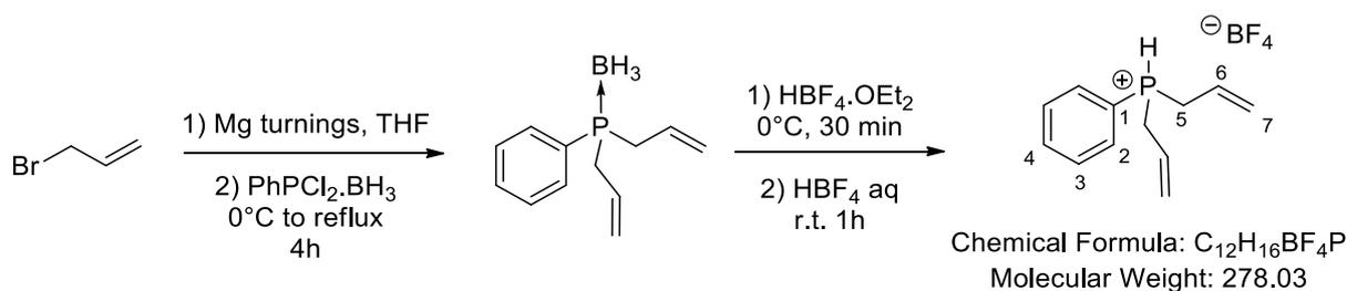
The synthesis was done in two steps. The synthesis of diallylphenylphosphine borane complex was done following a procedure reported by Gouverneur.<sup>3</sup> The synthesis of diallylphenylphosphonium tetrafluoroborate salt **49** was done following a procedure by Denmark.<sup>4</sup>
