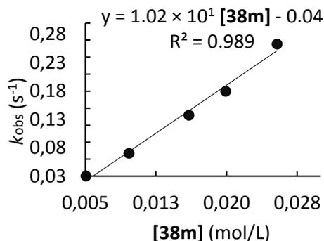
**Table S2.** Kinetics of the reaction of **38m** with **41b** (CH<sub>2</sub>Cl<sub>2</sub>, 20°C, stopped-flow, detection at 572 nm)
