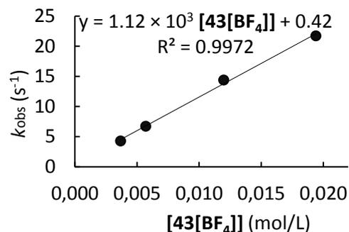
**Table S6.** Kinetics of the reaction of **43[BF<sub>4</sub>]** with **41f** (CH<sub>3</sub>CN, 20°C, stopped-flow, detection at 642 nm)
