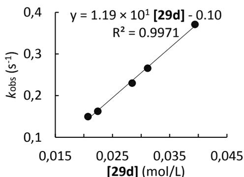
**Table S11.** Kinetics of the reaction of **29d** with **28d** (CH<sub>2</sub>Cl<sub>2</sub>, 20°C, stopped-flow, detection at 611 nm)
