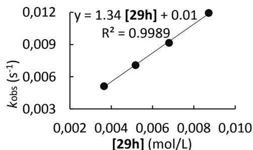
**Table S21.** Kinetics of the reaction of **29h** with **28d** (CH<sub>2</sub>Cl<sub>2</sub>, 20°C, stopped-flow, detection at 611 nm)
