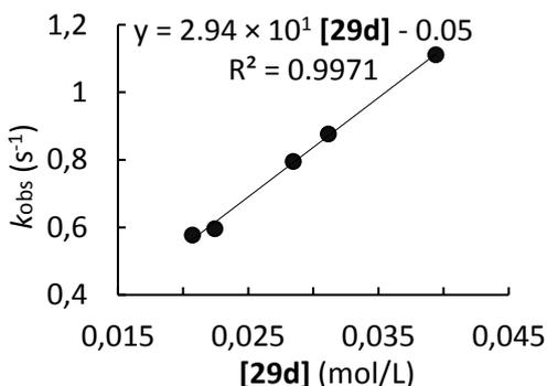
**Table S12.** Kinetics of the reaction of **29d** with **28c** (CH<sub>2</sub>Cl<sub>2</sub>, 20°C, stopped-flow, detection at 671 nm)
