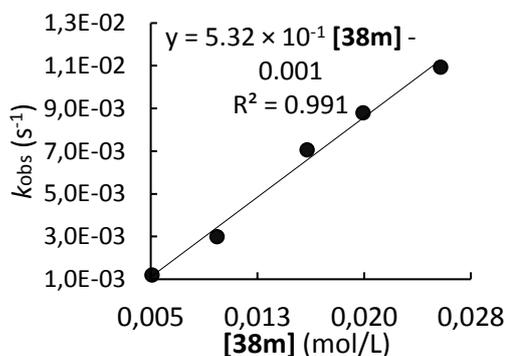
**Table S10.** Kinetics of the reaction of **38m** with **41d** (CH<sub>2</sub>Cl<sub>2</sub>, 20°C, stopped-flow, detection at 621 nm)
