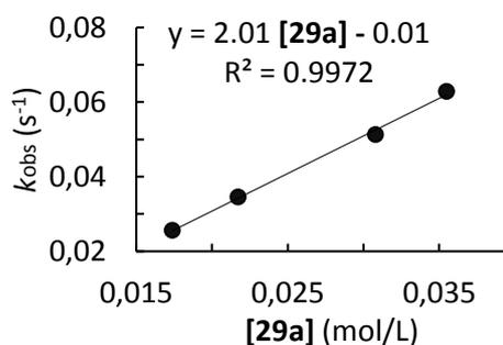
**Table S2.** Kinetics of the reaction of **29a** with **28c** (CH<sub>2</sub>Cl<sub>2</sub>, 20°C, stopped-flow, detection at 671 nm)
