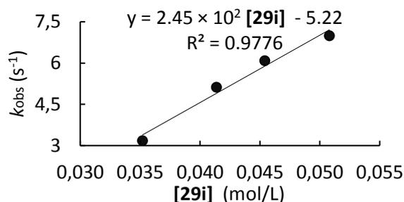
**Table S23.** Kinetics of the reaction of **29i** with **28b** (CH<sub>2</sub>Cl<sub>2</sub>, 20°C, stopped-flow, detection at 586 nm)
