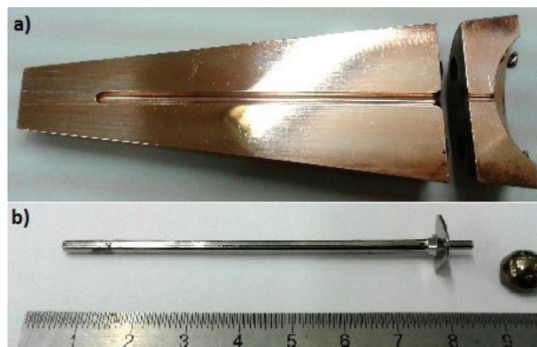
Figure 2.1: a) Half of the copper mold on the left and crucible on the right used for casting 3mm diameter cylinders of bulk metallic glasses. b) The as casted metallic glass rod.
