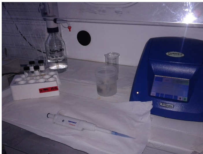
Figure 38 : Fluorimètre Turner Designs Trilogy.
