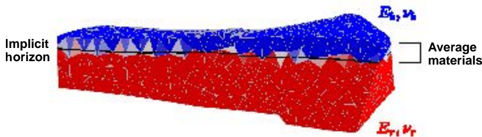
Figure 1.2: Equivalent mechanical properties. Faulted model with an implicit horizon (black thick line). This horizon is the boundary of two layers (red and blue). Average Young's modulus and Poisson's ratio is defined for each tetrahedron crossed by the implicit horizon.
