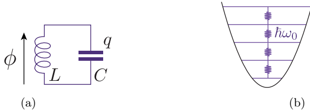
Figure 45: (a) LC resonator equivalent of the microwave cavity mode. \phi is the magnetic flux threading the inductor and q is the charge on the electrode of the capacitor. (b) The energy dispersion of this system is that of a quantum harmonic oscillator.
