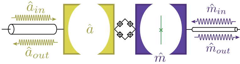
Figure 55: Schematic of the 3D architecture for the quantum node experiment. Transmon qubit shown in green is capacitively coupled to the memory resonator.
