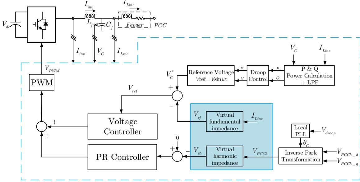
Figure 1.9: Droop Control with enhanced virtual impedance.
