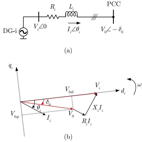
Figure 2.17: Single Line circuit with vector diagram
