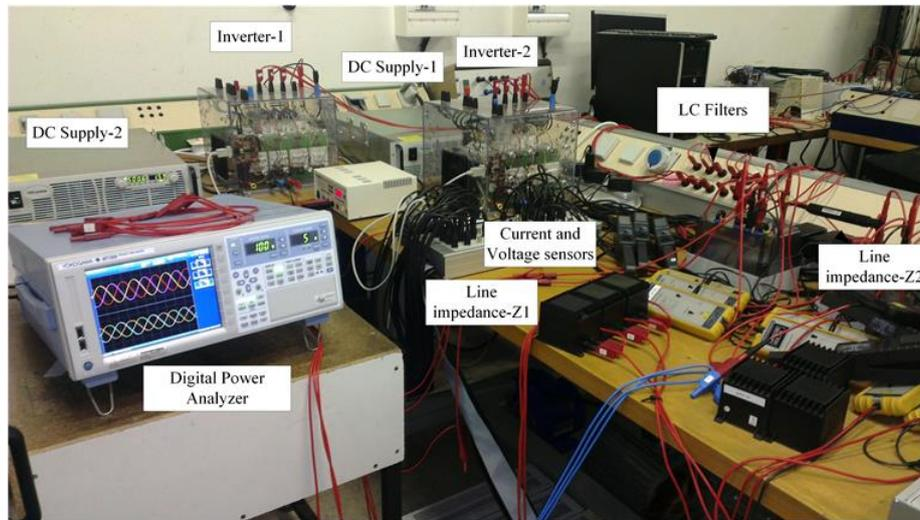
Figure 4.14: Experimental test bench constructed in the Laboratory.
