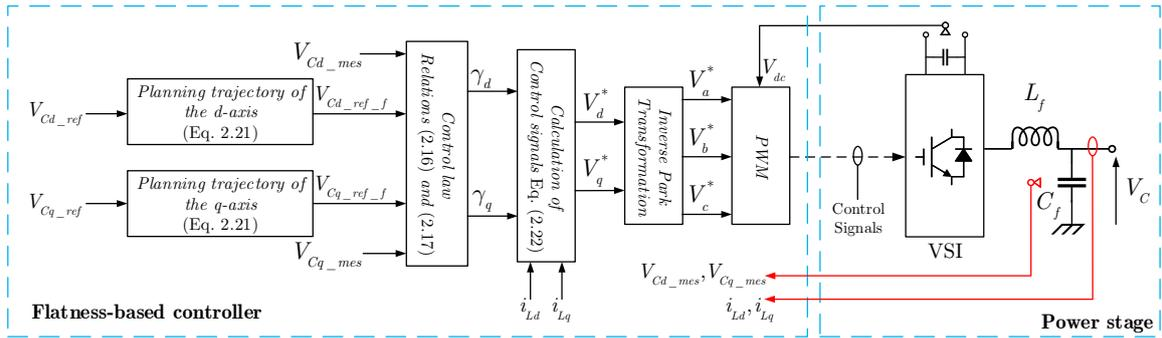
Figure 2.2: Functional diagram of the proposed Control.
