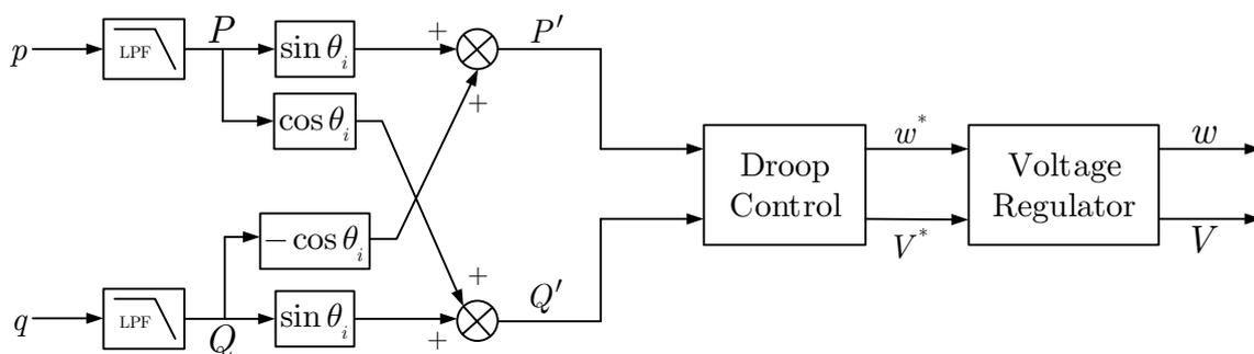
Figure 1.10: Virtual Power Droop Control Block diagram.
