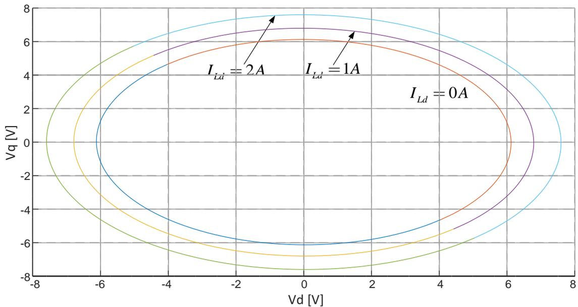
Figure 5.13: Estimated Domain of attraction for the system under the effect of constant current load ( $P_c(\text{CPL}) = 600\text{W}$ ,  $R_{ch} = 100\Omega$ ).
