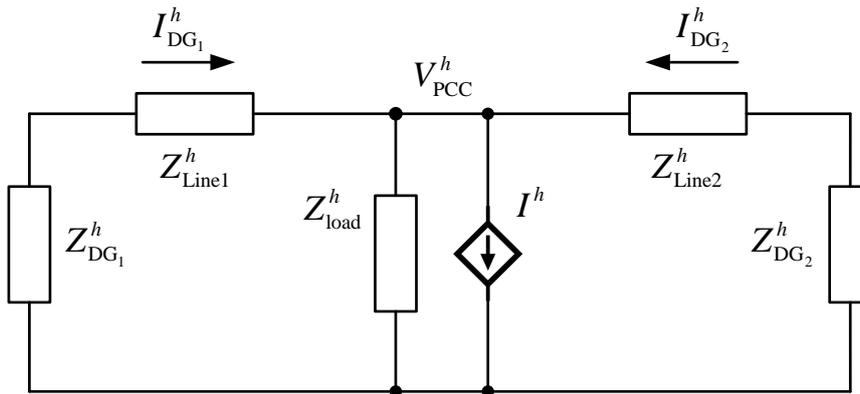
Figure 3.2: Equivalent circuit of two DGs at harmonic frequencies.
