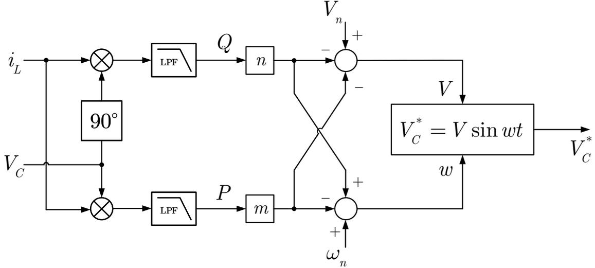
Figure 1.7: Droop Control for complex line impedance.
