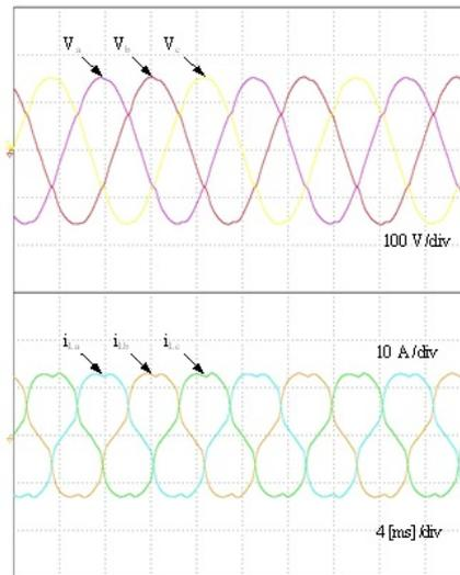
Figure 2.15: Experimental results for output ac voltages and currents with a nonlinear load, ( $V_{dc}=500$  V,  $V_{rms} =110$  V,  $P_{load}=3.2$  kW).
