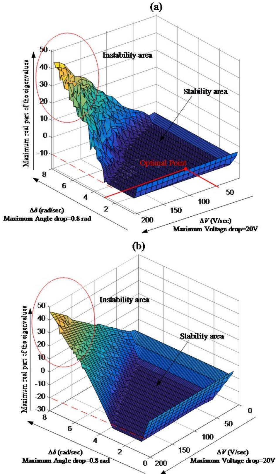
Figure 4.5: Stability margin study by observing the maximum real part of the eigenvalues with respect to the variation of the angle and voltage drop set parameters for: (a)  $K_e = 10\text{sec}^{-1}$ ,  $K_a = 10\text{sec}^{-1}$ ; (b)  $K_e = 20\text{sec}^{-1}$ ,  $K_a = 20\text{sec}^{-1}$ .
