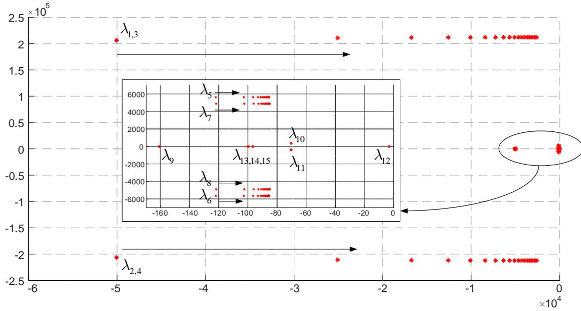
Figure 5.8: Low-frequency eigenvalues as function of  $R_{ch}$  load change (increasing):  $100 \leq R_{ch} \leq 2000$  ( $\Omega$ ).
