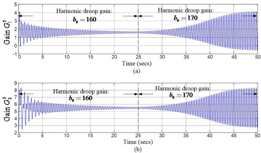
Figure 3.13: Simulation results for system stability: 5th Harmonic gain time response for both DGs.
