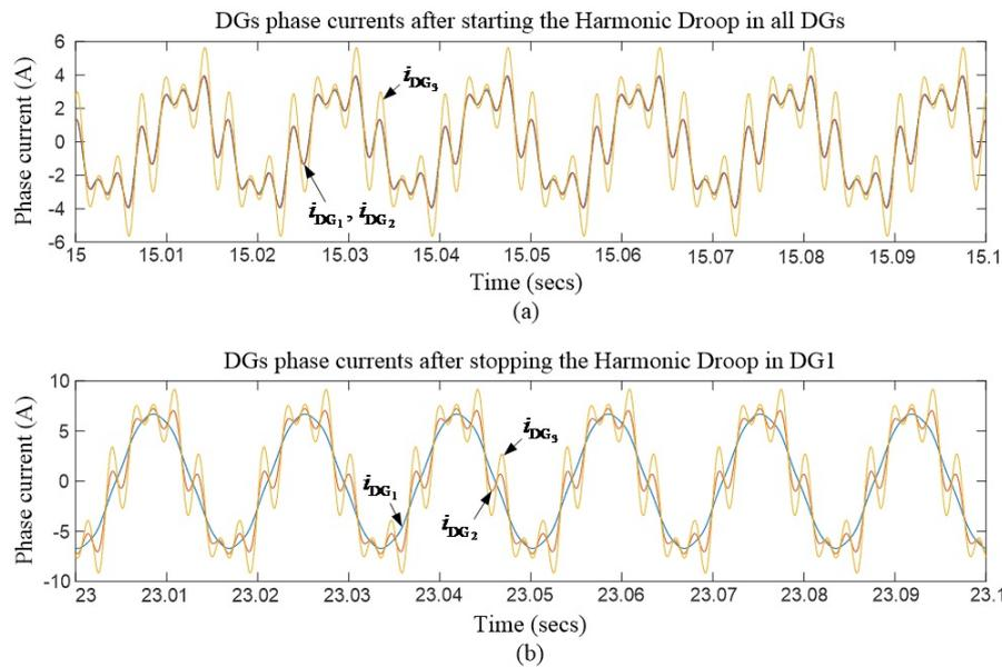
Figure 3.19: Simulation results for microgrid with three DGs: (a) Phase currents before Harmonic compensation:  $i_{DG_1}$ ,  $i_{DG_2}$ , and  $i_{DG_3}$ ; (b) Phase currents after Harmonic compensation.
