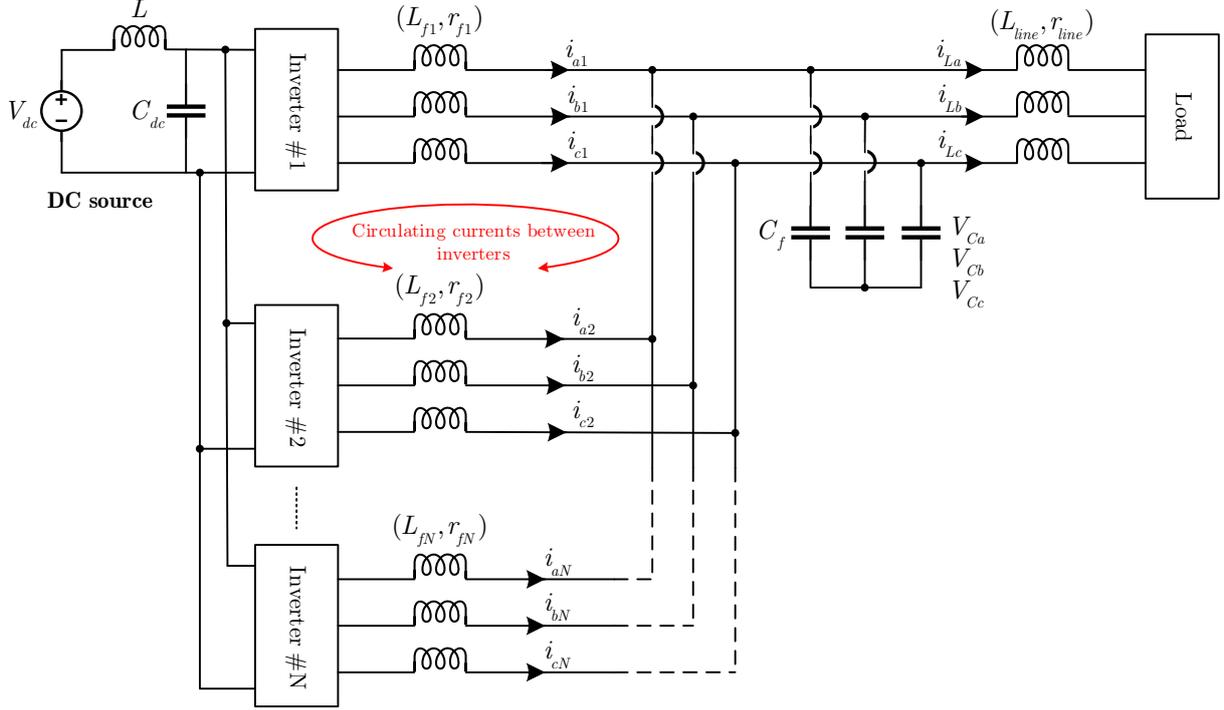
Figure 2.5: System with  $N$ -parallel inverters.
