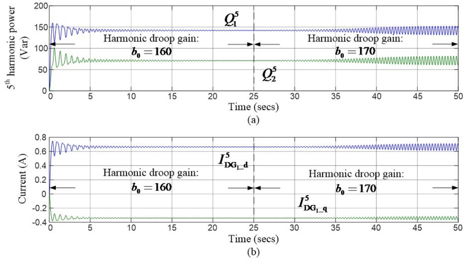
Figure 3.12: Simulation results for system stability: 5th Harmonic power distribution for both DGs with DG<sub>1</sub> harmonic current time response.
