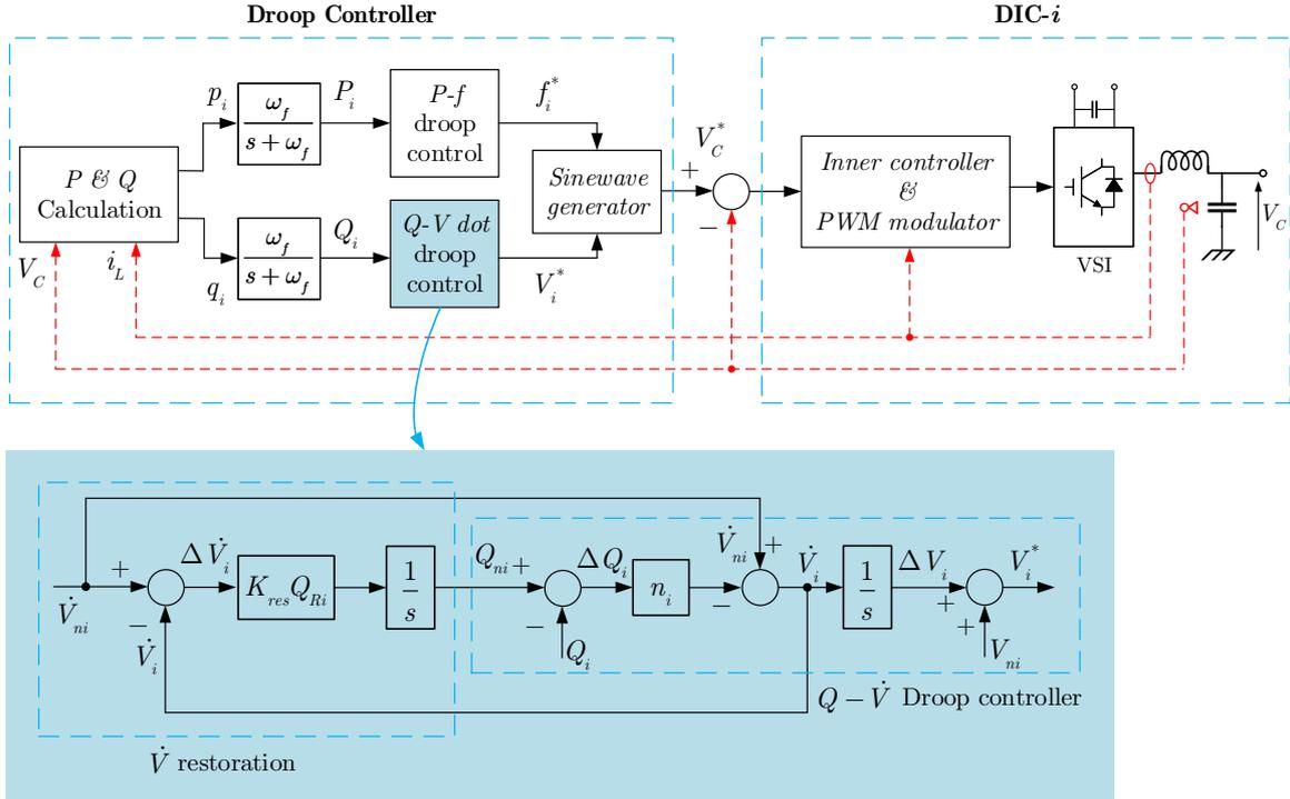
Figure 1.13:  $Q - \dot{V}$  droop Controller and the overall control block diagram of DIC- $i$ .
