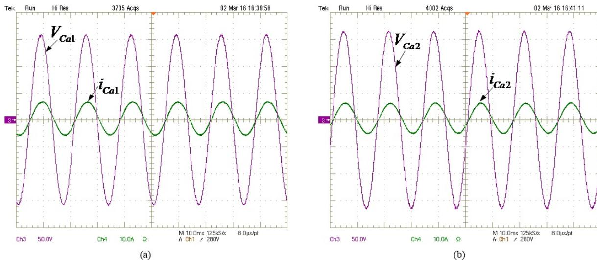
Figure 2.24: Experimental results for Case 1: (a) phase voltage and phase current for DG1; (b) phase voltage and phase current for DG2.
