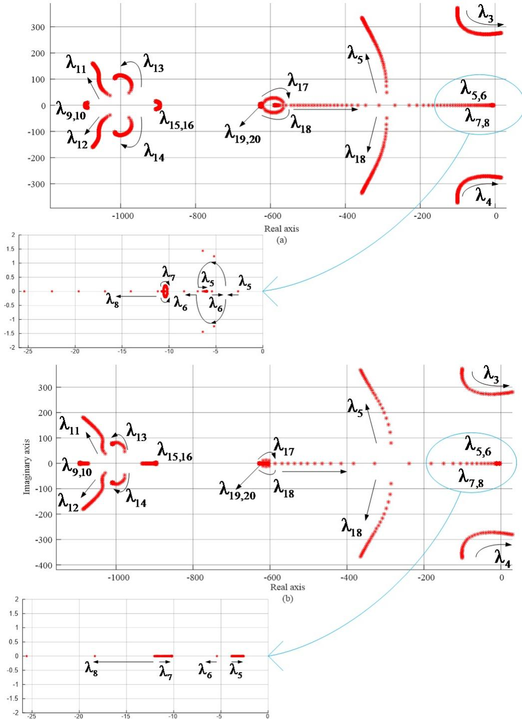
Figure 4.4: Root locus with the variation of parameters in the Droop control: ( $K_e = 10\text{sec}^{-1}$ ,  $K_a = 10\text{sec}^{-1}$ ). (a) Variation of  $m_i$ :  $5 \times 10^{-5} \leq m_1 \leq 5 \times 10^{-3}$  (rad/W.sec),  $1 \times 10^{-4} \leq m_2 \leq 1 \times 10^{-2}$  (rad/W.sec); (b) Variation of  $n_i$ :  $1.33 \times 10^{-2} \leq n_1 \leq 0.53$  (V/Var.sec),  $2.67 \times 10^{-2} \leq n_2 \leq 1.06$  (V/Var.sec).
