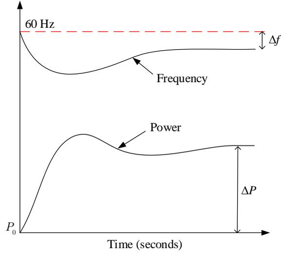
Figure 1.3: Synchronous Generator transient response.
