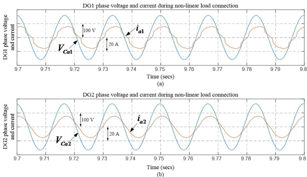
Figure 4.8: Simulation results for Microgrid with two DGs. (a) Phase voltage and current for DG<sub>1</sub>; (b) Phase voltage and current for DG<sub>2</sub>.
