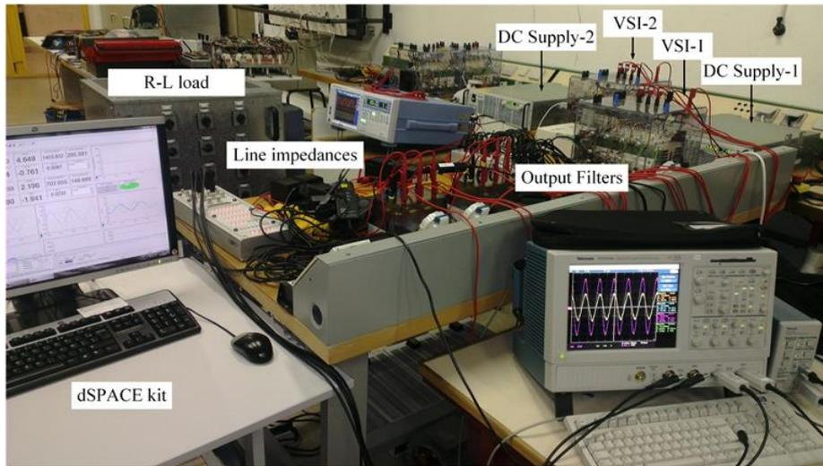
Figure 3.20: Experimental test bench constructed in the laboratory.
