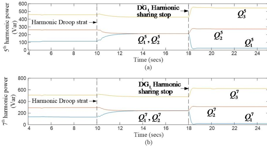
Figure 3.18: Simulation results for microgrid with three DGs with different harmonic ratings: (a) 5th Harmonic power for two DGs:  $Q_1^5$ ,  $Q_2^5$ ,  $Q_3^5$ ; (b) 7th Harmonic power for two DGs:  $Q_1^7$ ,  $Q_2^7$ ,  $Q_3^7$ .
