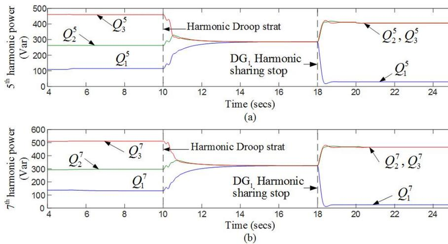
Figure 3.15: Simulation results for microgrid with three DGs with equal harmonic ratings: (a) 5<sup>th</sup> Harmonic power for two DGs:  $Q_1^5$ ,  $Q_2^5$ ,  $Q_3^5$ ; (b) 7<sup>th</sup> Harmonic power for two DGs:  $Q_1^7$ ,  $Q_2^7$ ,  $Q_3^7$ .
