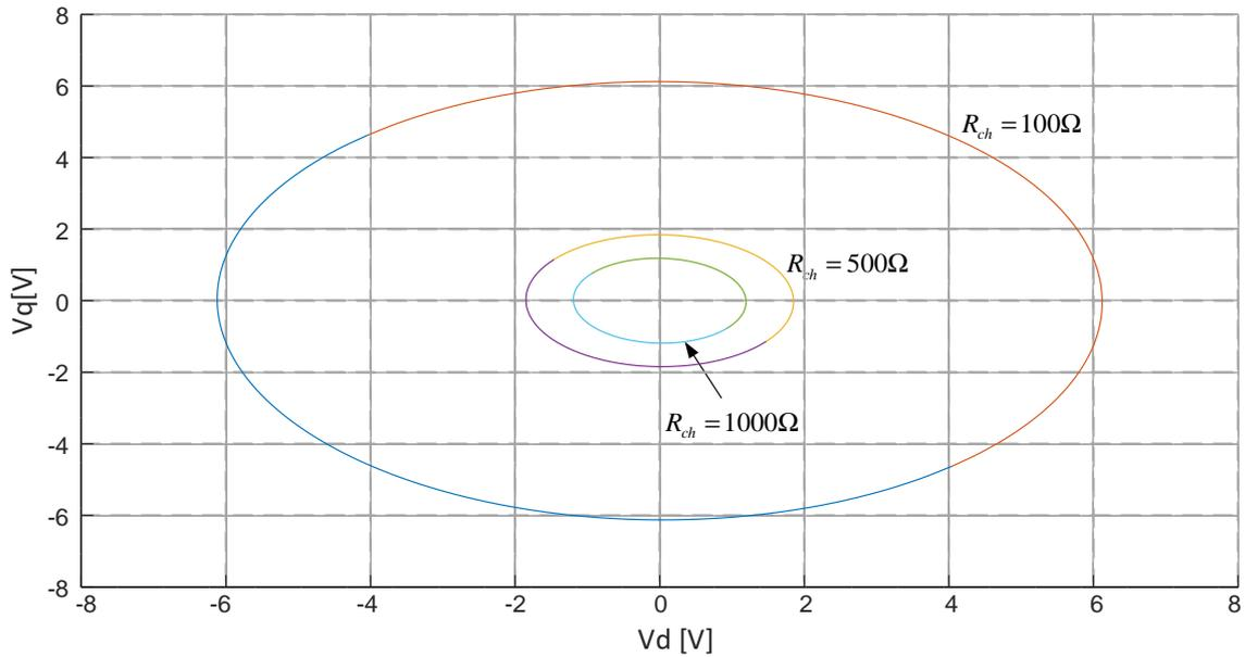
Figure 5.12: Estimated Domain of attraction for the system under the effect of Resistive Load,  $R_{ch}$  ( $P_c(\text{CPL}) = 600\text{W}$ ,  $I_{Ld} = 0$ ,  $I_{Lq} = -3\text{A}$ ).
