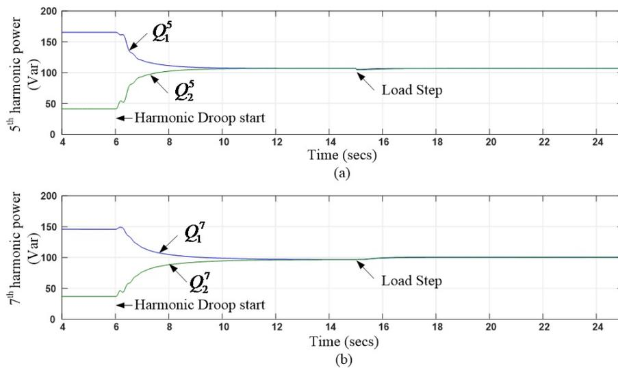
Figure 3.9: Simulation results for case 1. (a) 5<sup>th</sup> Harmonic power for two DGs:  $Q_1^5$ ,  $Q_2^5$ ; (b) 7<sup>th</sup> Harmonic power for two DGs:  $Q_1^7$ ,  $Q_2^7$ .
