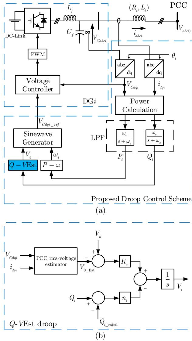
Figure 2.18: Proposed Droop Control scheme with modified  $Q - V_{Est}$  Droop.
