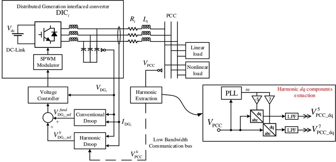
Figure 3.4: Proposed control strategy for DG interfaced converter.
