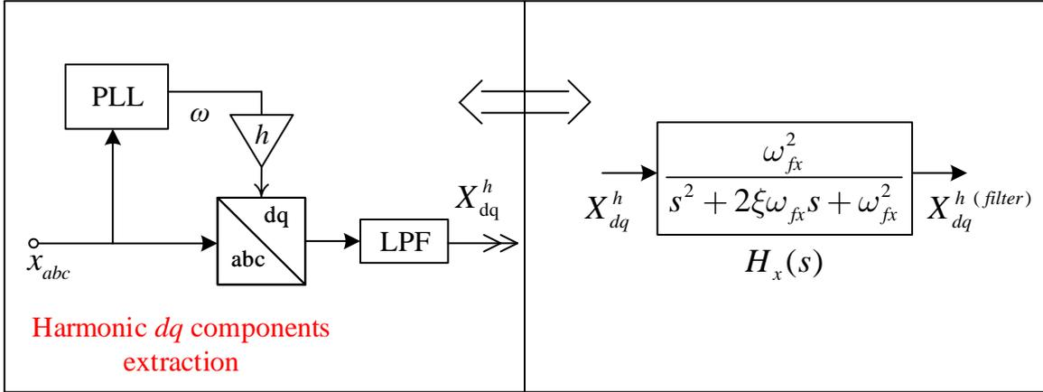
Figure 3.6: Synchronous individual harmonic “*dq* frame” extraction block.
