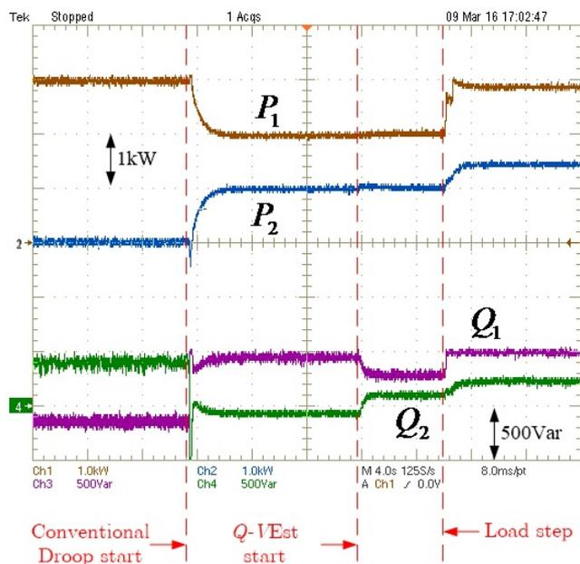
Figure 2.25: Experimental results for Case 2: Fundamental Real power:  $P_1$ ,  $P_2$ ; Fundamental Reactive power:  $Q_1$ ,  $Q_2$  before and after the intervention of the estimated PCC rms-voltage.
