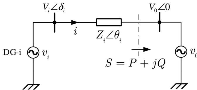
Figure 1.4: Distributed Generator Delivering power to infinite bus through impedance  $\bar{Z}_i$ .
