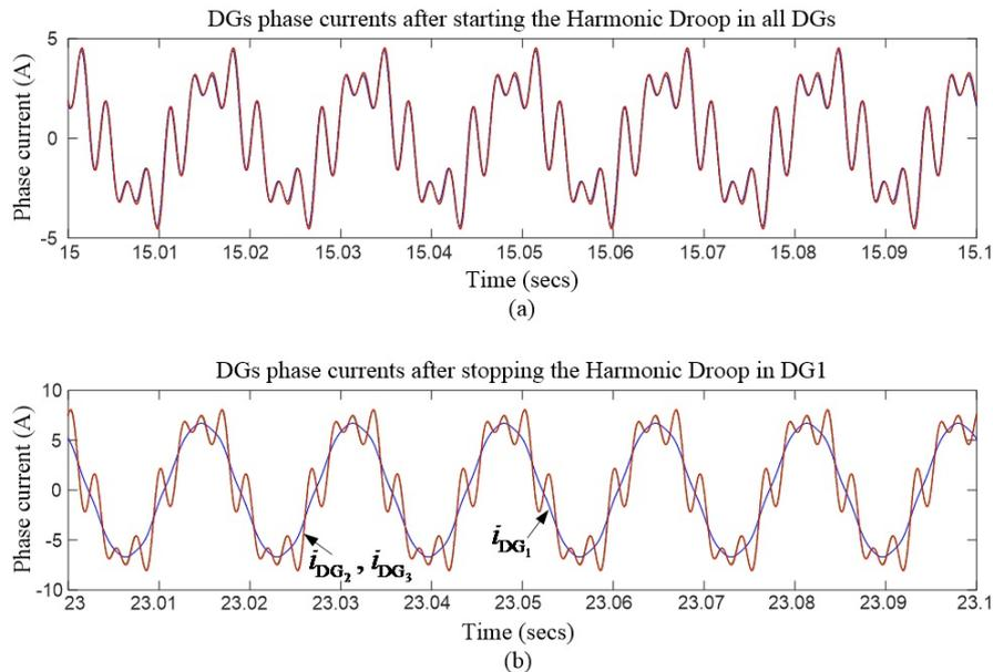
Figure 3.16: Simulation results for microgrid with three DGs: (a) Phase currents before Harmonic compensation:  $i_{DG_1}$ ,  $i_{DG_2}$ , and  $i_{DG_3}$ ; (b) Phase currents after Harmonic compensation.
