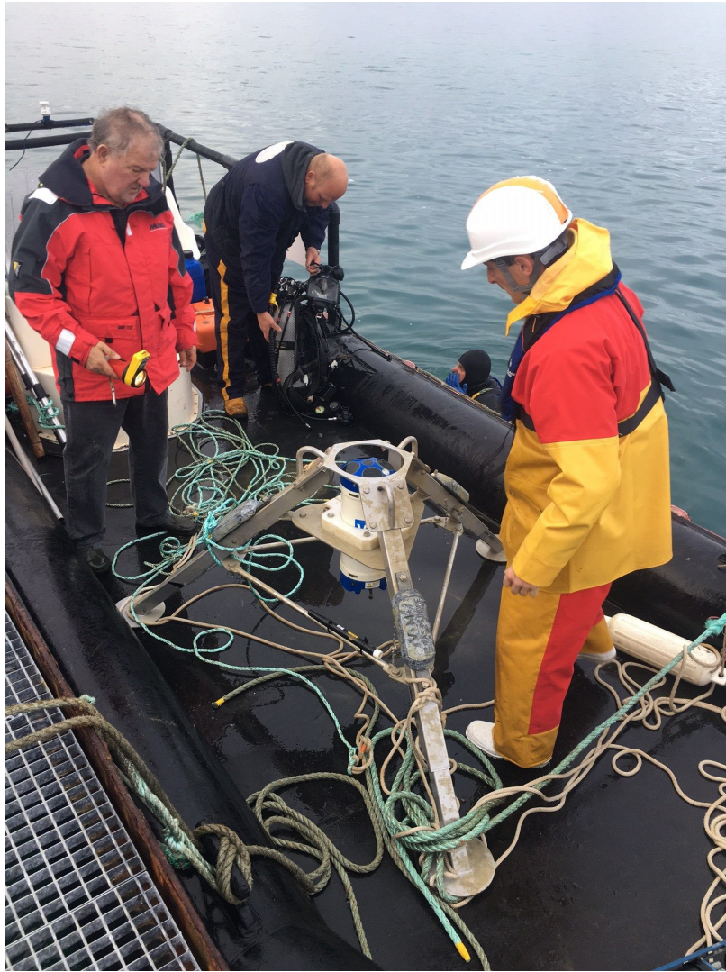
Figure 4.13: An ADCP fixed on its tripod during the measurements campaign (October 2016).
