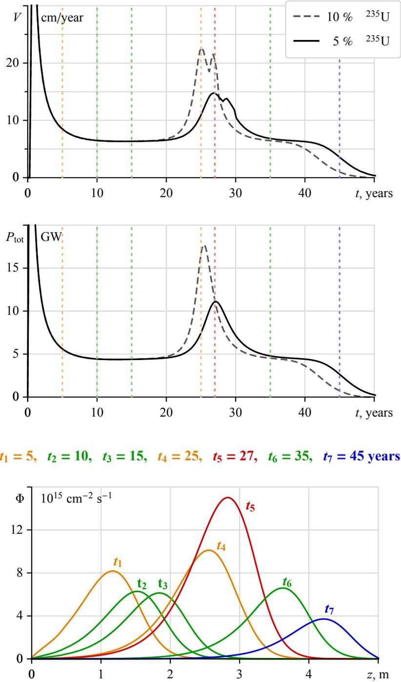
Figure 10.1: The NBW FR behavior in the case of presence of a uranium layer enriched with 5% (solid curves) and 10% (dashed curves)  $^{235}\text{U}$  at  $z = 3.0\text{--}3.2$  m: the axial distributions of the scalar neutron flux  $\Phi(z)$  for different time moments  $t_i$ ; the NBW velocity  $V(t)$  and the total FR power  $P_{\text{tot}}(t)$  as a functions of time.
