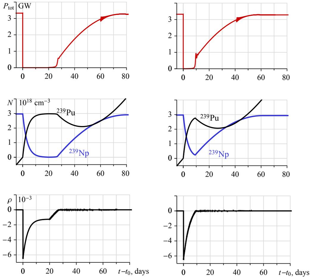
Figure 11.10: Evolution of the reactor power  $P_{\text{tot}}(t)$ , average over the FR volume concentrations  $N$  of  $^{239}\text{Np}$  and  $^{239}\text{Pu}$  and reactivity  $\rho(t)$  at restarting of the FR after its shutdown ( $t = t_0$ ) in 20 days (left plots) and in one day (right plots). Concentration of  $^{239}\text{Pu}$  is relative to  $t = t_0$ :  $N_{\text{Pu}}(t) - N_{\text{Pu}}(t_0)$ .
