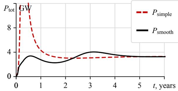
Figure 11.5: Total energy production power as a function of time for the FR variants with the simplified  $P_{\text{simple}}(t)$  (dashes) and the improved smooth  $P_{\text{smooth}}(t)$  (solid lines) start-up schemes, whose critical configurations are shown in Fig. 11.1 and in Fig. 11.4 correspondingly.
