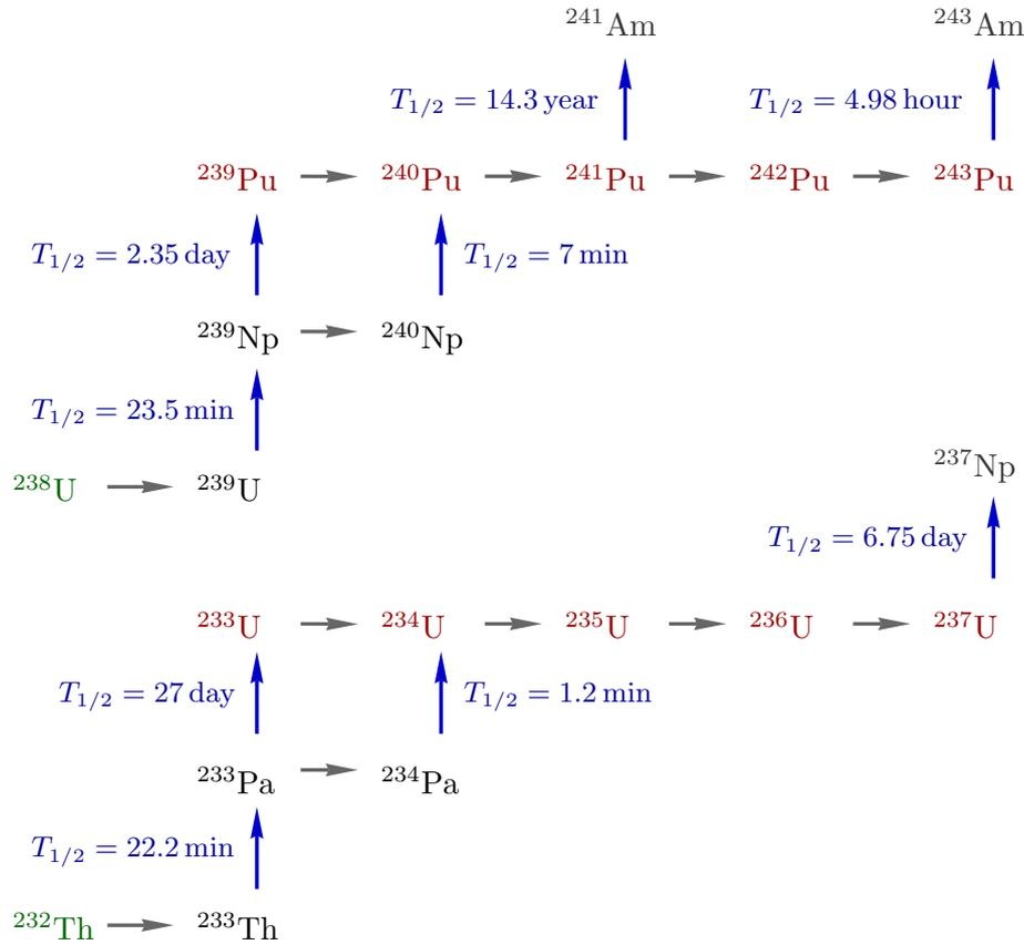
Figure 8.2: Scheme of the nuclear transformations starting from the basic isotope  $^{238}\text{U}$  (on top) and  $^{232}\text{Th}$  (at the bottom) under neutron irradiation. The horizontal arrows correspond to the  $(n, \gamma)$  reaction, and the vertical arrow corresponds to the  $\beta$ -decay of the nuclide with the half-period  $T_{1/2}$ .
