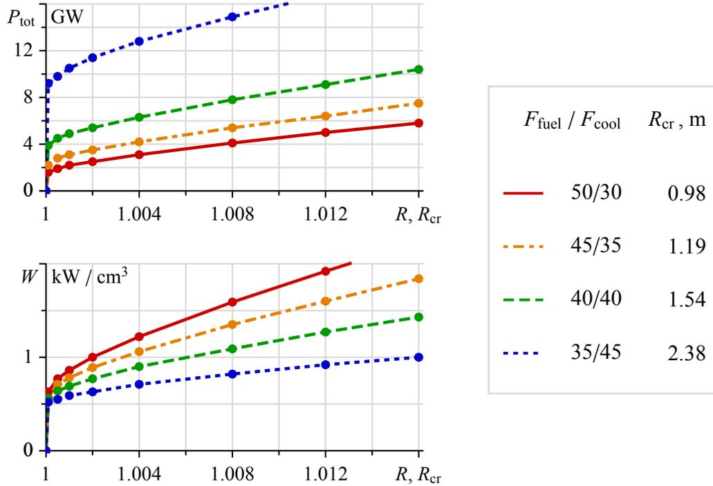
Figure 9.1: Total power production  $P_{\text{tot}}$  (upper plot) and density of power production  $W$  (bottom plot) as a function of cylinder radius  $R$  of FR for four variants of reactor composition  $F_{\text{fuel}} / F_{\text{cool}}$ , listed on the right together with the values of corresponding critical radii  $R_{\text{cr}}$ .
