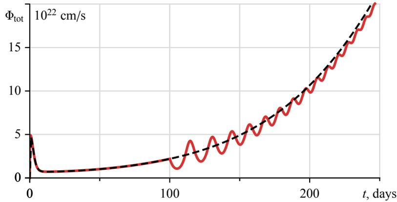
Figure 9.3: The integral neutron flux as a function of time  $\Phi_{\text{tot}}(t)$  at the initial stage of FR operation when the external neutron flux is turned off at  $t_{\text{off}} = 100$  days (solid red curve) and without switching off the external flux (dashed black curve).
