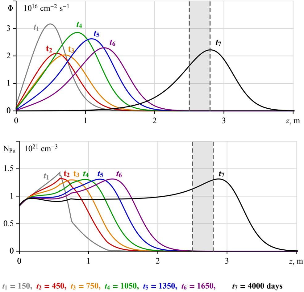
Figure 11.7: Evolution of axial profiles in the FR with the optimized ignition zone shown in Fig. 11.4 for the neutron flux  $\Phi(z)$  and the  $^{239}\text{Pu}$  concentration  $N_{\text{Pu}}$  at different time moments  $t_i$ .
