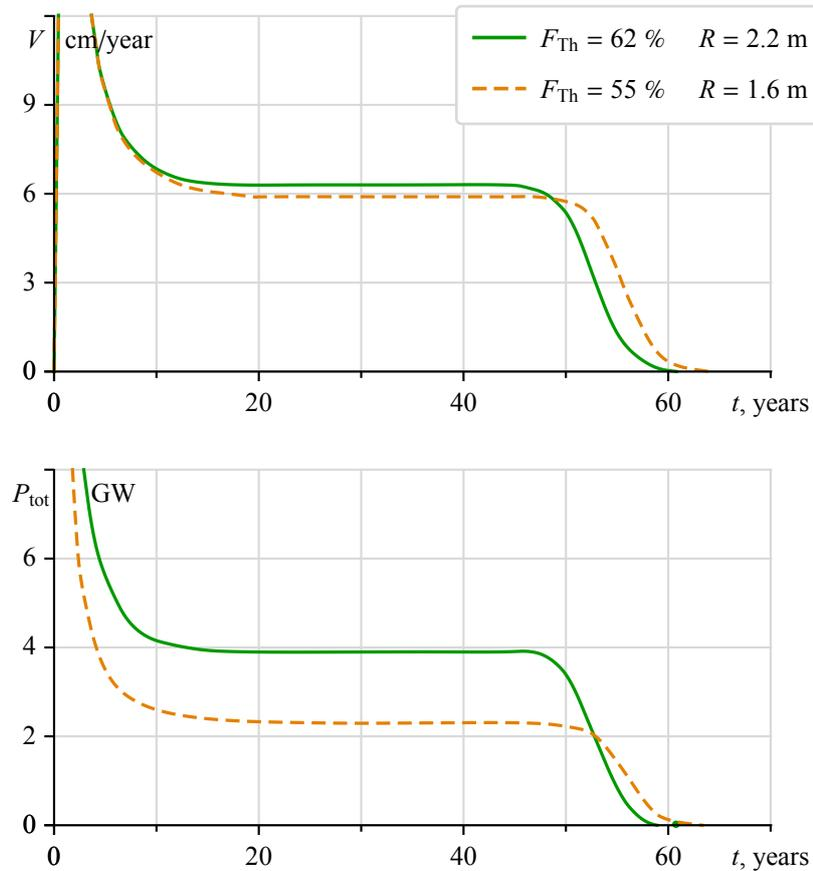
Figure 9.9: The NBW velocity  $V(t)$  and the total FR power  $P_{tot}(t)$  as a function of time; the axial distributions of the neutron fluence  $F(z)$  for the whole reactor campaign for two different fuel compositions: volume fraction of Th in the fuel  $F_{Th} = 62\%$  ( $R = 2.2$  m) and  $F_{Th} = 55\%$  ( $R = 1.7$  m).
