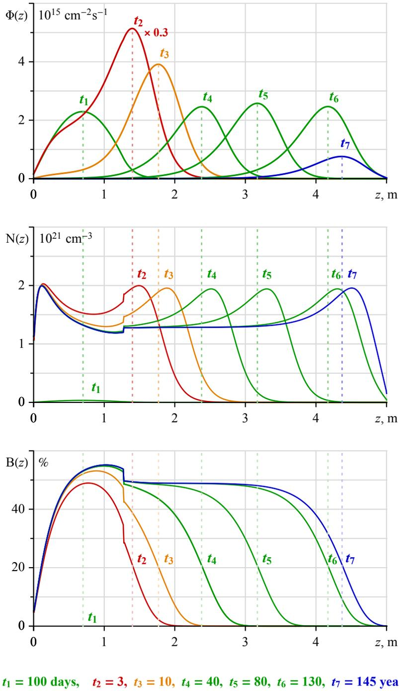
Figure 9.2: The NBW profiles in a hypothetical FR consisting only of metallic Th-U fuel: a scalar neutron flux  $\Phi(z)$ , concentration  $N(z)$  of  $^{233}\text{U}$  and the fuel burn-up depth  $B(z)$ , along the longitudinal coordinate of the reactor for different time moments listed at the bottom.
