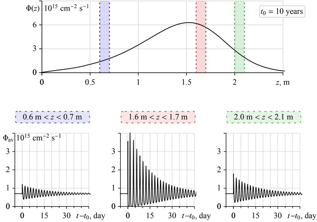
Figure 10.2: The perturbation of volume-average neutron flux  $\Phi_{av}(t)$  in the NBW FR caused by an external neutron source versus time. The source with intensity  $Q_{ex} = 2 \times 10^{11} \text{ cm}^{-3} \text{ s}^{-1}$  starts at  $t_0 = 10$  years, lasts for one hour and is situated at  $(0.6 \text{ m} < z < 0.7 \text{ m})$  or  $(1.6 \text{ m} < z < 1.7 \text{ m})$  or  $(2.0 \text{ m} < z < 2.1 \text{ m})$ .
