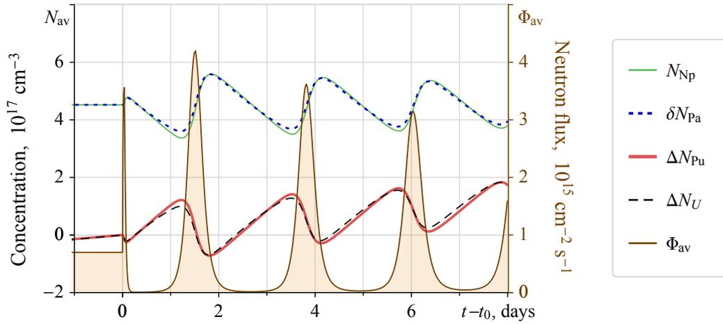
Figure 10.3: Evolution of the volume-averaged neutron flux  $\Phi_{\text{av}}(t)$  and concentrations  $N_{\text{av}}(t)$  of the main fissile and intermediate nuclides in the fuel of mixed Th–U–Pu cycle with time. First three oscillations from Fig 10.2 for the case ( $1.6 \text{ m} < z < 1.7 \text{ m}$ ).
