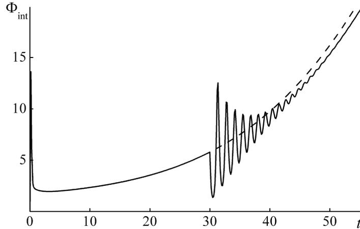
Figure 9.8: The integral neutron flux  $\Phi_{\text{int}}$  ( $10^{22}$  cm/s) as a function of time  $t$  (days) at the initial stage of the reactor campaign for  $t_{\text{off}} = 30$  days (solid line) and  $t_{\text{off}} = 100$  days (dashed line). Here  $F_{\text{Th}} = 62\%$  and  $R = 2.3$  m.
