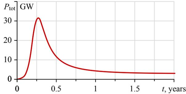
Figure 11.2: Total energy production power  $P_{\text{tot}}(t)$  as a function of time for the FR variant with a simplified start-up critical configurations (see Fig. 11.1).
