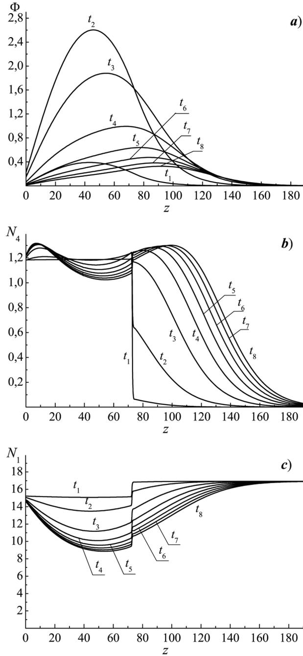
Figure 11.3: Initial evolution of axial profiles ( $z$  in cm) near the ignition zone (a) for the neutron flux  $\Phi$  ( $\times 10^{17} \text{ cm}^{-2} \text{ s}^{-1}$ ) and the (b)  $^{239}\text{Pu}$  and (c)  $^{238}\text{U}$  concentrations  $N_4$  and  $N_1$  ( $10^{21} \text{ cm}^{-3}$ ) for the FR with simplified start-up scheme at the time moments  $t_1 = 40$ ,  $t_2 = 80$ ,  $t_3 = 120$ ,  $t_4 = 160$ ,  $t_5 = 200$ ,  $t_6 = 240$ ,  $t_7 = 280$  and  $t_8 = 320$  days.
