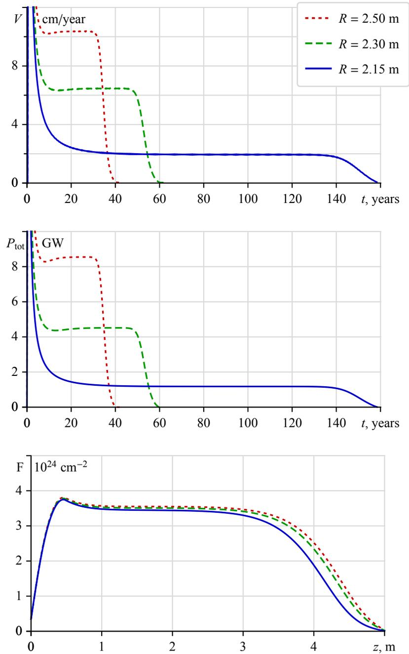
Figure 9.6: The NBW velocity  $V(t)$  and the total FR power  $P_{\text{tot}}(t)$  as a function of time; the axial distributions of the neutron fluence  $F(z)$  for the whole reactor campaign for different reactor radii listed on the right. Here  $F_{\text{Th}} = 62\%$ .
