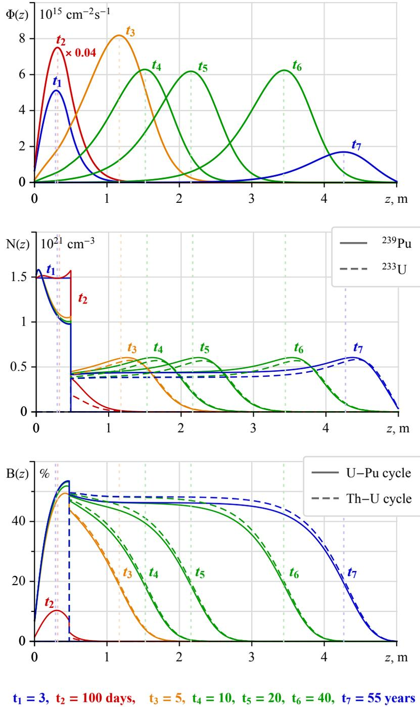
Figure 9.5: The axial distributions of the NBW characteristics: the scalar neutron flux  $\Phi(z)$ ; the concentration of main fissile isotope  $N(z)$ ; the fuel burn-up depth of the fuel components  $B(z)$ , at different time moments listed at the bottom. Here  $F_{Th} = 62\%$  and  $R = 2.3$  m.
