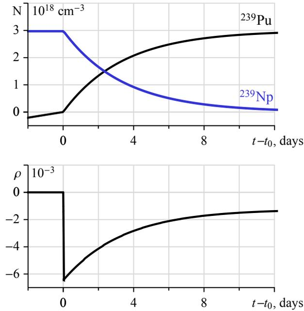
Figure 11.9: Evolution of the average over FR volume concentrations  $N(t)$  for  $^{239}\text{Np}$  and  $^{239}\text{Pu}$  isotope and the FR reactivity  $\rho(t)$  at its shutdown ( $t = t_0$ ). Concentration of  $^{239}\text{Pu}$  is relative to  $t = t_0$ :  $N_{\text{Pu}}(t) - N_{\text{Pu}}(t_0)$ .
