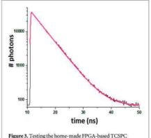
acquisition system. Monoexponential fluorescence decay (semilog plot) of fluorescence in PBS solution measured, with the FPGA-based TDC, in a conventional 1 mm thick quartz cuvette standing in place of the microfluidic chip in the experimental set-up described above.
