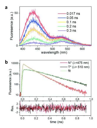
**Figure 3: TRF spectroscopy of compound 1 in MeOH. a.** Fluorescence spectra at a selection of time delays after pulsed laser excitation at 343 nm. Solid thick lines result from numerically smoothing the raw data (thin lines) **b.** Decay kinetics of the N\* (in red) and T\* (in black) bands integrated over the  $\lambda$ <475 nm and  $\lambda$ >510 nm spectral windows, respectively. Both curves are fitted globally (green lines) and the weighted residuals are displayed below.
