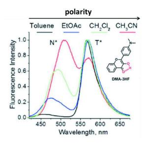
Figure 3-Adopted from<sup>57,58</sup>. 4'-dialkylamino-3-hydroxyflavone dye undergoes ESIPT and exhibits solvent-dependent dual emission.
