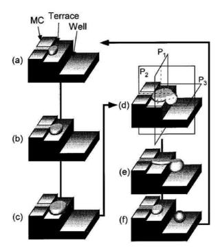
Figure 15- Adapted from <sup>175</sup>. Schematic illustration of the droplet-formation mechanism caused by interfacial tension. Dispersed phase passed through the micro-fabricated channel inflated on the terrace in a disk-like shape (a-c). The dispersed phase flowed into the well and transformed into a spherical droplet (d-f).
