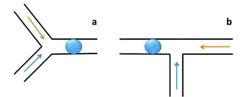
Figure 16-Schematic illustration of a.Y-junction and b. T-junction geometries for droplet formation in different droplet microfluidics chip geometry. In yellow arrow is the oil and in blue the liquid compound.
