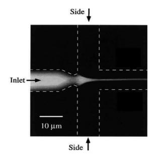
Figure 14-Adapted from<sup>158</sup>. Hydrodynamic focusing region, where two side channels press the stream of the inlet channel and due to simultaneous diffusion across the same stream fast mixing is achieved.
