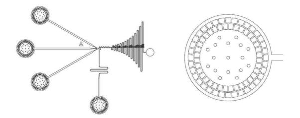
Figure 20-a. Overview of a device drawing (AutoCAD). The three input channels for aqueous solutions are presented on the left and the one for oil is located at the bottom. b. Zoom on an input, where a filter is used composed of blocks spaced less than the width of the channels in order to avoid blocking.
