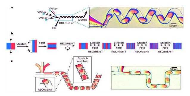
Figure 18-a. Droplet mixing. Arrow color corresponds to dye in stream solution. Dashed line in image indicates merging of the streams. b. Schema of a fluid element undergoing stretching, folding and reorientation. c. Microphotographs of a microfluidic network in which flow patterns inside plugs in the microchannel demonstrate flow folding and stretching pattern. Figure from <sup>166</sup>.
