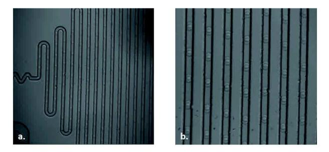
Figure 22-Droplets flowing in a  $50x50\mu m$  channel with speed 50 mm/s between light pulses separated by 0.5 ms a. full picture b. zoom.
