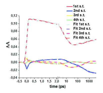
Figure 28-The 4 first singular kinetic traces were fitted globally. Data acquired for 4-Methoxy-3-Hydroxyfavone in DMF solvent.
