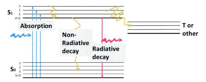
Figure 5-Schematic illustration of radiative and non-radiative de-excitation processes.
