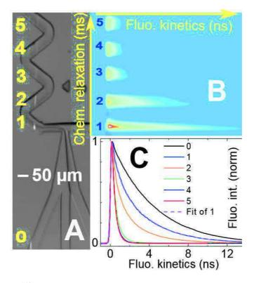
Figure 38-Adapted from<sup>148</sup>. Mixing time measurements A) Microfluidic chip illuminated by the excitation line. The intersection regions of the excitation line with the microfluidic channel are labeled 0 to 5. B) 2D streak camera data: several fluorescence kinetic traces are acquired simultaneously along the propagation in the channel. C) Fluorescence kinetic traces at each of the five positions in the microfluidic chip.
