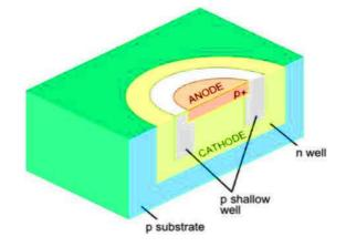
Figure 49-From<sup>387</sup>, SPAD cross section.
