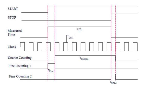
Figure 50-Operation principle of a TDC<sup>393</sup>.
