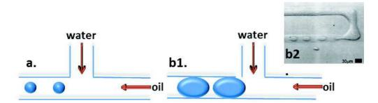
Figure 17-Sketch of a microfluidic T-junction used to create a. water droplets and b1 plugs in oil (b2 photograph of the discontinuous water phase introduced into the continuous oil phase<sup>177</sup>). Water stream comes from the vertical direction meeting the perpendicular flow from the oil channel. The channel dimensions are typically on the order of 50-100  $\mu$ m.
