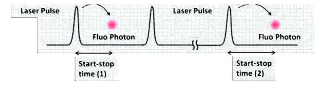
Figure 8-Schematic illustration of the TCSPC technique, where the start signal corresponds to the excitation laser pulse and the stop to the single photon detection.
