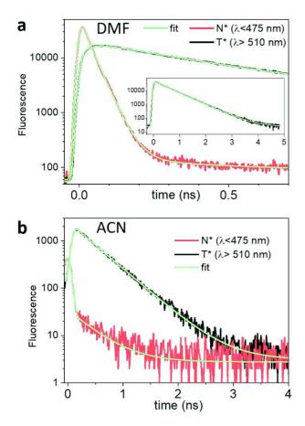
Figure 4: TRF spectroscopy of compound 1 in a. DMF and b. ACN. Decay kinetics of the N\* (in red) and T\* (in black) bands are integrated over the  $\lambda$ <475 nm and  $\lambda$ >510 nm spectral windows, respectively. For each panel, both curves are fitted simultaneously (green lines).
