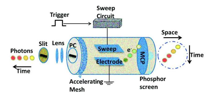
Figure 7-Schematic illustration of operating principle of streak tube.
