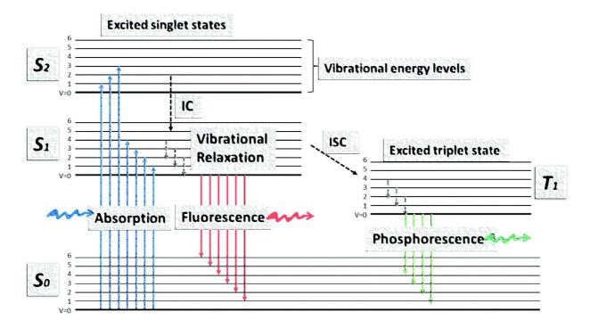
Figure 1-Jablonski energy diagram depicting the transition between electronic states of a molecule. Dashed lines indicate non-radiative transitions, IC stands for internal conversion, ISC stands for intersystem crossing. All of these transitions will be explained in the following parts.
