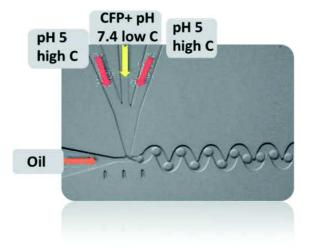
Figure 37-Microfluidic chip-Photograph of the mixing region (T-junction) of a microfluidic chip.
