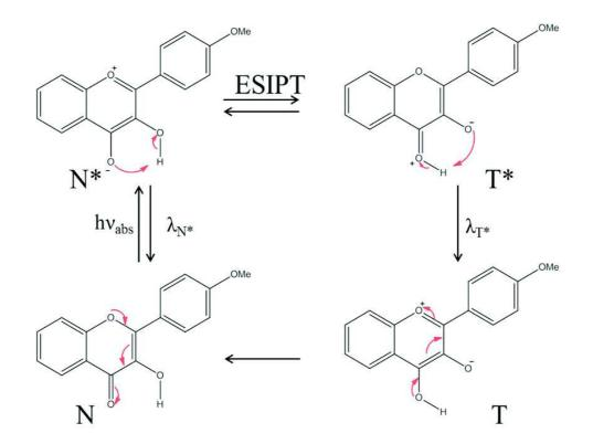
Figure 24-Schematic illustration of ESIPT reaction in 4M3HF.
