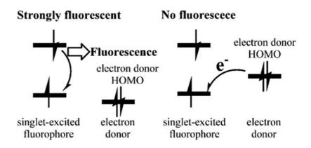
Figure 4-adopted from<sup>64</sup>. On the left, the HOMO (highest occupied molecular orbital) energy level of the electron donor moiety is too low to allow electron transfer. Consequently, emission from the singlet-excited fluorophore is not affected. On the right, the HOMO energy level is high enough to allow electron transfer, thus the fluorescence decreases.
