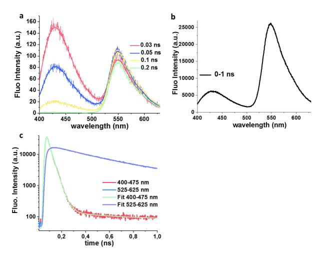
Figure 26-TRF Spectroscopy of 4M3HF in DMF. a. Fluorescence spectra of selected time delays after laser pulse excitation at 343nm.b. Same as above integrated of the full recorded spectrum. c. Decay kinetics of the N\* (in red) and T\* (in black) bands integrated over the  $\lambda$ <475 nm and  $\lambda$ >525 nm spectral windows, respectively. Both curves are fitted globally.
