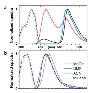
**Figure 2.** Steady-state absorption (dashed lines) and emission (full lines) spectra of **a**. compound **1** and **b**. compound **2** for which no ESIPT reaction is possible, in MeOH (red), DMF (black), ACN (green) and toluene (blue).
