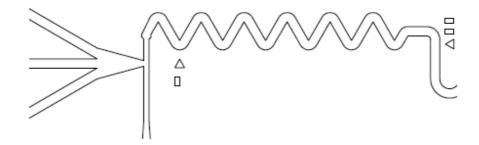
Figure 21-Photograph of the mixing region in one of our microfluidic chips.
