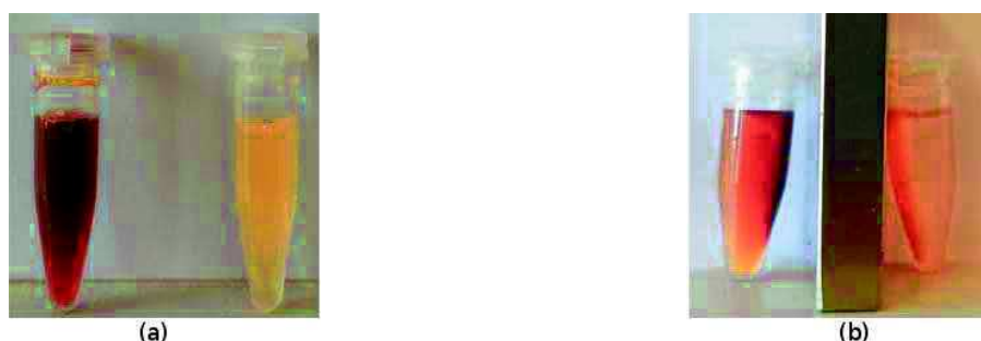
Figure 15. Optical micrographs of the two SPIONS-loaded PMMA NPs suspensions obtained with the nanoprecipitation (right) and nanoemulsification (left) methods without magnetic field (a) and in presence of a simple magnet (b).
