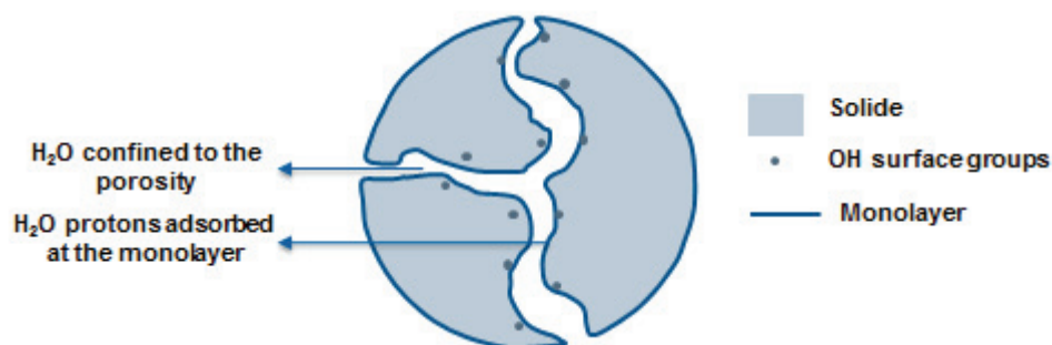
Figure 53 – Different types of \text{H}_2\text{O} protons present in the alumina support (adapted from [160])
