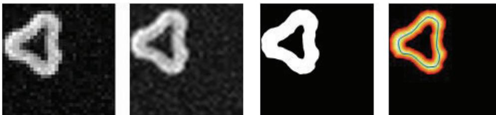
**Figure 52** – Example of processing and analysis of MRI image. From left to right : initial image (resolution  $47 \mu\text{m} \times 47 \mu\text{m}$ ), increase of resolution by numerical interpolation (resolution  $14 \mu\text{m} \times 14 \mu\text{m}$ ), automatic segmentation, distance function calculation (red to yellow colors) and medial axis extraction (blue color)
