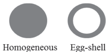
Figure 2 – Metal profile: homogeneous and eggshell distributions (where the shaded area represents the metal) [9]
