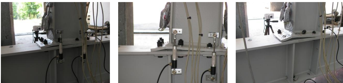
Figure 5.6 Deformation of connection elements during experimental testing
