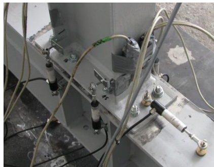
Figure 6.2 End plate connection with extended end plate
