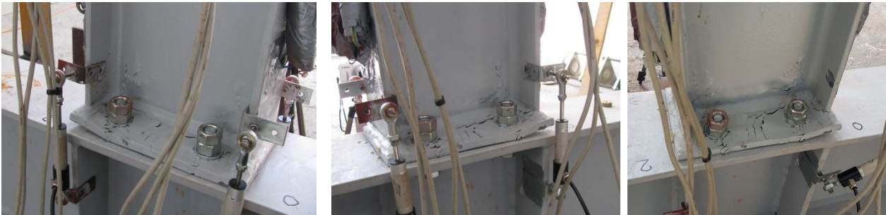
Figure 6.7 Deformation of connection elements during experimental testing
