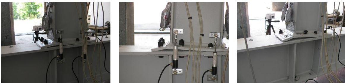
Figure 5.6 Deformation of connection elements during experimental testing
