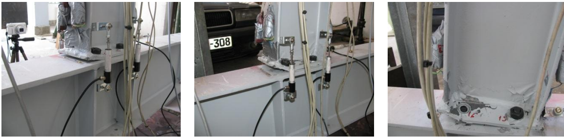
Figure 5.10 Deformation of connection elements during the experimental testing
