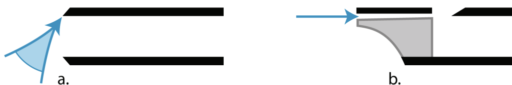
Fig. 1. Blowing angle variations regarding two different organological kinds of flutes: (a) oblique flute, (b) duct-flute
