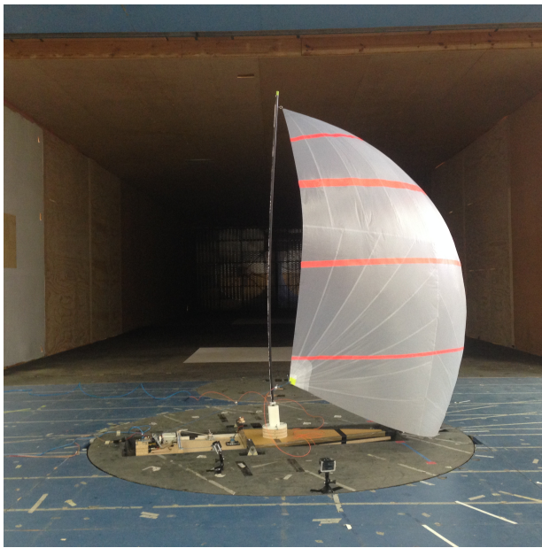
(a) Free mast configuration. The mast is cantilevered at the step and unstayed. Important mast bending can be observed (2015).
