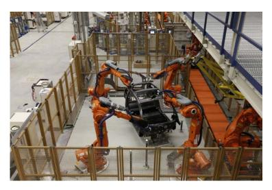
Figure 2.1 – An example of four robots working together, in an automotive factory, on the same car. The robots are fulfilling different tasks and they have a really limited awareness of other robots and of their environment (from which they are separated through a cage).
