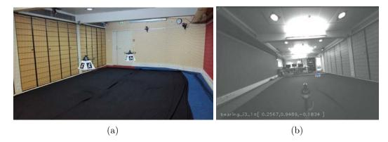
Figure 8.1 – First tests with the AprilTag fiducial markers. Fig. 8.1(a): two quadrotor UAVs flying in our flying arena with some Apriltag [197] mounted on them. Note that we plan to reduce the size of the fiducial markers used in our applications to make them more compact and easy to embed on each UAV. Fig. 8.1(b): a snapshot of an onboard camera which shows the detection of an AprilTag fiducial marker mounted on another quadrotor UAV and the consequent translation to a bearing vector.
