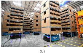
Figure 2.3 – Multiple robots moving shelves around a warehouse at Amazon (Fig. 2.3(a)) and Alibaba<sup>5</sup>(Fig. 2.3(b)).
