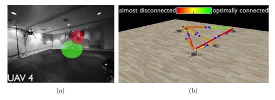
Figure 6.4 – Fig. 6.4(a) highlights why the *occluded visibility* constraint is needed. Indeed, it is possible to notice how the visibility of the robot in red, with respect to the *observing* robot, is being occluded by the robot in green. As usual, Fig. 6.4(b) is the graph view corresponding to the case of Fig. 6.4(a).
