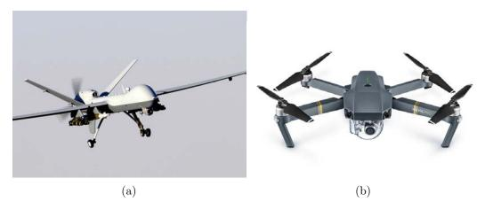
Figure 2.6 – Examples of fixed and rotary wing UAVs. Fig. 2.6(a): the MQ-9 Reaper, from General Atomics. Fig. 2.6(b): the Mavic Pro, from DJI.
