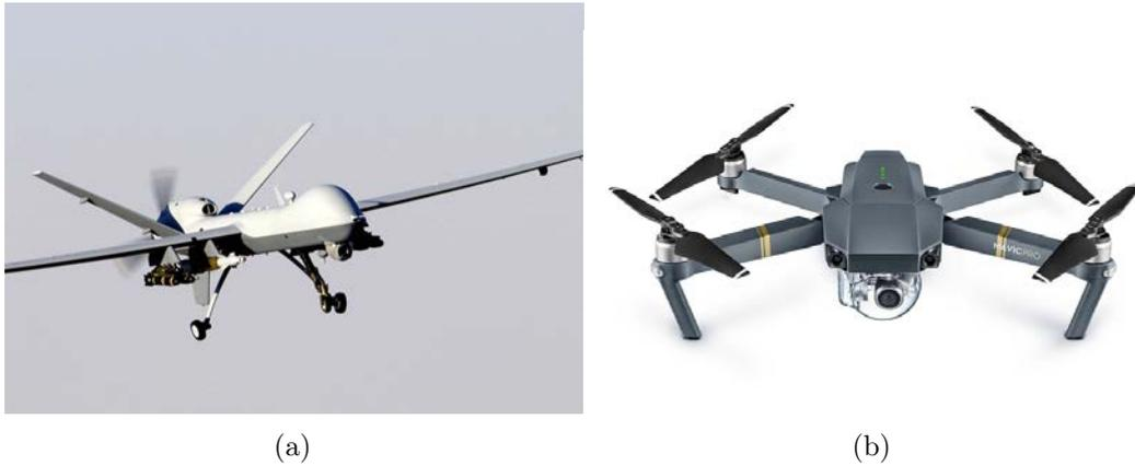
Figure 2.6 – Examples of fixed and rotary wing UAVs. Fig. 2.6(a): the MQ-9 Reaper, from General Atomics. Fig. 2.6(b): the Mavic Pro, from DJI.
