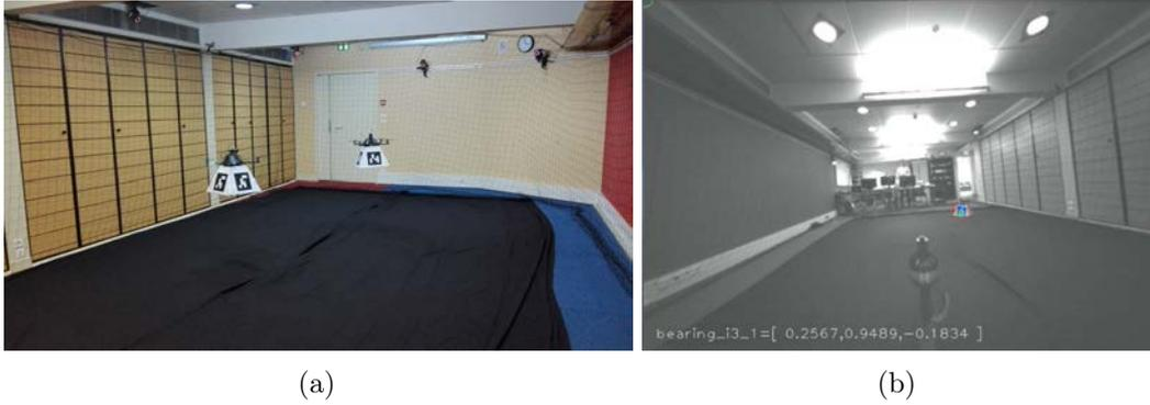
Figure 8.1 – First tests with the AprilTag fiducial markers. Fig. 8.1(a): two quadrotor UAVs flying in our flying arena with some Apriltag [197] mounted on them. Note that we plan to reduce the size of the fiducial markers used in our applications to make them more compact and easy to embed on each UAV. Fig. 8.1(b): a snapshot of an onboard camera which shows the detection of an AprilTag fiducial marker mounted on another quadrotor UAV and the consequent *translation* to a bearing vector.
