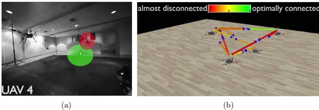
Figure 6.4 – Fig. 6.4(a) highlights why the *occluded visibility* constraint is needed. Indeed, it is possible to notice how the visibility of the robot in red, with respect to the *observing* robot, is being occluded by the robot in green. As usual, Fig. 6.4(b) is the graph view corresponding to the case of Fig. 6.4(a).
