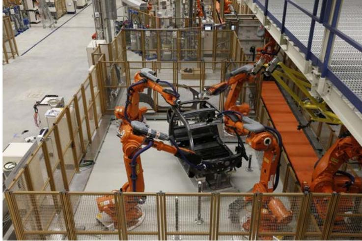
Figure 2.1 – An example of four robots working together, in an automotive factory, on the same car. The robots are fulfilling different tasks and they have a really limited awareness of other robots and of their environment (from which they are separated through a cage).
