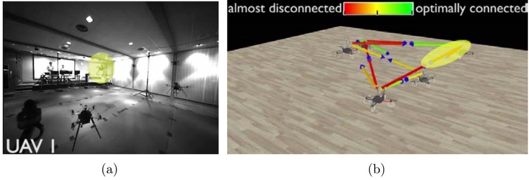
Figure 6.1 – Fig. 6.1(a) is a snapshot from the onboard camera mounted on a quadrotor. It is taken when the robot is close to lose a link (with respect to the robot highlighted in yellow) due to the *maximum range* constraint. Fig. 6.1(b) is the graph view corresponding to the case of Fig. 6.1(a).
